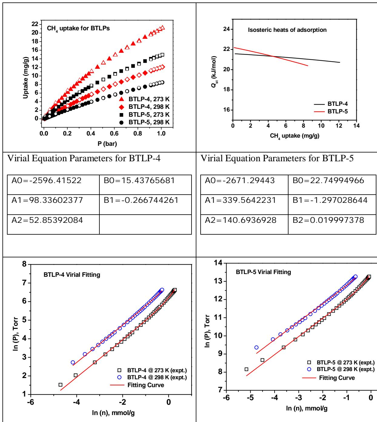
**Figure S12.** Low-pressure CH<sub>4</sub> gas uptakes and the isosteric heat of adsorptions for BOLPs.  $Q_{st}$  is calculated from Virial equation where isotherms collected at 273 and 298 K were fitted. Pressure is Torr and uptake is mmol/g.
