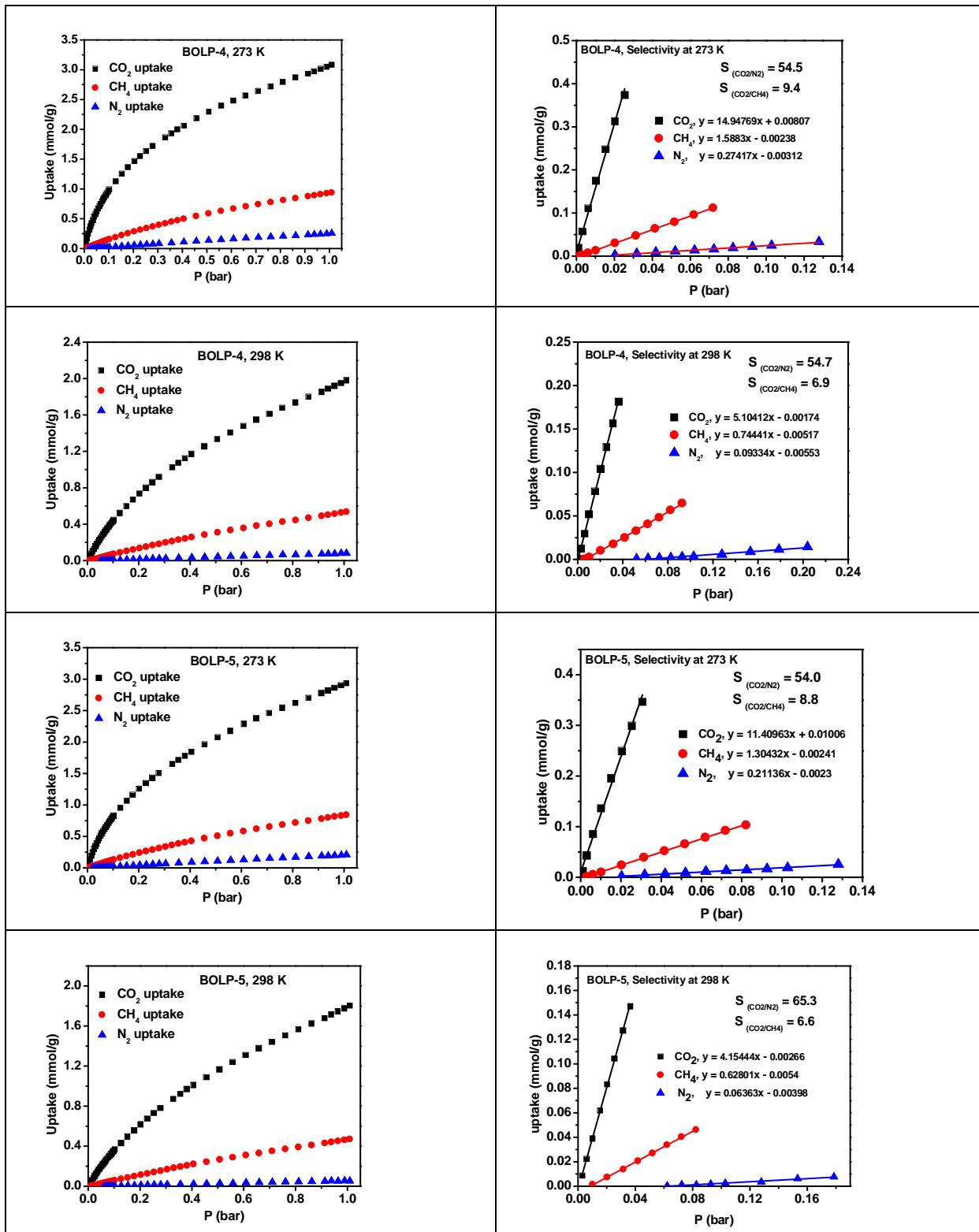
In order to calculate selectivities by IAST, the pure component isotherms of CO<sub>2</sub> were fitted with the dualsite Langmuir (DSL) isotherm model with a temperature dependent parameter. CH<sub>4</sub> and N<sub>2</sub> isotherms were fitted to single site Langmuir isotherms. Fitting parameters were used to calculate IAST selectivities. Details about the calculations were explained previously.
