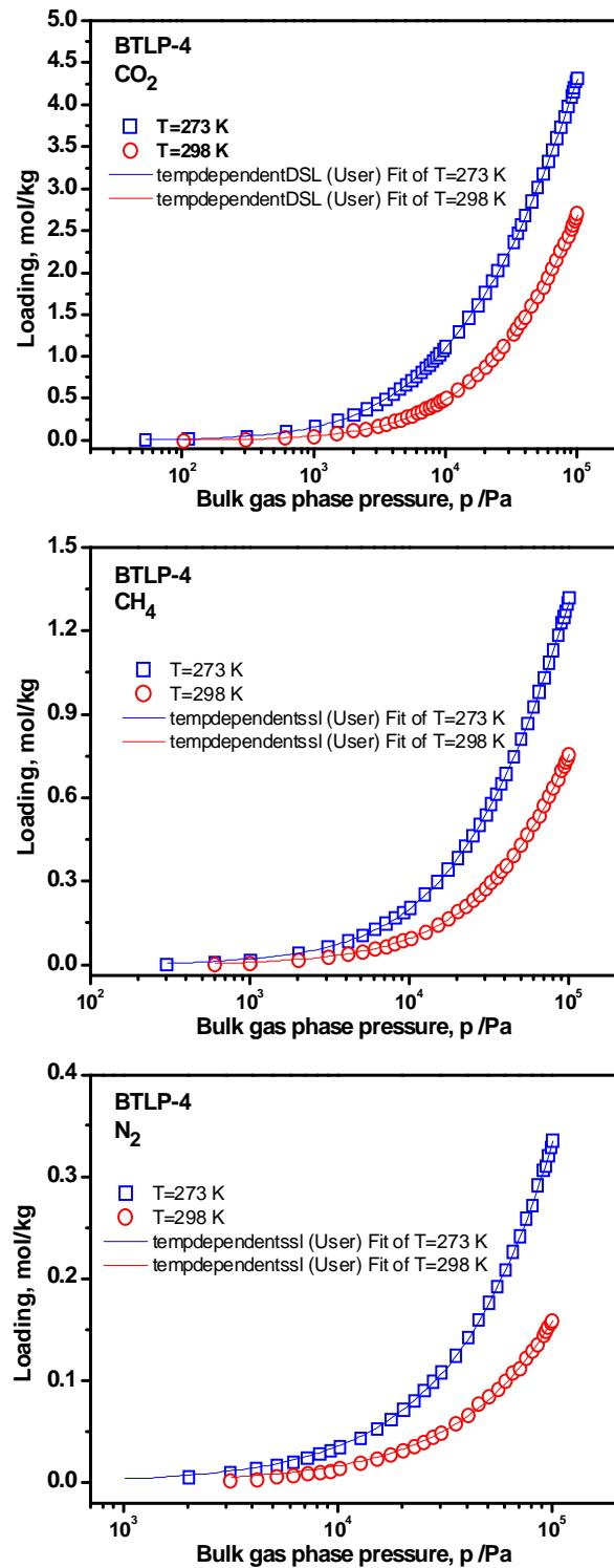
**Figure S18.** Dual site or single site Langmuir fitting plots for BTLP-5 at 273 (blue square) and 298 K (red circles) for CO<sub>2</sub> (top), CH<sub>4</sub> (middle) and N<sub>2</sub> (bottom).
