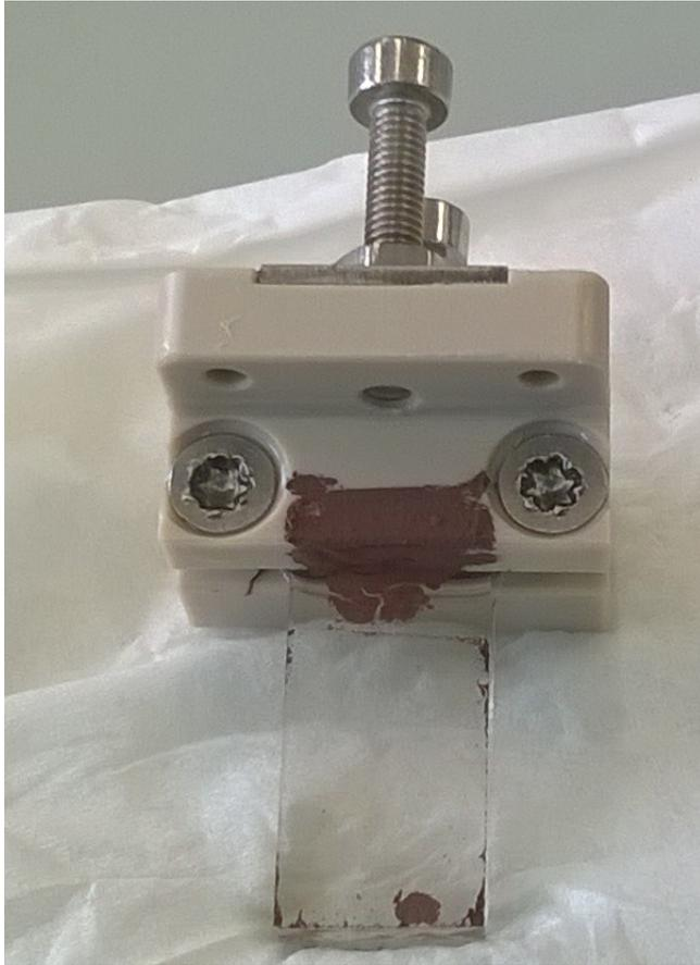
Figure SI 6. Picture of destroyed electrode after measurement. This electrode's active material contained 1 wt% GO and no additional TiO<sub>2</sub> necking was applied to improve stability. The film lifted off the FTO slide and floated on the water during measurement, indicating a hydrophobic particle surface due to significant GO coverage.
