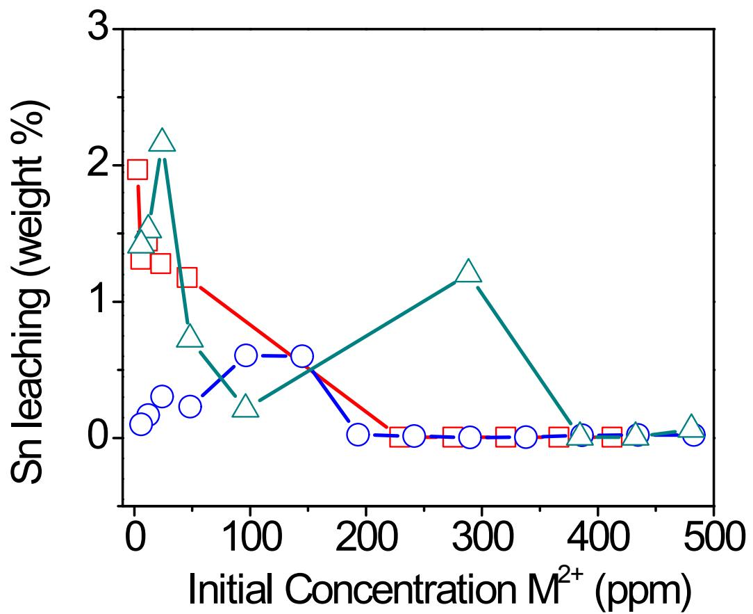
Figure S10. Plot shows the data for tin leaching (weight %) for the heavy metal ion exchange experiments of various concentrations (~5-500 ppm).
