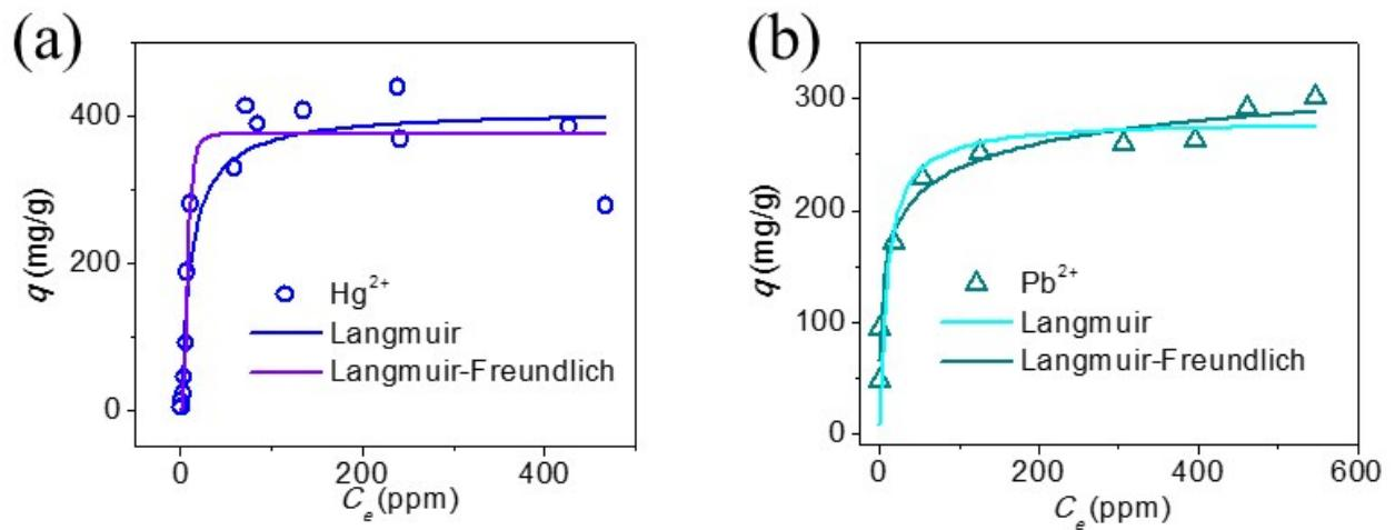
Figure S9. Equilibrium data for Hg<sup>2+</sup> and Pb<sup>2+</sup> ion-exchange, the solid data represents the fitted lines by Langmuir and Langmuir-Freundlich isotherm model.
