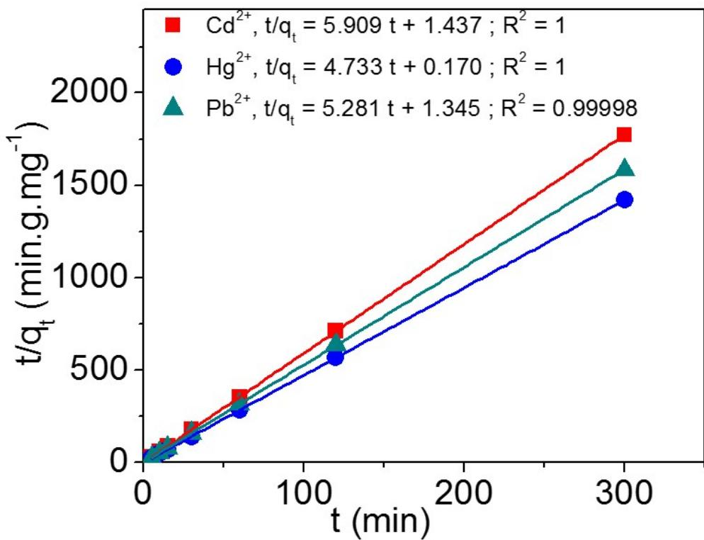
Figure S11. The plot of  $t/q_t$  vs  $t$  for the kinetics data of heavy metal ion absorption by KTS-3, which is fitted satisfactorily with the pseudo-second order kinetic model.
