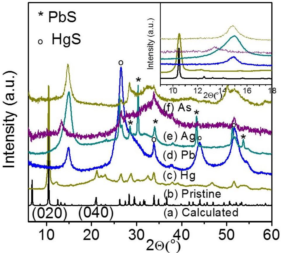
Figure S6. Powder X-ray diffraction patterns of pristine KTS-3 and the heavy metal ion-exchanged materials. The (020) and (040) reflection peaks for the exchanged materials shift towards higher  $2\theta$  (lower d spacing) indicates contraction of the interlayer distance.
