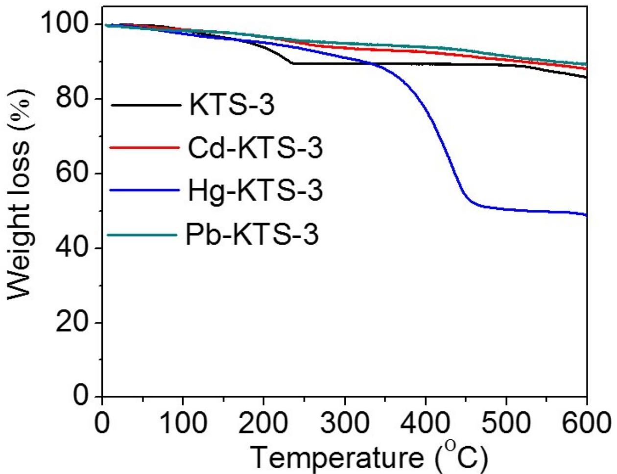
Figure S7. The TG analysis of the ion-exchanged materials.
