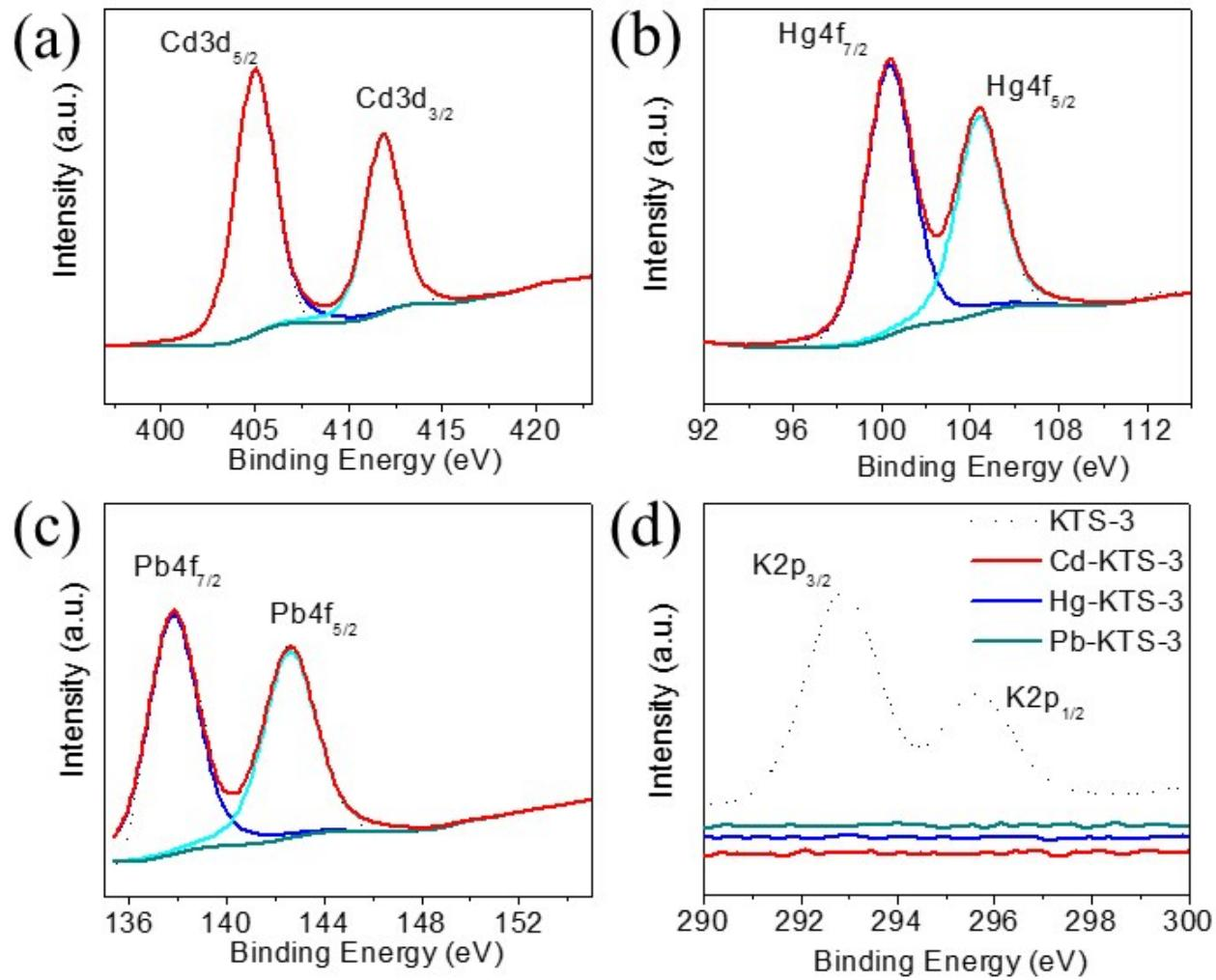
Figure S8. X-ray photoelectron spectra of (a) cadmium, (b) mercury, (c) lead and (d) potassium spectrum for the ion-exchanged materials. Dotted and solid lines represent experimental and deconvoluted spectra, respectively. Please note that no peak was observed for potassium for the heavy metal ion-exchanged materials, confirmation of complete potassium ion-exchange.
