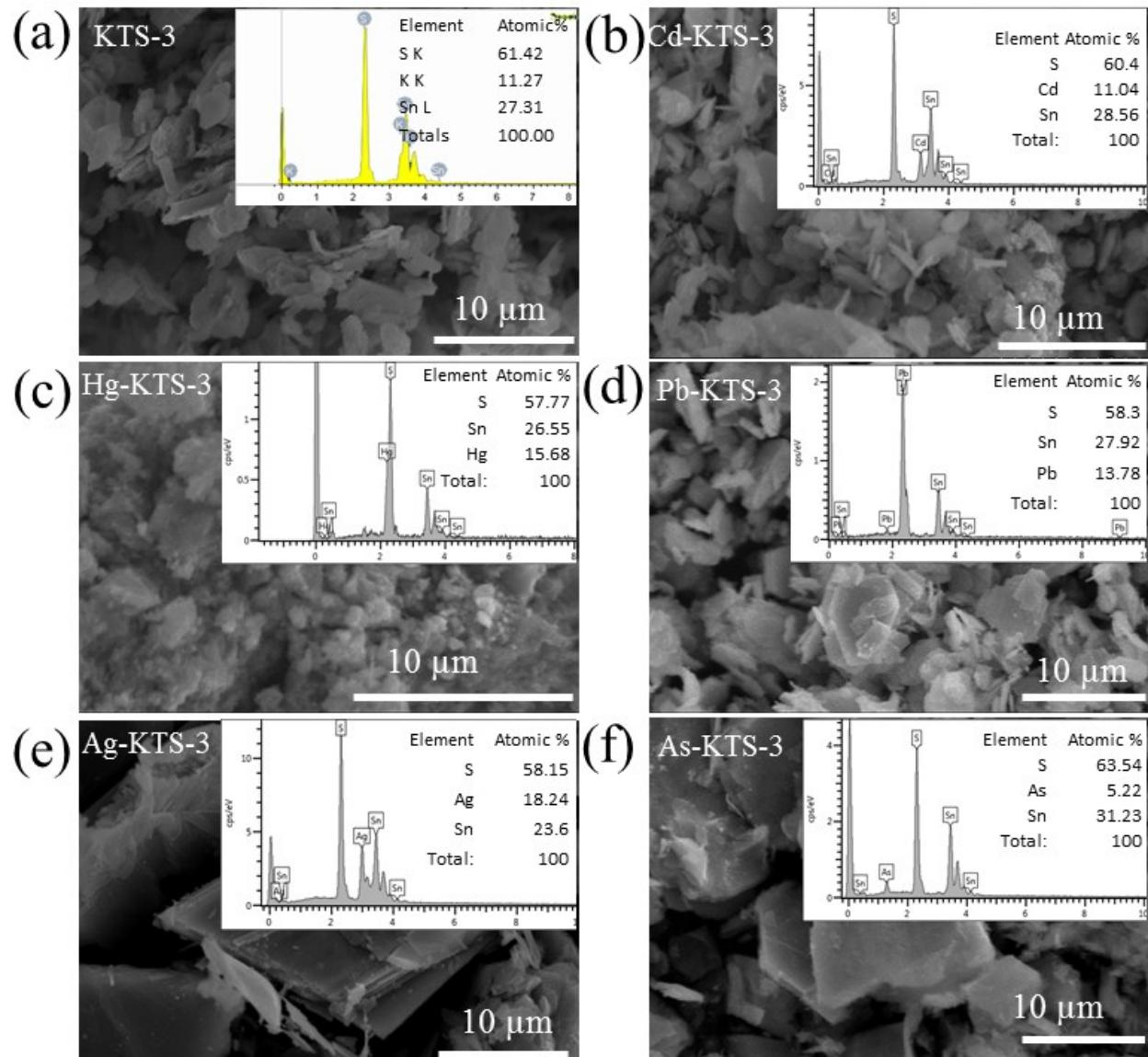
Figure S1. SEM micrograph and EDS data of (a) KTS-3 and the ion-exchanged samples (b) Cd-KTS-3, (c) Hg-KTS-3, (d) Pb-KTS-3, (e) Ag-KTS-3, and (f) As-KTS-3, respectively.
