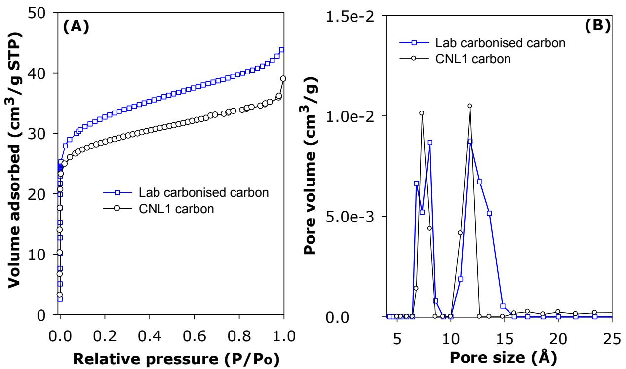
**Supporting Figure S16.** Nitrogen sorption isotherms (A) and pore size distribution curves (B) of CNL1 carbon and lab-based carbon from pyrolysis (carbonisation) of wood chippings under air containing atmosphere.
