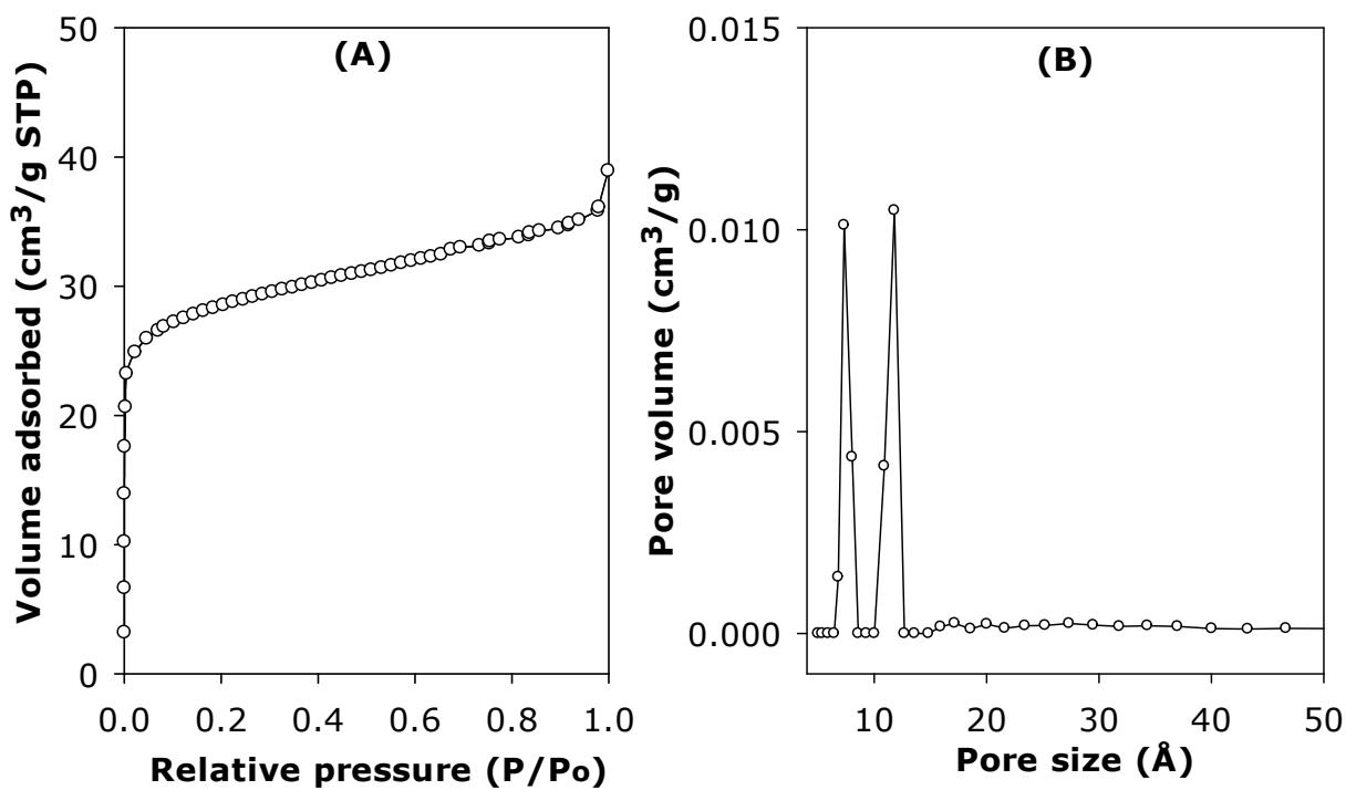
**Supporting Figure S5.** Nitrogen sorption isotherm (A) and pore size distribution curve (B) of CNL1 carbon.
