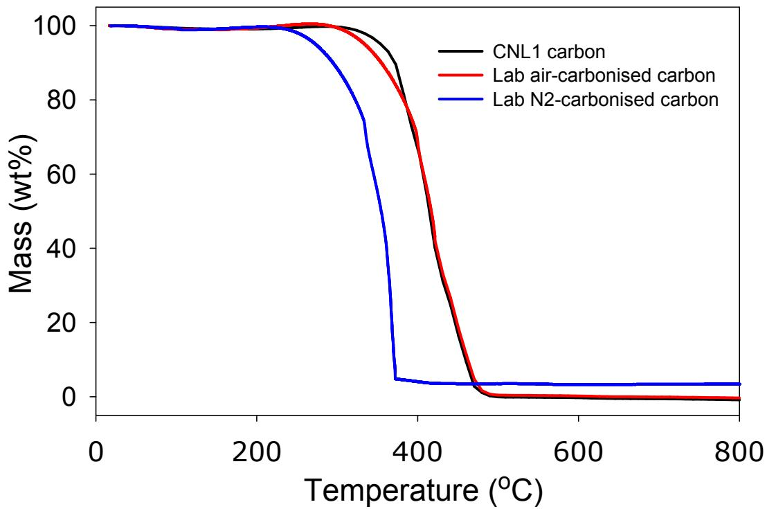
**Supporting Figure S14.** Thermogravimetric analysis (TGA) curve of CNL1 carbon, and lab-based carbon from pyrolysis (carbonisation) of wood chippings under air (lab air-carbonised carbon) or N<sub>2</sub> (lab N2-carbonised carbon).
