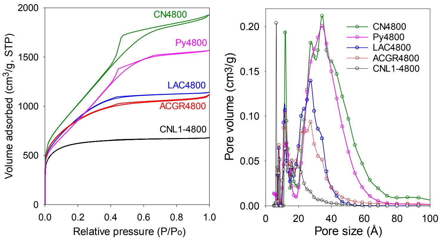
**Supporting Figure S10.** Nitrogen sorption isotherms and pore size distribution curves of activated CNL1-2800 carbon compared to analogous activated carbons derived from lignin (LAC4800), grass (ACGR4800), carbon nanotube superstructures (CN4800) or polypyrrole (Py4800) under similar activation conditions (i.e., 800 °C and KOH/carbon ratio of 4).
