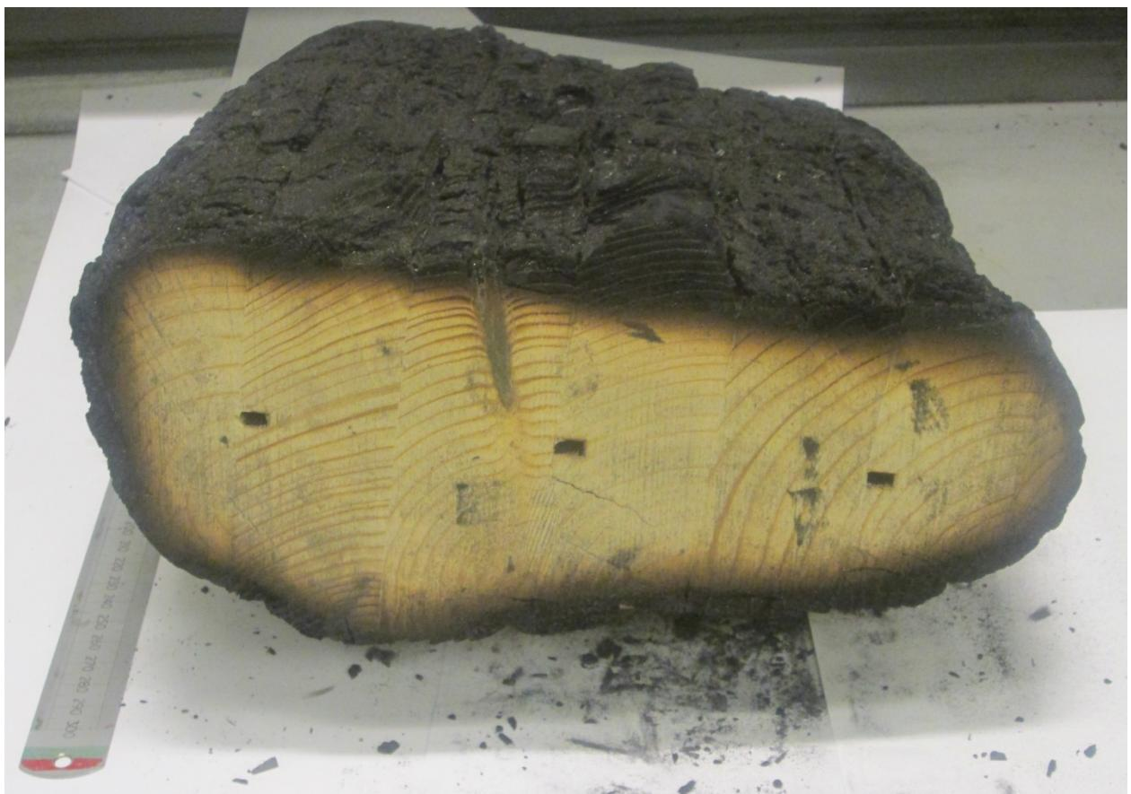
**Supporting Figure S2.** Cross section of charred wooden beam from Carbon Neutral Laboratory (CNL1).
