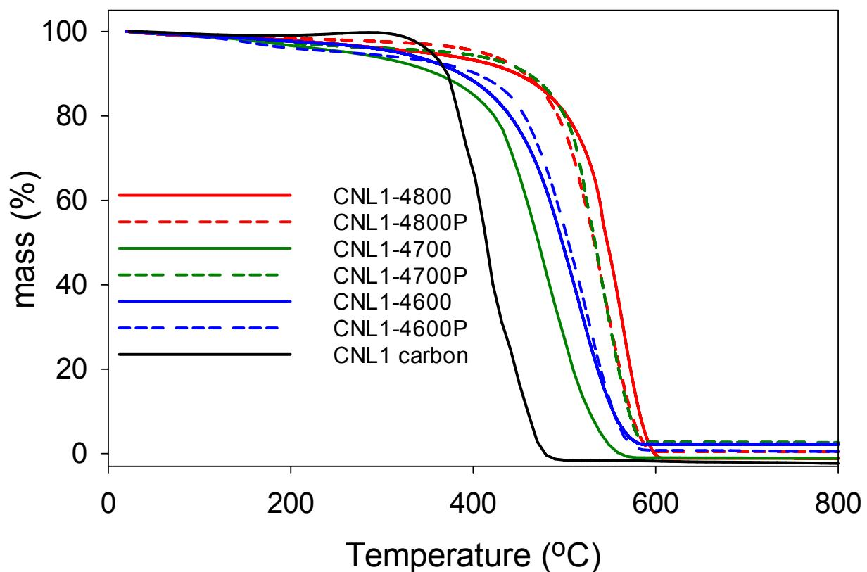
**Supporting Figure S7.** Thermogravimetric analysis (TGA) curve of CNL1 carbon and activated CNL1-4T carbons thermally treated in air.
