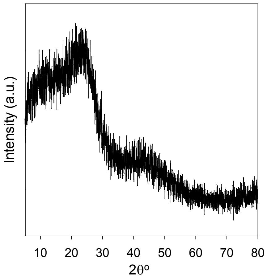
**Supporting Figure S3.** Powder XRD pattern of CNL1 carbon.
