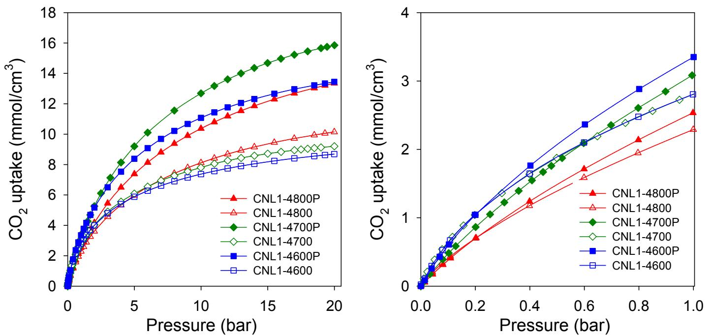
**Supporting Figure S20.** Volumetric CO<sub>2</sub> uptake isotherms at 25 °C and 0 – 20 bar (left panel) and 0 – 1 bar (right panel) for activated CNL1-4T carbons.
