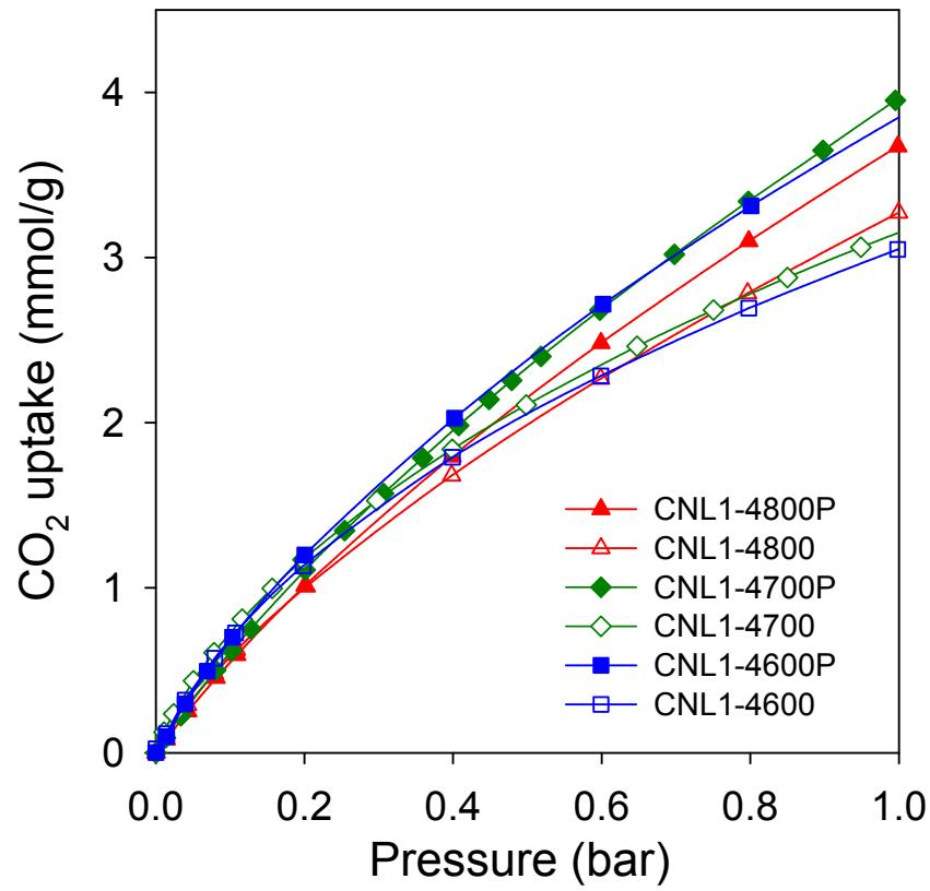
**Supporting Figure S18.** CO<sub>2</sub> uptake isotherms at 25 °C and 0 - 1 bar for activated CNL1-4T carbons.
