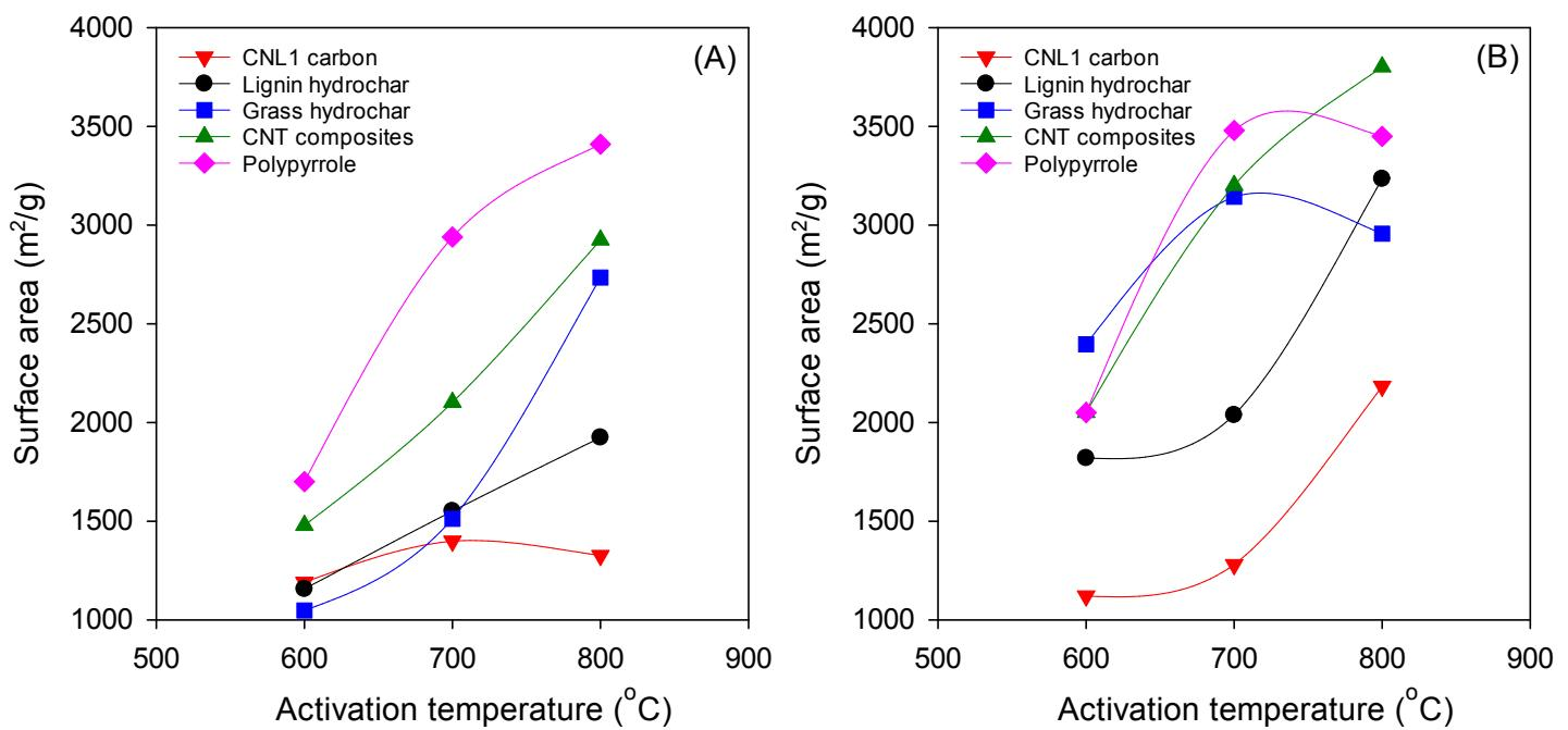
**Supporting Figure S11.** A plot of total surface area as a function of activation temperature for activated carbons derived from CNL1 carbon and other precursors at KOH/carbon ratio of; (A) 2 and (B) 4.
