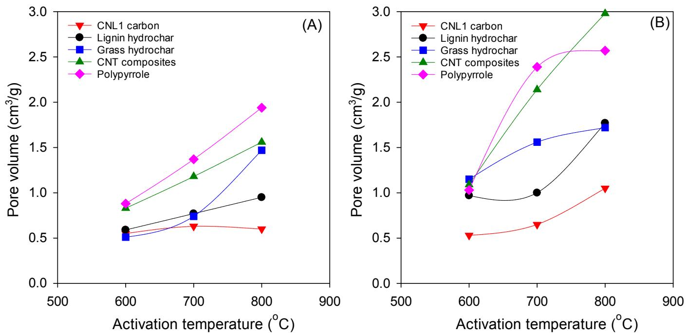
**Supporting Figure S12.** A plot of total pore volume as a function of activation temperature for activated carbons derived from CNL1 carbon and other precursors at KOH/carbon ratio of; (A) 2 and (B) 4.
