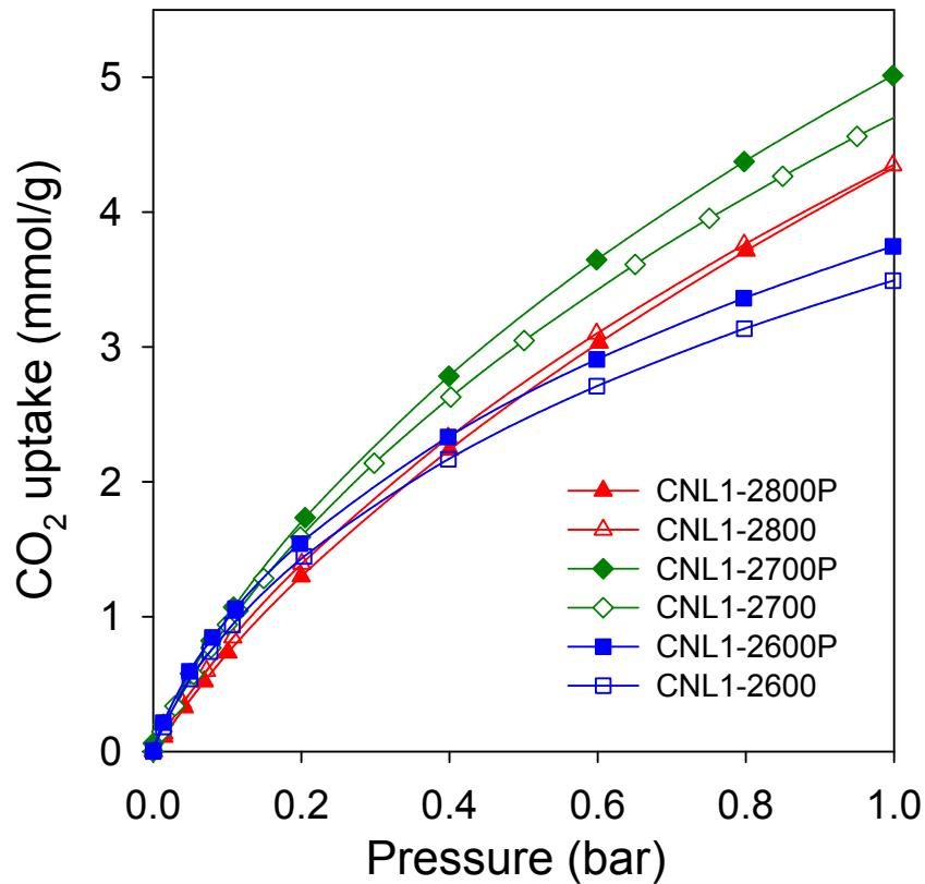
**Supporting Figure S17.** CO<sub>2</sub> uptake isotherms at 25 °C and 0 - 1 bar for activated CNL1-2T carbons.
