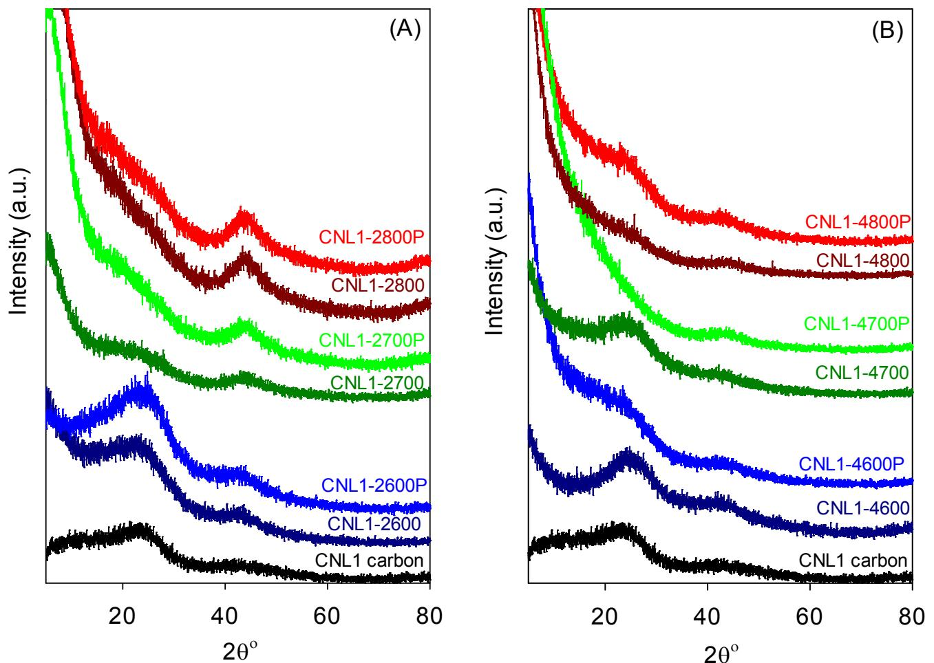
**Supporting Figure S8.** Powder XRD pattern of CNL1 carbon, and activated CNL1-2T (A) and CNL1-4T (B) carbons.
