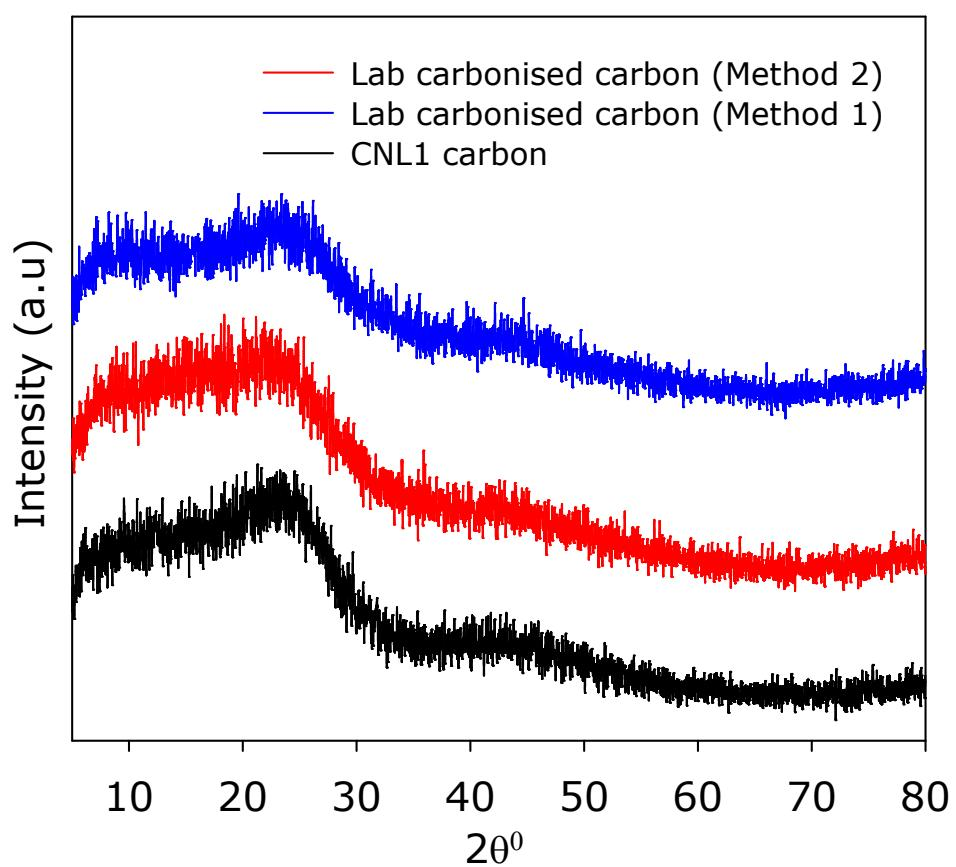
**Supporting Figure S15.** Powder XRD patterns of CNL1 carbon, and lab-based carbon from pyrolysis (carbonisation) of wood chippings under air containing atmosphere. See above for description of method 1 and 2.
