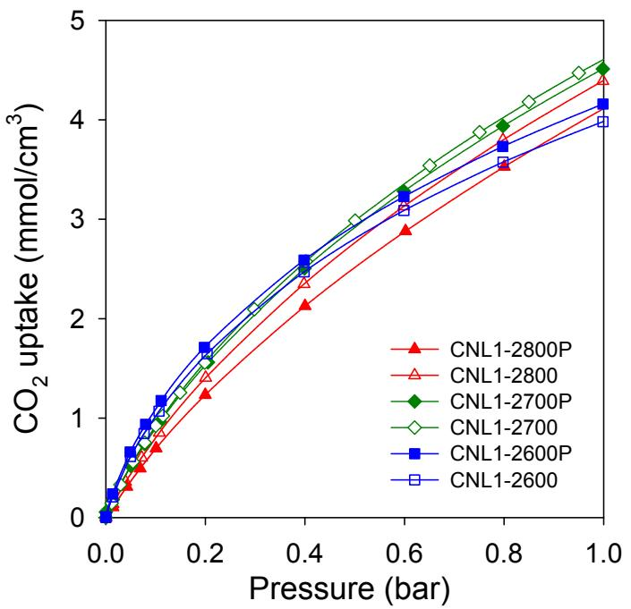
**Supporting Figure S19.** Volumetric  $\text{CO}_2$  uptake isotherms at 25 °C and 0 – 20 bar (left panel) and 0 – 1 bar (right panel) for activated CNL1-2T carbons.
