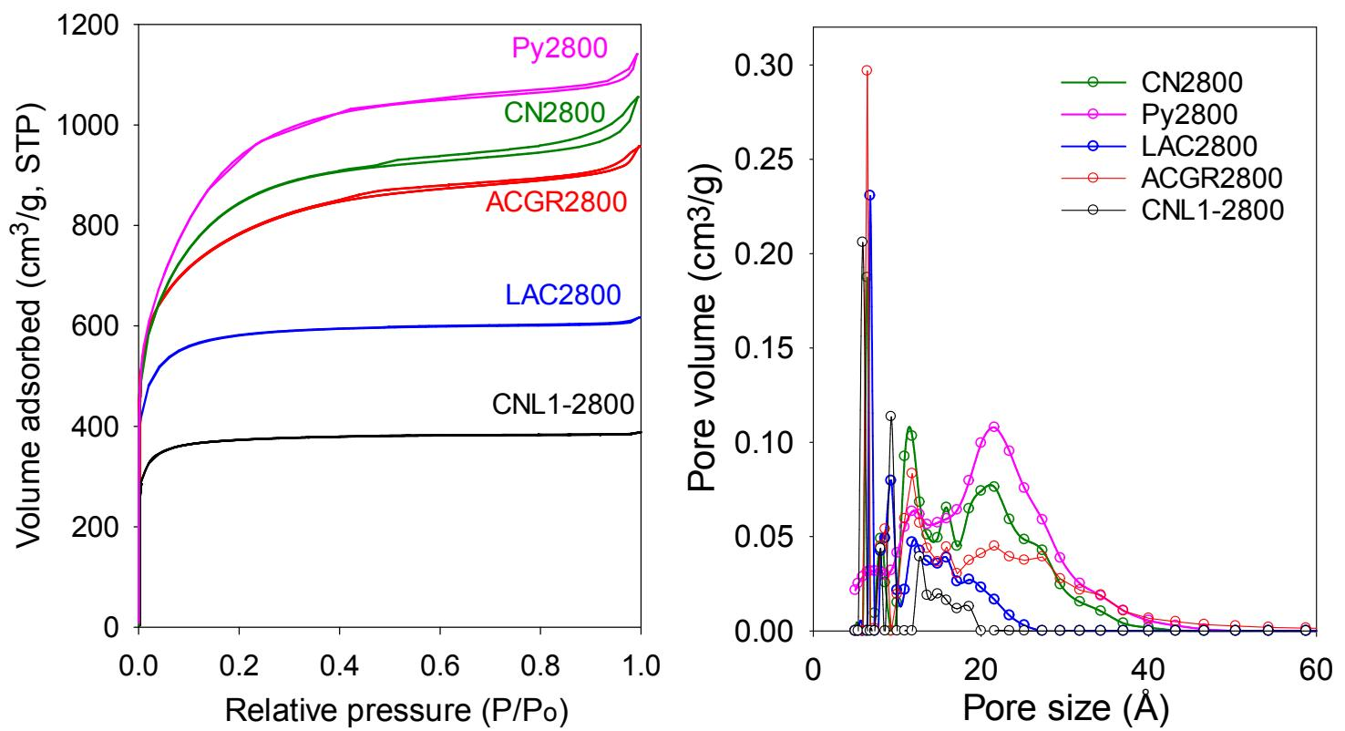
**Supporting Figure S9.** Nitrogen sorption isotherms and pore size distribution curves of activated CNL1-2800 carbon compared to analogous activated carbons derived from lignin (LAC2800), grass (ACGR2800), carbon nanotube superstructures (CN2800) or polypyrrole (Py2800) under similar activation conditions (i.e., 800 °C and KOH/carbon ratio of 2).
