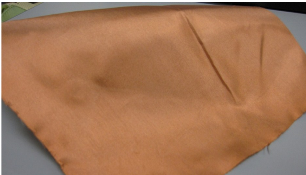
Fig. S1 Photograph of a large piece of copper-plated Dacron cloth.
