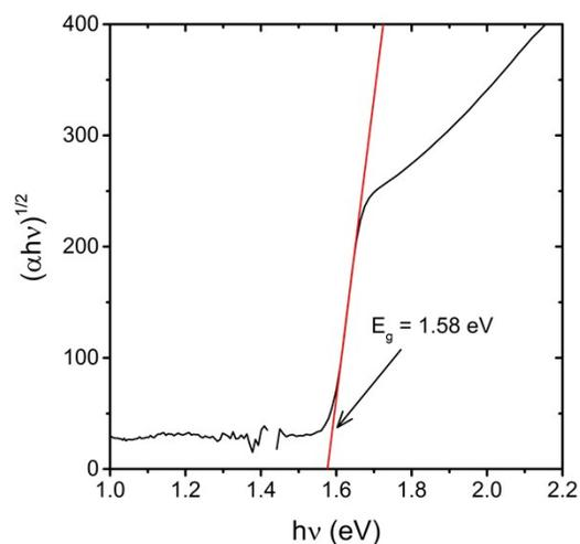
**Figure S6.** Tauc plot for optical band-gap determination the perovskite film prepared at 50°C. Values are calculated from the absorption coefficient in Figure S5.
