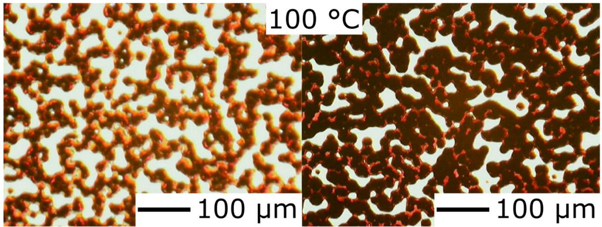
**Figure S11.** Optical microscope images (x255 magnification) of the intermediate films obtained with different substrate temperatures (left) and of the resulting perovskite films after annealing at 100 °C (right).
