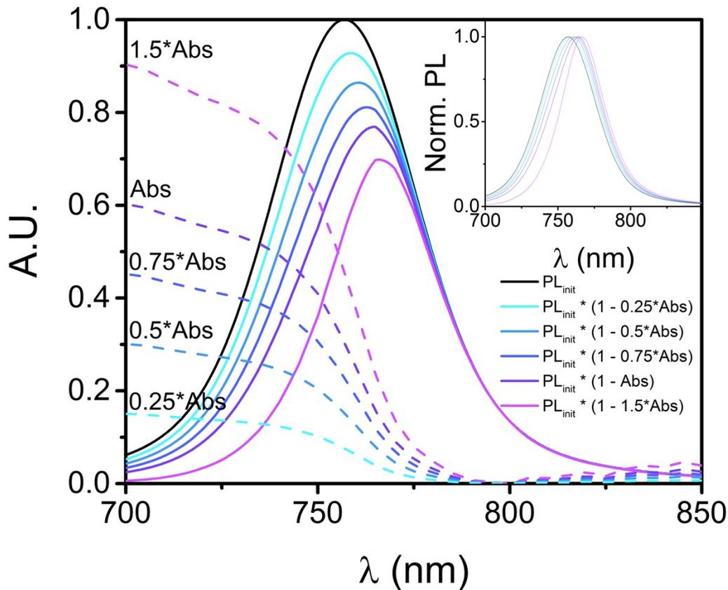
**Figure S9.** Modeling of the inner-filter effect. A normalized emission spectrum,  $PL_{init}$ , is subjected to different amounts of filtering from the absorbance spectrum,  $Abs$ , of the perovskite. This filtering serves to shift the emission peak towards longer wavelengths.
