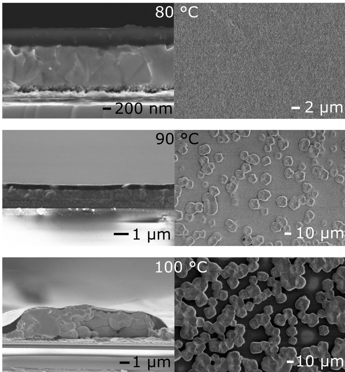
**Figure S10.** Scanning electron microscope images of perovskite solar cell cross-sections (left) and of the surface morphology for perovskite films (right) prepared with different substrate temperatures.
