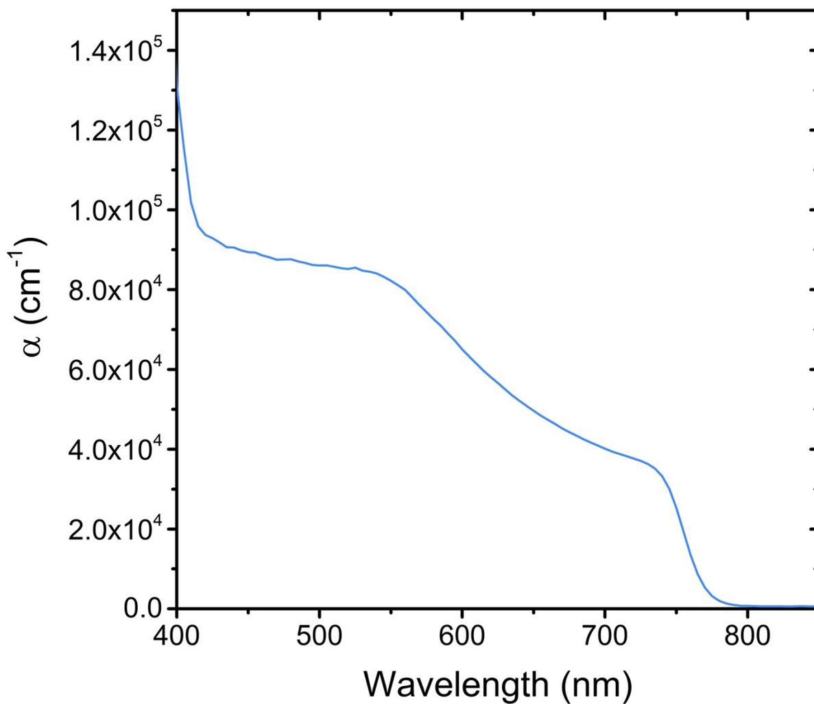
**Figure S5.** Absorption coefficient ( $\alpha$ ) of the  $(\text{FAPbI}_3)_{0.85}(\text{MAPbBr}_3)_{0.15}$  perovskite film prepared with substrate temperatures of 50 °C. Values are calculated from the equations described above using the data from Figure S4.
