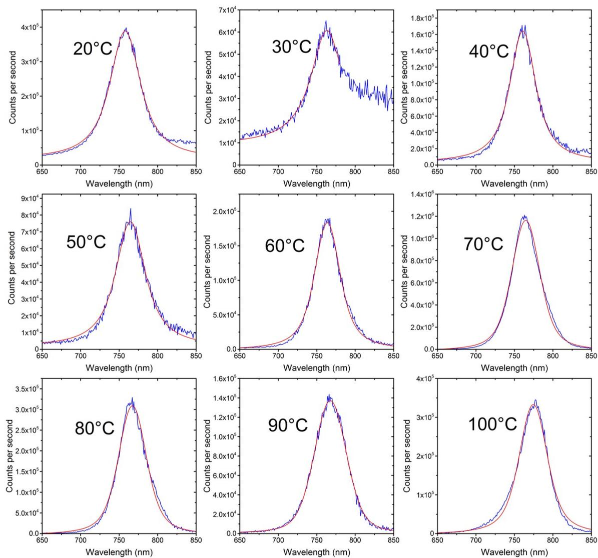
**Figure S7.** Raw-data (blue) from steady-state photoluminescence measurements of the perovskite films prepared with different substrate temperatures. The data was fitted using a Voigt profile probability density function (red) in Origin 2015. An excitation wavelength of 500 nm was used.
