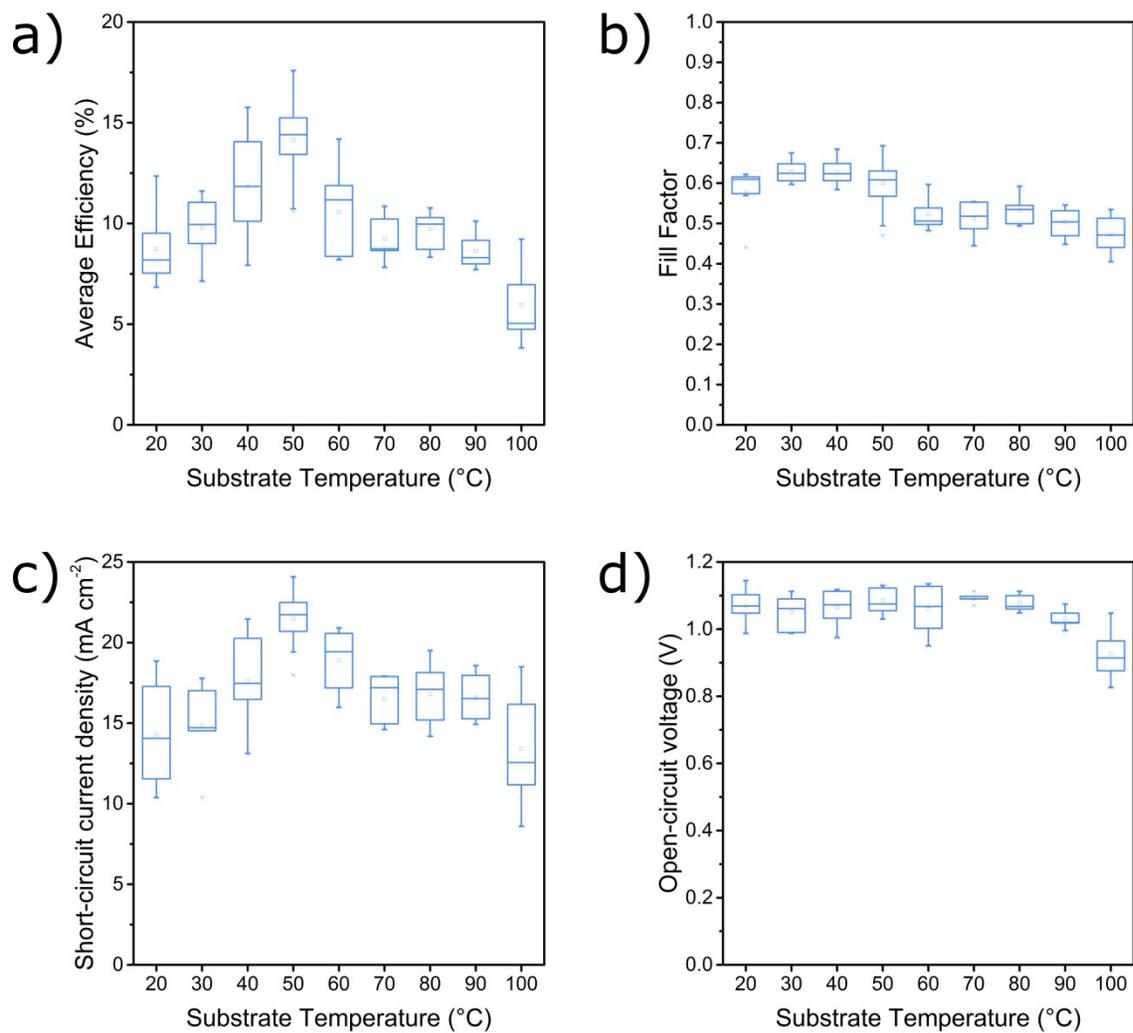
**Figure S12.** Boxplot statistics of; a) photovoltaic performances, b) fill factors, c) short-circuit current densities and d) open circuit voltages of solar cells prepared with different substrate temperatures. The parameters are derived from the average of the backward (open-circuit to short-circuit) and forward (short-circuit to open-circuit)  $I$ - $V$  scans. The scan rate was 10 mV/s.
