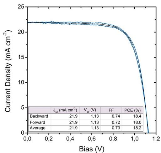
**Figure S13.** Current-voltage ( $I$ - $V$ ) scan of a standard mixed-ion perovskite device prepared in a dry nitrogen glovebox under 1 sun illumination intensity. Both backward and forward scans are depicted (blue) along with the average of the two (dashed). Parameters presented in the inset table are: short circuit current density ( $J_{sc}$ ), open circuit voltage ( $V_{oc}$ ), fill factor ( $FF$ ), and power conversion efficiency (PCE). The scan rate was 10 mV/s.
