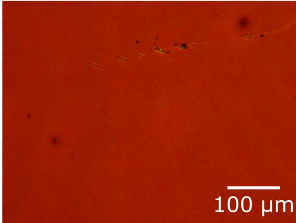
**Figure S2.** Optical microscope image (x255) of a methylammonium lead(II) triiodide (MAPbI<sub>3</sub>) intermediate film prior to annealing.
