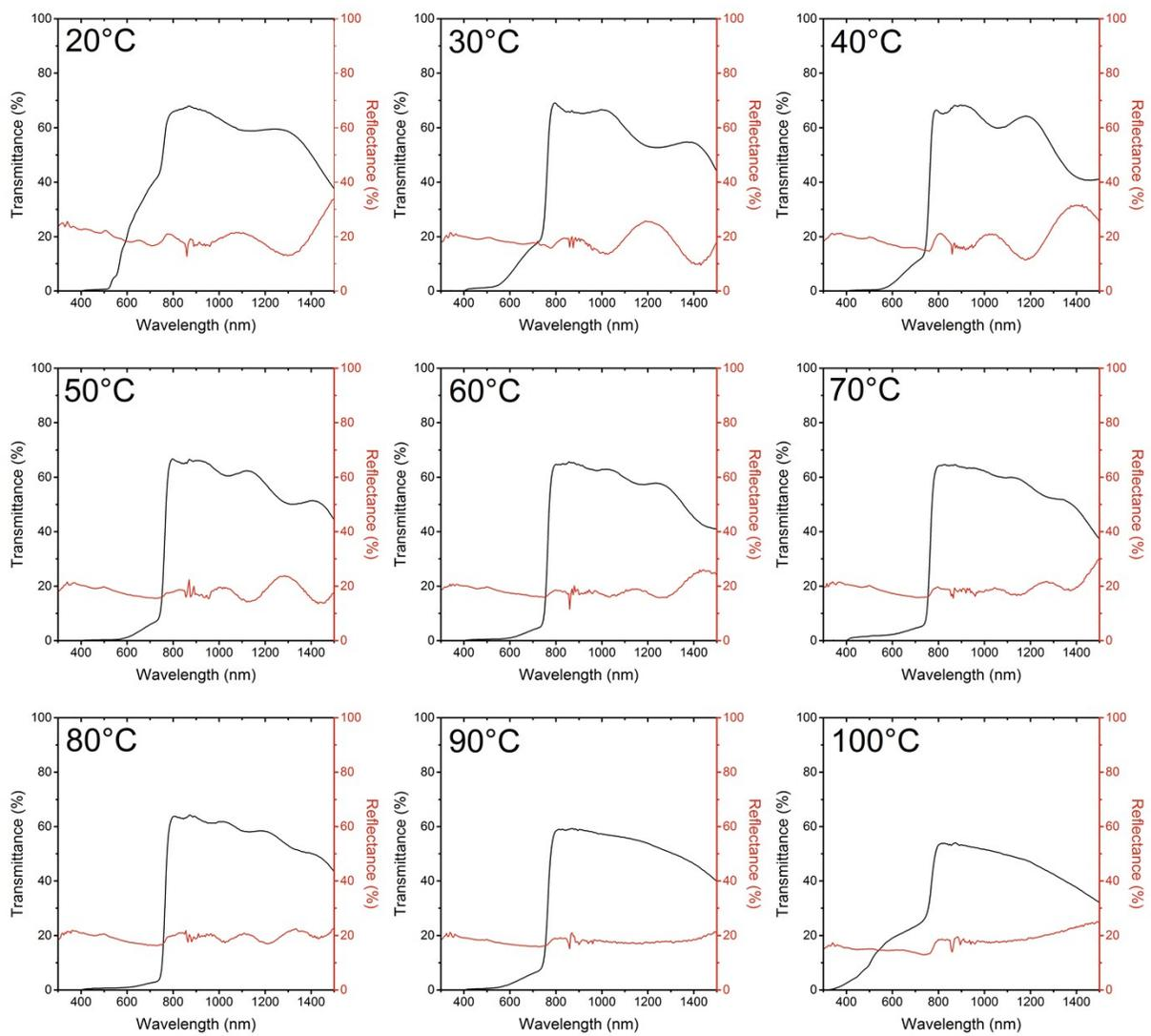
**Figure S4.** UV-Vis-NIR transmittance (black) and reflectance (red) spectra of the perovskite films prepared with different substrate temperatures.
