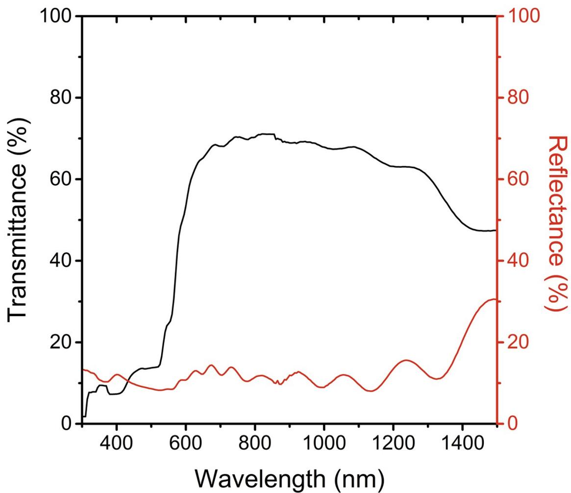
**Figure S3.** UV-Vis-NIR transmittance (black) and reflectance (red) spectra of the red intermediate phase. The interference fringes observed in the reflectance spectrum indicate a uniform thickness of the film.
