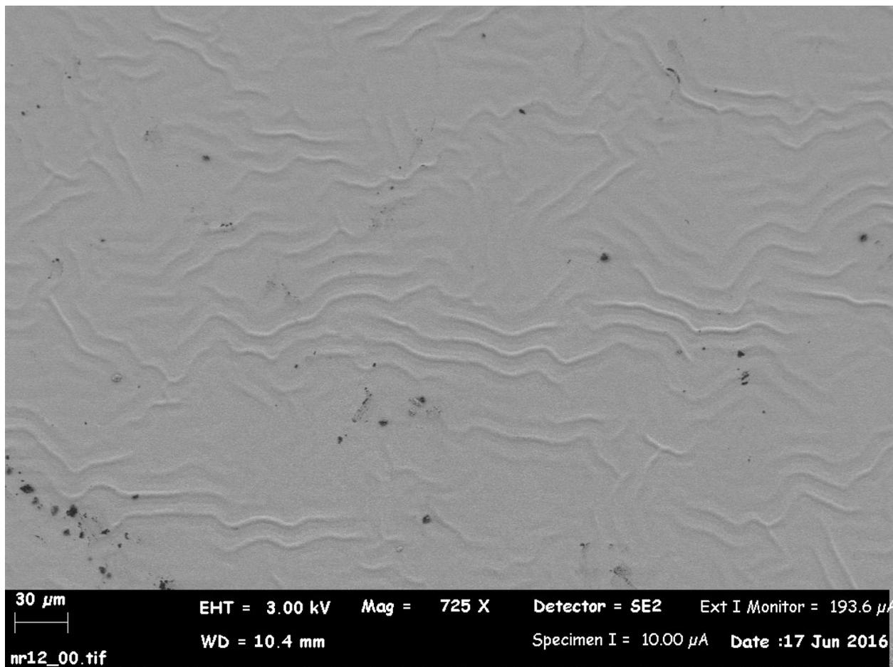
**Figure S14.** Scanning electron microscope image of the surface morphology for a mixed-ion perovskite film prepared at 50 °C. Similar wrinkle features are observed as for the optical microscope with approximately the same wavelength distance ( $\sim 15 \mu\text{m}$ ) between each wrinkle.
