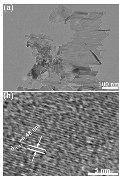
Fig. S4 (a) TEM image of LTO1, and (b) HRTEM image of LTO1.
