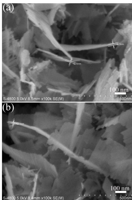
Fig. S2 SEM images of the as-prepared materials: (a) LTO1, and (b) LTO2.
