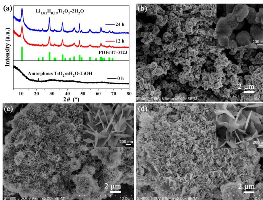
Fig. S1 The precursors of LTO2 obtained from hydrothermal treatment at different time: (a) XRD patterns, (b) SEM images for 0 h, (c) 12 h, and (d) 24 h, respectively.
