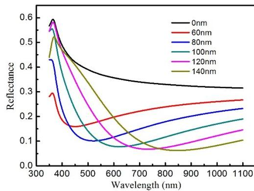
**Figure S3.** Finite Difference Time Domain (FDTD) based simulations of reflectance spectra of planar Si with different thickness of PMMA antireflection coating. 100 nm PMMA offers the best effect for reducing the optical loss of the device.
