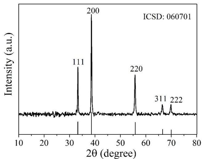
**Figure S6.** The XRD pattern of the pristine  $\text{Ca}_{0.5}\text{Mn}_{0.5}\text{O}$
