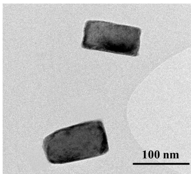
**Figure S7.** The TEM image of the pristine  $\text{Ca}_{0.5}\text{Mn}_{0.5}\text{O}$
