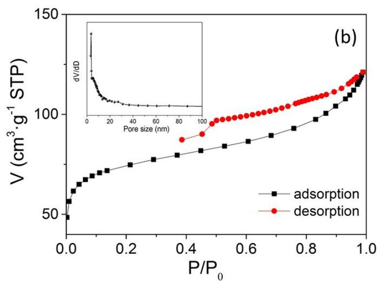
**Figure S3.** N<sub>2</sub> adsorption-desorption isotherms of MnO/C.
