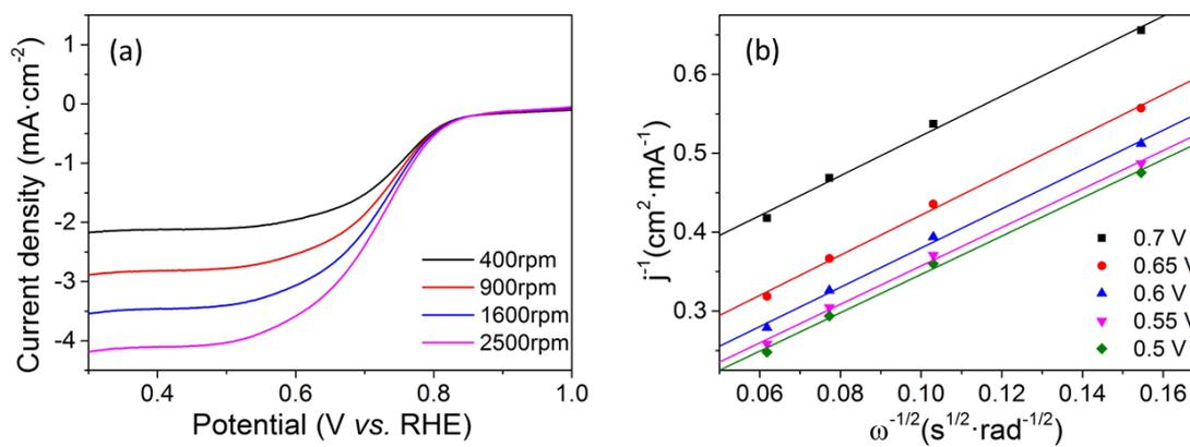
**Figure S5.** (a) LSV curves of MnO/C at the rotation speed from 400 rpm to 1600 rpm, and (b) the corresponding Koutechy-Levich plots.
