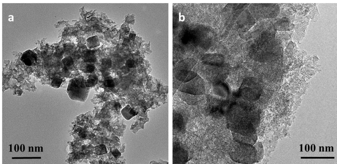
**Figure S1.** TEM image of (a) MnO/C and (b) Ca<sub>0.5</sub>Mn<sub>0.5</sub>O/C
