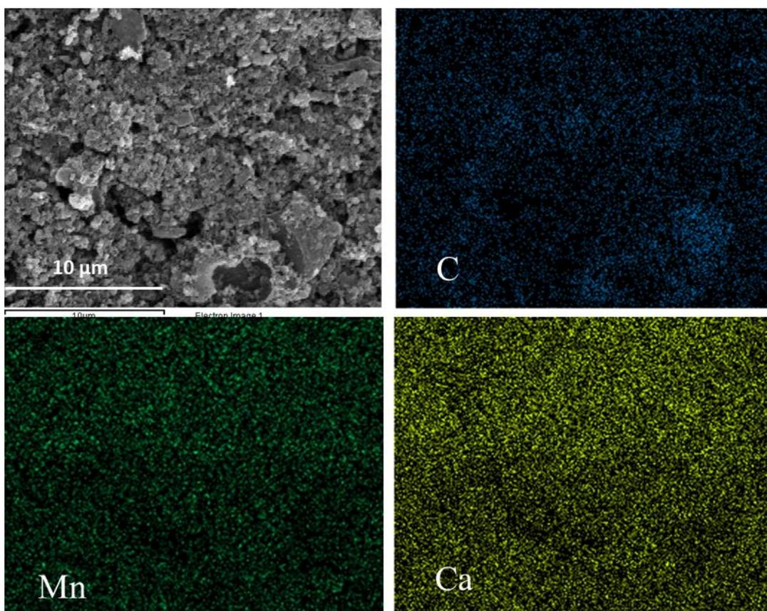
**Figure S2.** SEM image and EDS mapping of Ca<sub>0.5</sub>Mn<sub>0.5</sub>O/C. From the EDS mapping, one can see that C, Mn, and Ca are evenly distributed, which suggests that the Ca-substitution is uniform over the whole material.
