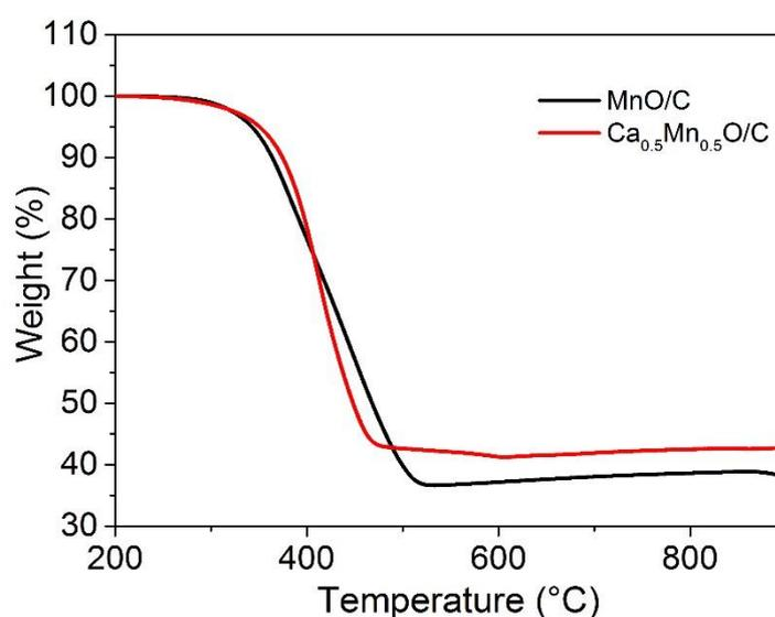
**Figure S4.** TGA curve obtained for  $\text{Ca}_{0.5}\text{Mn}_{0.5}\text{O}/\text{C}$  and  $\text{MnO}/\text{C}$  in air.
