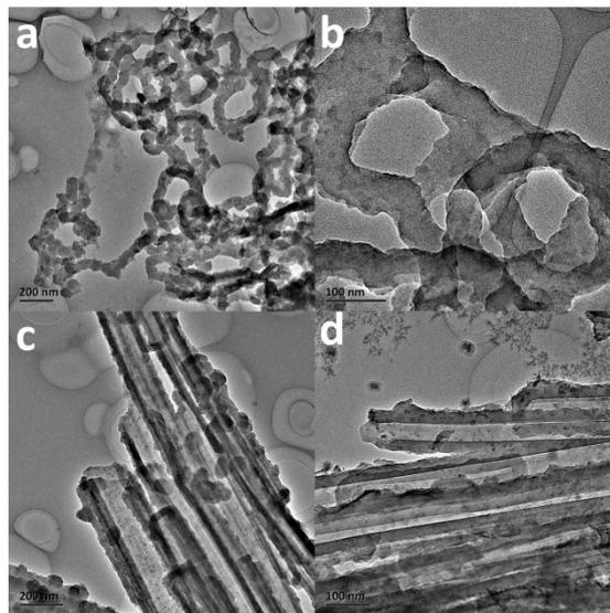
Fig. S3. TEM images of PPy nanowire and PPy nanotube. As shown, the TEM images of PPy nanowire and PPy nanotube are showed here. As shown in Fig. S3, the the diameters of PPy nanotubes and PPy nanowire are 120 nm and 50 nm, respectively. And a hollow structure is observed clearly in Fig.S3c and Fig. S3d, which is beneficial to inhibit the migration of lithium polysulfides in the electrolyte.
