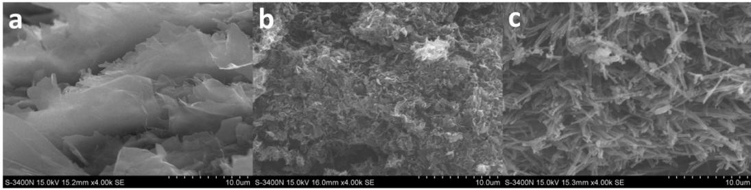
Fig. S2. Cross section morphology of different coating layer, (a) rGO, (b) PPy nanowire, (c) PPy nanotube. As shown, there are more pores for PPy nanotube coating layer compared to those of PPy nanowire. This is beneficial to absorb more lithium polysulfides in the electrolyte.
