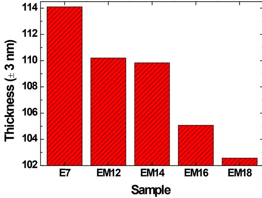
Fig. S6 Comparison of the film thickness of EG added and mixed co-solvent added PEDOT:PSS films on n-type Si substrates, as estimated by UV-reflectometry method.
