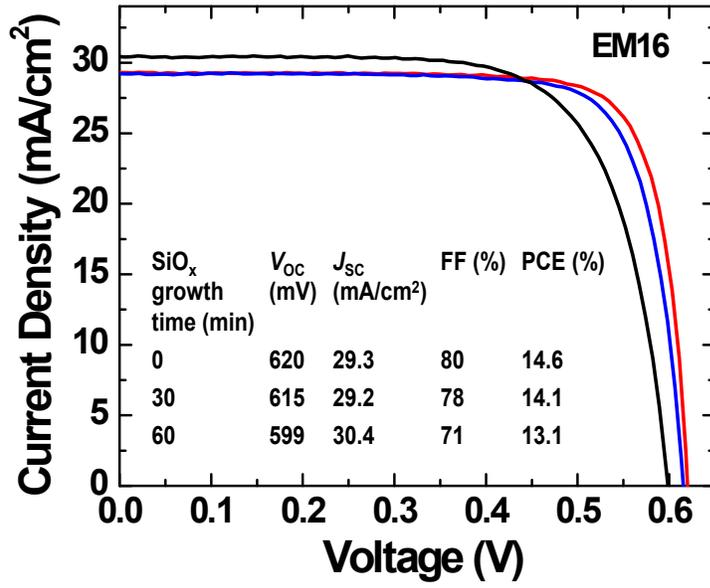
Fig. S2 Effects of the SiO<sub>x</sub> growth time on the solar cell properties of the EM16 sample.
