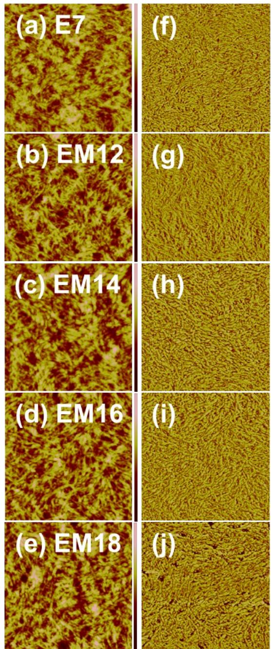
Fig. S4 AFM topography images of (a) E7, (b) EM12, (c) EM14, (d) EM16, and (e) EM18 samples and their corresponding phase images in (f-j). The image area is  $1 \times 1 \mu\text{m}^2$  and the vertical scale bar is from 0 to 20 nm.
