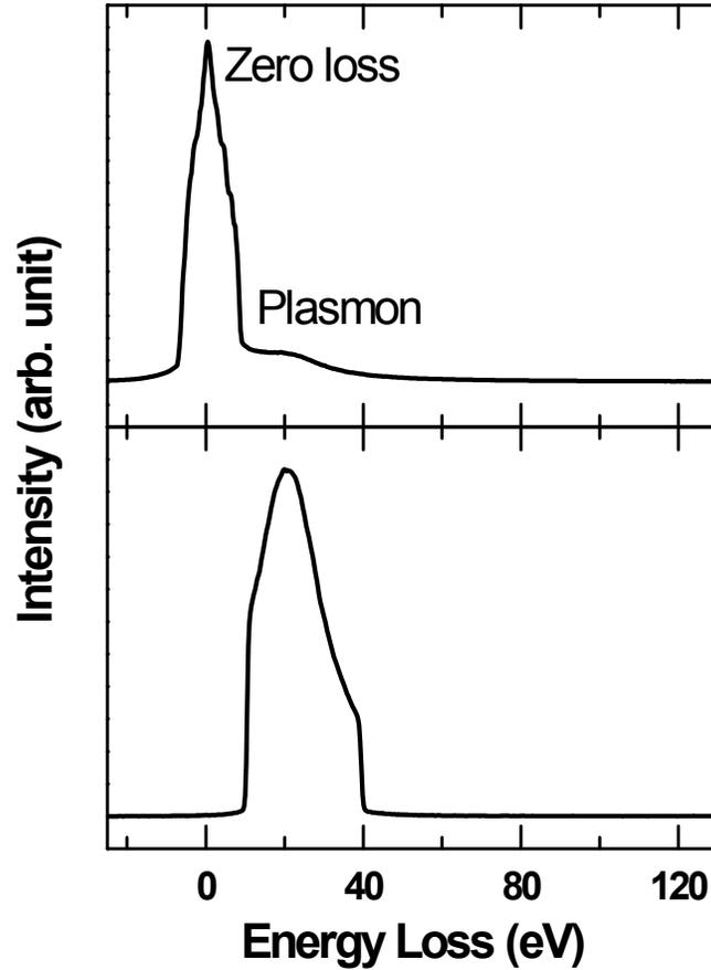
Fig. S5 Typical electron energy loss (EELS) spectra of the EM16 sample before (upper) and after (lower) applying an energy filter. The zero loss and plasmon peaks are labelled in the spectrum before applying the filter. Similar EELS spectra were also observed for other samples. An adjustable slit was used as a filter to selectively limit the energy range to 10-40 eV, which was used to form the low-loss energy-filtered TEM (EFTEM) images.
