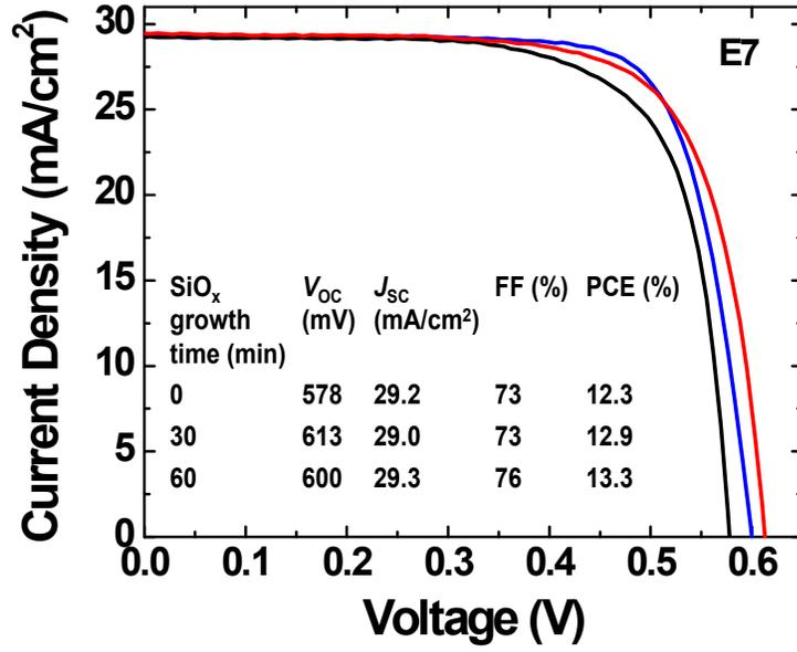
Fig. S1 Effects of the SiO<sub>x</sub> growth time on the solar cell properties of the E7 sample.
