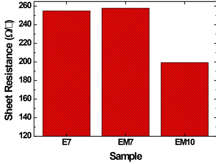
Fig. S3 Comparison of sheet resistance of the E7, EM7, and EM10 samples.
