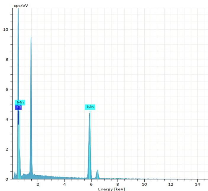
**Figure S4.** EDX spectra of the highly active mixed-valent MnO<sub>x</sub> spheres.
