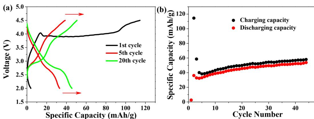
**Figure S5.** (a) The discharge-charge curves at a current density of 100 mA/g<sub>carbon</sub> of Li-ion batteries with mixed-valent MnO<sub>x</sub> spheres cathode at 2.0-4.5 V. (b) Cycling performance of the mixed-valent MnO<sub>x</sub> spheres cathode.
