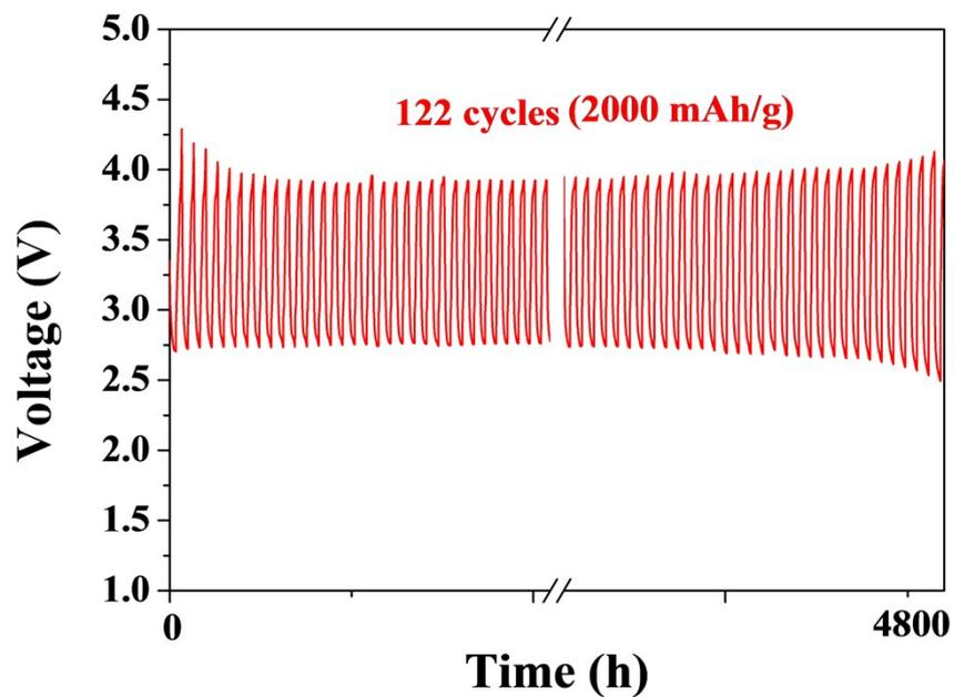
**Figure S6.** Cycling performance of Li-O<sub>2</sub> batteries with mixed-valent MnO<sub>x</sub> spheres under 200 mA/g<sub>carbon</sub> at a limited capacity of 2000 mAh/g<sub>carbon</sub>.
