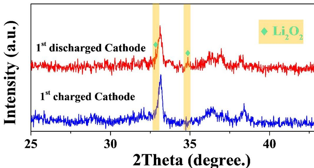
**Figure S9.** XRD pattern of mixed-valent  $\text{MnO}_x$  spheres electrode after first discharge and charge.
