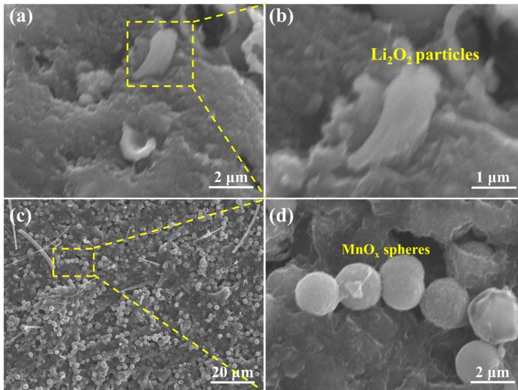
**Figure S8.** (a) SEM image of the  $\text{MnO}_x$  electrodes after discharging to 2.5 V. (b) Corresponding enlarged SEM image of the yellow area in (a). SEM (c) and corresponding enlarged images (d) of the  $\text{MnO}_x$  electrodes after one deep discharge-charge cycle.
