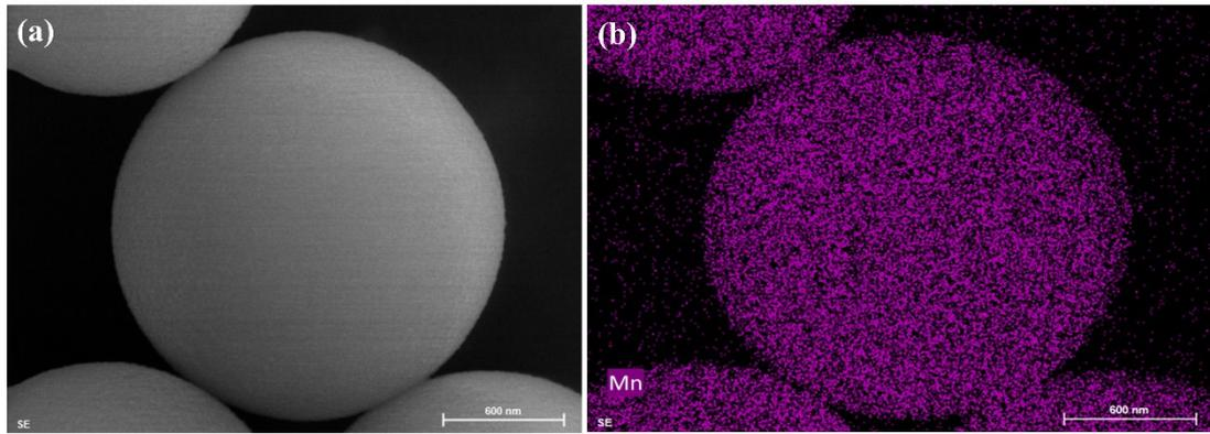
**Figure S3.** The dark-field scanning SEM image and corresponding elemental mapping image of the mixed-valent  $\text{MnO}_x$  spheres.
