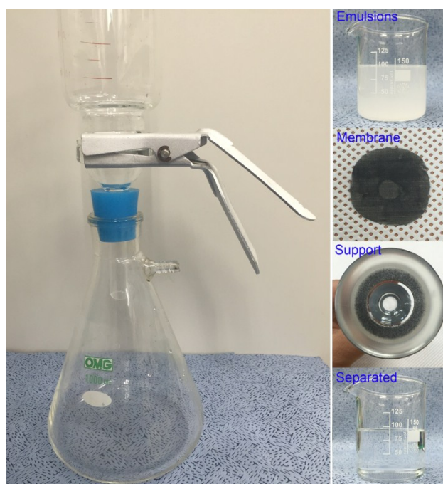
Fig. S5. The photographs of device for water-in-toluene emulsion separation, including original emulsions, as-prepared membrane, membrane support, and separated emulsions.
