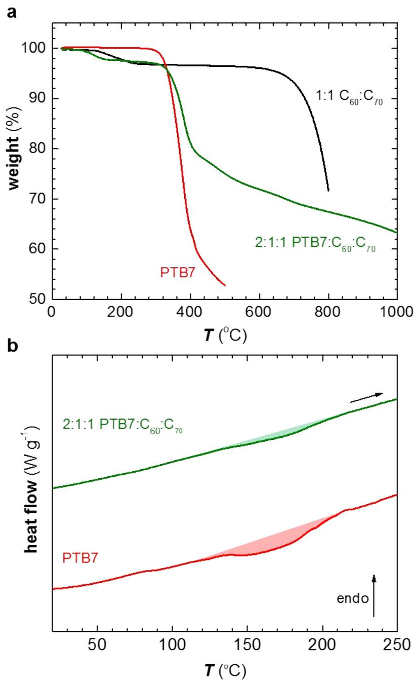
**Fig. S3** (a) TGA scans of PTB7, 1:1  $\text{C}_{60}$ :  $\text{C}_{70}$  and 2:1:1 PTB7: $\text{C}_{60}$ : $\text{C}_{70}$ , (b) DSC second heating thermograms of PTB7 and 2:1:1 PTB7: $\text{C}_{60}$ :  $\text{C}_{70}$  (heating rate 20  $^{\circ}\text{C min}^{-1}$ ). The TGA measurement of 2:1:1 PTB7: $\text{C}_{60}$ : $\text{C}_{70}$  was performed on material that was drop-cast from *o*-DCB and dried under vacuum for two days.
