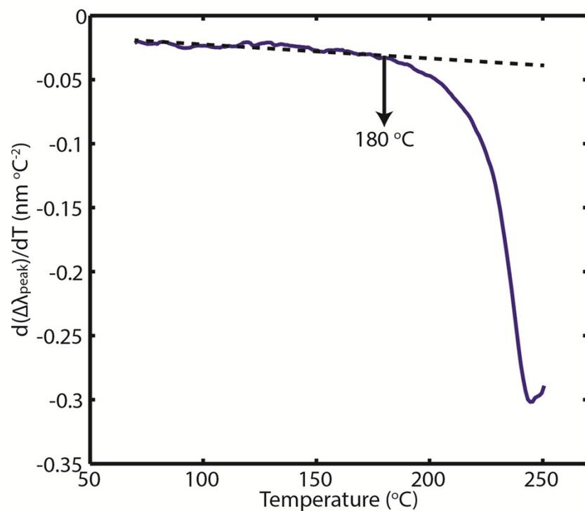
**Fig. S1** Rate by which the peak wavelength  $\Delta\lambda_{peak}$  of the plasmonic resonance changes with temperature,  $d(\Delta\lambda_{peak})/dT$ , i.e. the slope. The onset of the glass transition temperature  $T_g$  is defined as the first point where the value of  $d(\Delta\lambda_{peak})/dT$  deviates from the initial linear region.
