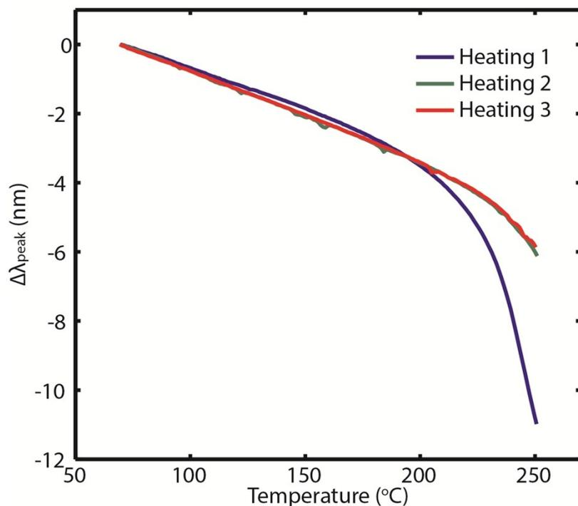
**Fig. S4** The peak wavelength  $\Delta\lambda_{peak}$  of the plasmonic resonance recorded during the first, second and third heating scans of the same 2:1:1 PTB7:C<sub>60</sub>:C<sub>70</sub> film, using a heating rate of 5 °C min<sup>-1</sup> and a natural cooling rate within a temperature interval of 60 to 250 °C.
