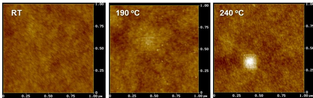
**Fig. S5** AFM topography images of 2:1:1 PTB7:C<sub>60</sub>:C<sub>70</sub> thin films: as spin-coated (left), after annealing for 10 min at 190 °C (centre), and 240 °C (right). AFM images were recorded between crystallites. The surface roughness  $R_{rms}$  was 0.4 nm, 0.5 nm and 0.5 nm, respectively.
