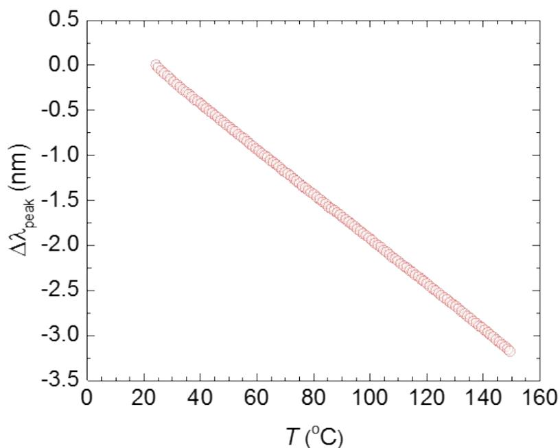
**Fig. S2** Plasmonic nanospectroscopy second heating scan of neat PTB7.
