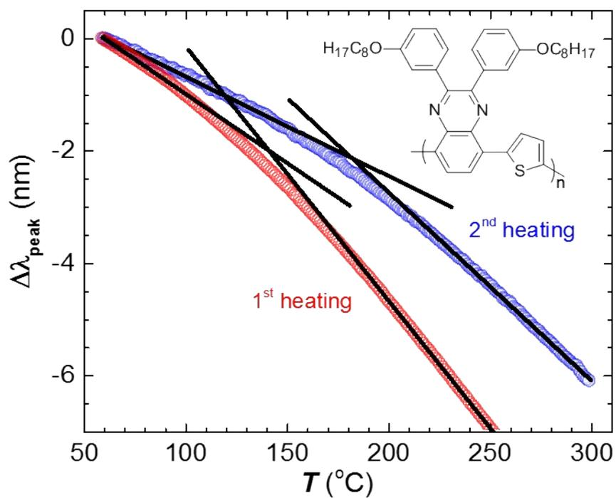
**Fig. S7** Plasmonic nanospectroscopy first (red) and second heating scan (blue) of 2:1:1 TQ1:C<sub>60</sub>:C<sub>70</sub>. The intersection of the straight line fits (black) indicate a thermal transition, which we interpret as the glass transition temperature  $T_g \sim 141$  °C and 182 °C, respectively (inset: chemical structure of TQ1).
