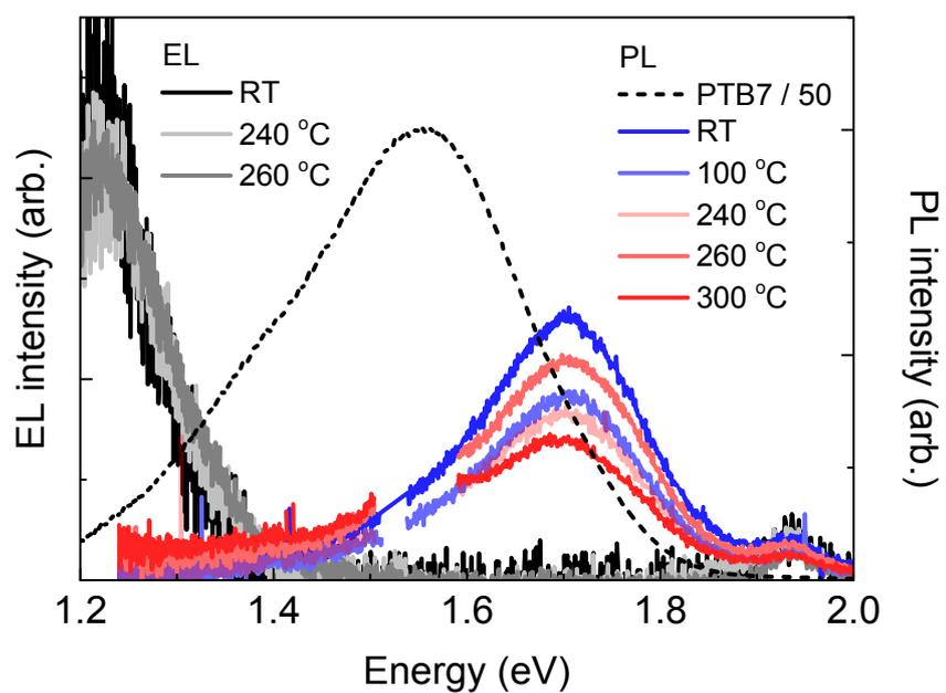
**Fig. S6** (a) Electroluminescence (EL) and photoluminescence (PL) spectra of reference PTB7 and 2:1:1 PTB7:C<sub>60</sub>:C<sub>70</sub> after annealing at temperatures ranging from RT to 300 °C for 10 min.
