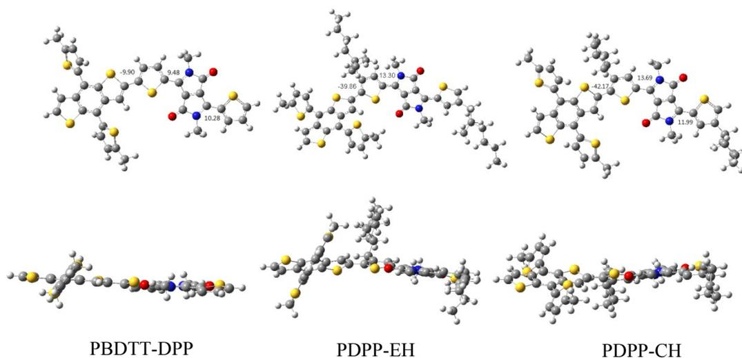
**Figure S2.** Gaussian-predicted (B3LYP/6-31G(d) Level) conformations of PBDTT-DPP, PDPP-EH and PDPP-CH in front view (top) and side view (bottom).
