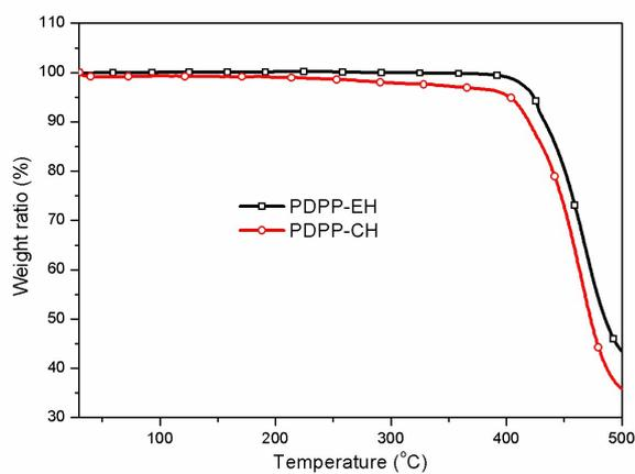
**Figure S1.** TGA curves of polymers PDPP-EH and PDPP-CH at a heating rate of  $10\text{ }^{\circ}\text{C min}^{-1}$  under nitrogen.
