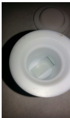
Figure S1. Photograph showing the positioning of the FTO substrate inside the Teflon-lined bomb, at 45° to both the walls and base of the vessel. No dependence was observed on whether the conductive side of the FTO substrate faced towards the bottom of the vessel or towards the top.
