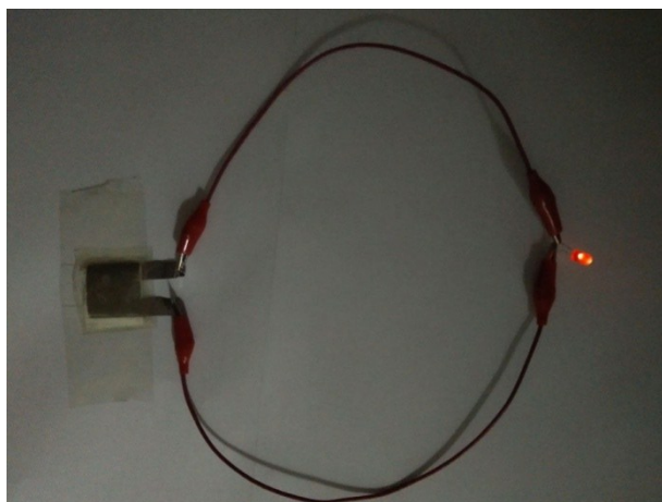
Figure S12. An LED indicator powered by the ASC device.
