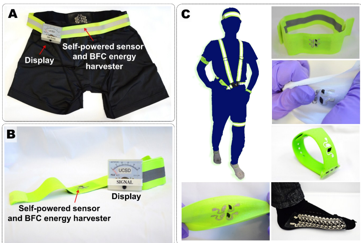
Figure S7. The fully integrated system for wearable lactate biosensing showing the “scavenge-sense-display” concept. The stretchable BFC arrays were printed on (A) the wearable underwear textile and (B) the stretchable strap. (C) Illustration of a ‘green’ model and photographs of wearable energy harvesting system and self-powered BFC array printed on conventional textiles and different body-worn accessories, such as stretchable headbands, straps and socks .
