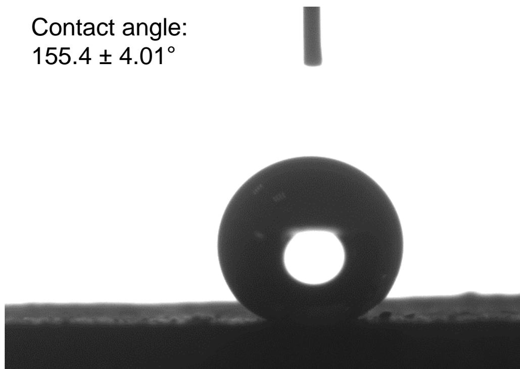
**Figure S8.** Superhydrophobic behavior of the **CalP**-coated surface. A sessile water droplet (7.0 μL) sitting on a **CalP** surface has a contact angle of 155.4 ± 4.01°.
