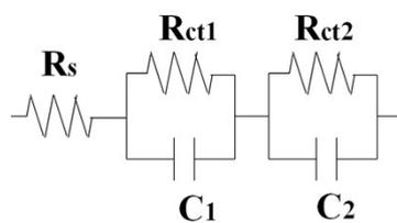
**Figure S3.** Equivalent circuit for fitting EIS in this work.
