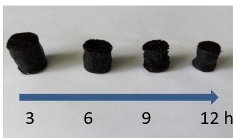
**Figure S5.** Photograph of GH-CuS cylinders prepared under different hydrothermal reaction times.
