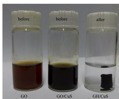
**Figure S2.** Photograph of homogeneous aqueous dispersion of GO, the mixture of GO and CuS, and the resultant cylinder of GH-CuS.
