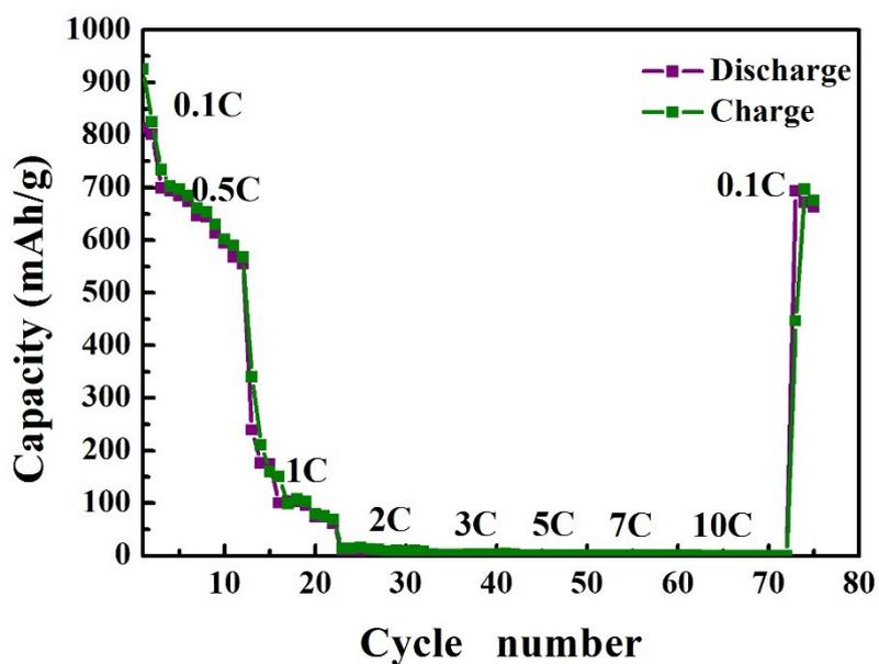
**Figure S7.** Rate capability of pure MoS<sub>2</sub> nanosheet at various current densities of 0.1C, 0.5C, 1C, 2C, 3C, 5C, 7C, 10C, and finally returned to 0.1 C (1C=1A/g). The results show bare MoS<sub>2</sub> exhibited unstable capacity retention and poor high rate performance due to low conductivity of electrode.
