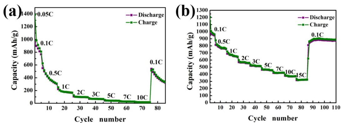
**Figure S8.** Rate capability of Ge/MoS<sub>2</sub> nanocomposites at various weight ratios to evaluate the appropriate parameter at the current densities from 0.1C to 10C, and finally returned to 0.1 C (1C=1A/g). (a) Ge/MoS<sub>2</sub> (1:1) (b) Ge/MoS<sub>2</sub> (4:1)
