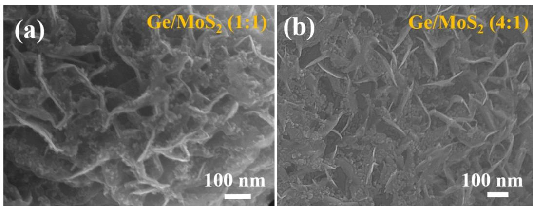
**Figure S6.** SEM images of Ge/MoS<sub>2</sub> nanocomposites with different mixed weight ratios. (a)1:1 (b)4:1
