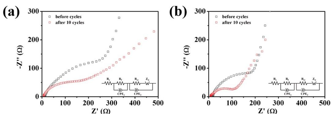
**Figure S5.** Nyquist plots of the Ge/MoS<sub>2</sub> composites (a) before and (b) after annealing with the current density at 0.1 A/g. The equivalent circuit is shown in the inset of (a) and (b).
