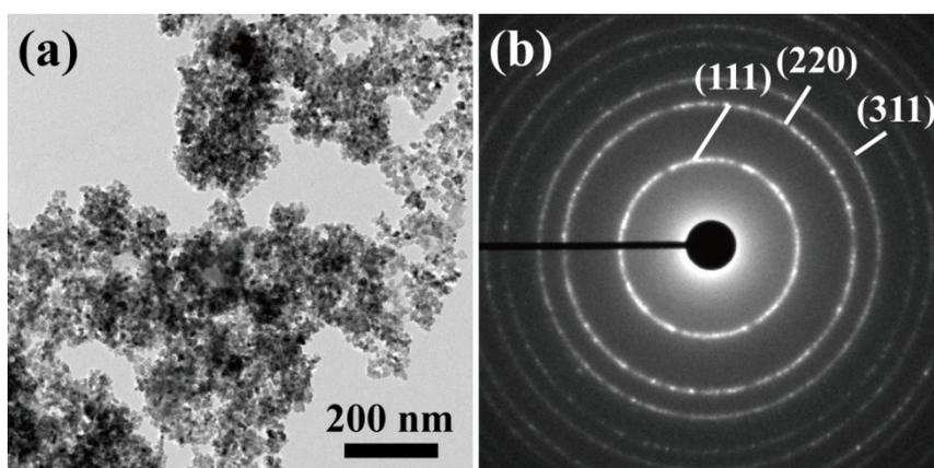
**Figure S4.** (a) TEM image and (b) SAED pattern of the Ge nanoparticles.
