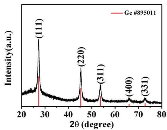
**Figure S3.** XRD pattern of the Ge nanoparticles.
