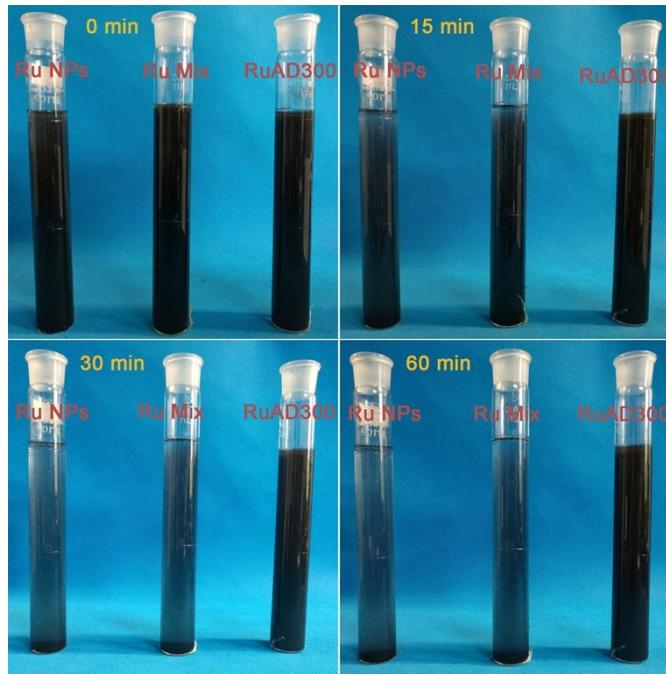
**Fig. S4** The settlement in deionized water for samples of Ru NPs, Ru Mix, and RuAD300 at different times.
