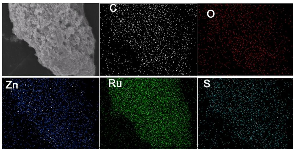
**Fig. S3** FESEM image of RuAD600 and corresponding EDS surface scanning images.
