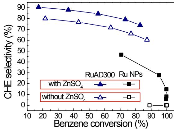
**Fig. S6** Plots of the selectivity of CHE versus the conversion of benzene over Ru NPs and RuAD300 with and without  $\text{ZnSO}_4$ .
