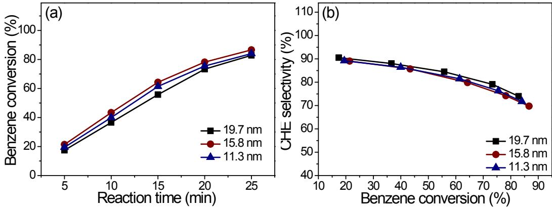
**Fig. S5** Plots of the (a) benzene conversion versus the reaction time and (b) CHE selectivity versus the benzene conversion over different crystallite size of BZSS (300 mg) chemisorbed on Ru NPs.
