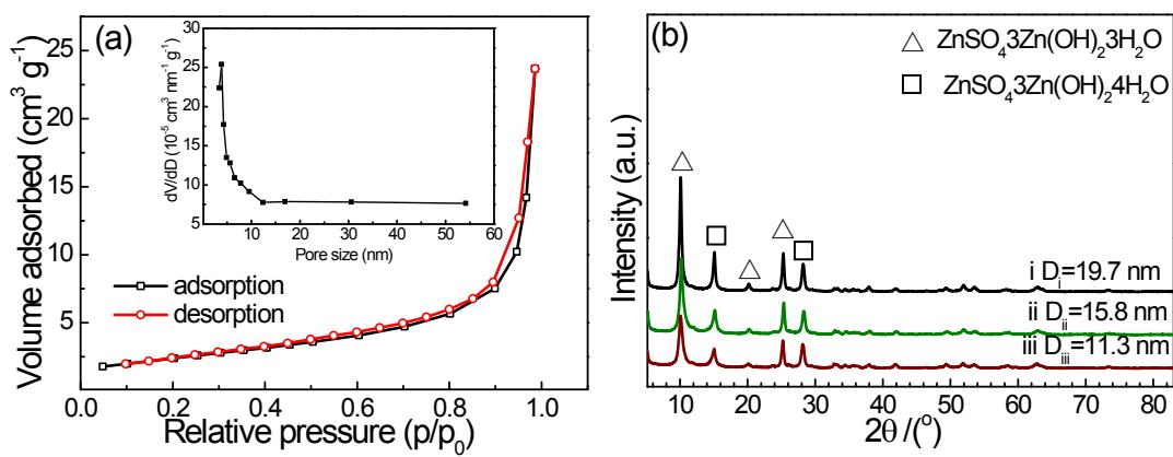
**Fig. S2** (a)  $N_2$  adsorption-desorption isotherms of BZSS, inset is the corresponding Barrett-Joyner-Halenda (BJH) pore size distribution curves. (b) XRD patterns of BZSS with different crystallite size prepared by (i) adding NaOH dropwise, (ii) adding NaOH dropwise,  $ZnSO_4$  excess 50%, (iii) adding NaOH dropwise,  $ZnSO_4$  excess 100%. The crystallite size calculation is according to the Scherrer equation.
