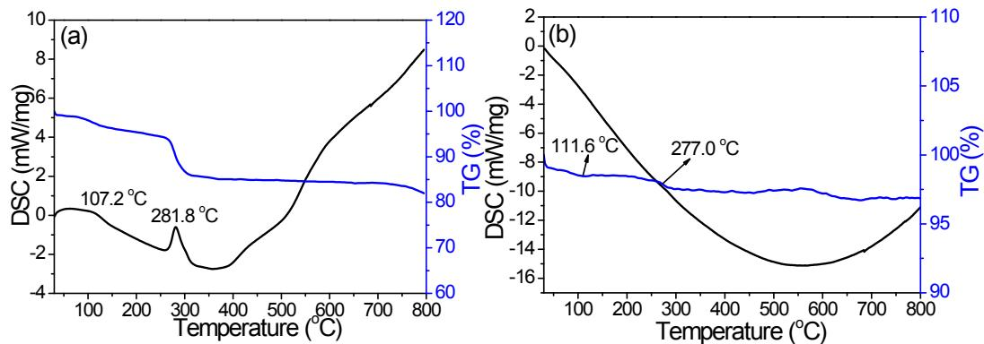
**Fig. S9** TG/DSC curves of (a) BZSS, and (b) RuAD300.
