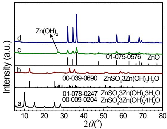
**Fig. S8** XRD patterns of (a) BZSS, and samples calcinated at (b) 200 °C, (c) 300 °C, and (d) 700 °C under N<sub>2</sub> atmosphere.
