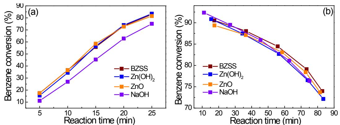
**Fig. S10** Comparisons of the catalytic performance of benzene-selective hydrogenation by chemisorbing of 300 mg BZSS, 196 mg  $\text{Zn}(\text{OH})_2$ , 160 mg  $\text{ZnO}$ , and by adding 158 mg NaOH.
