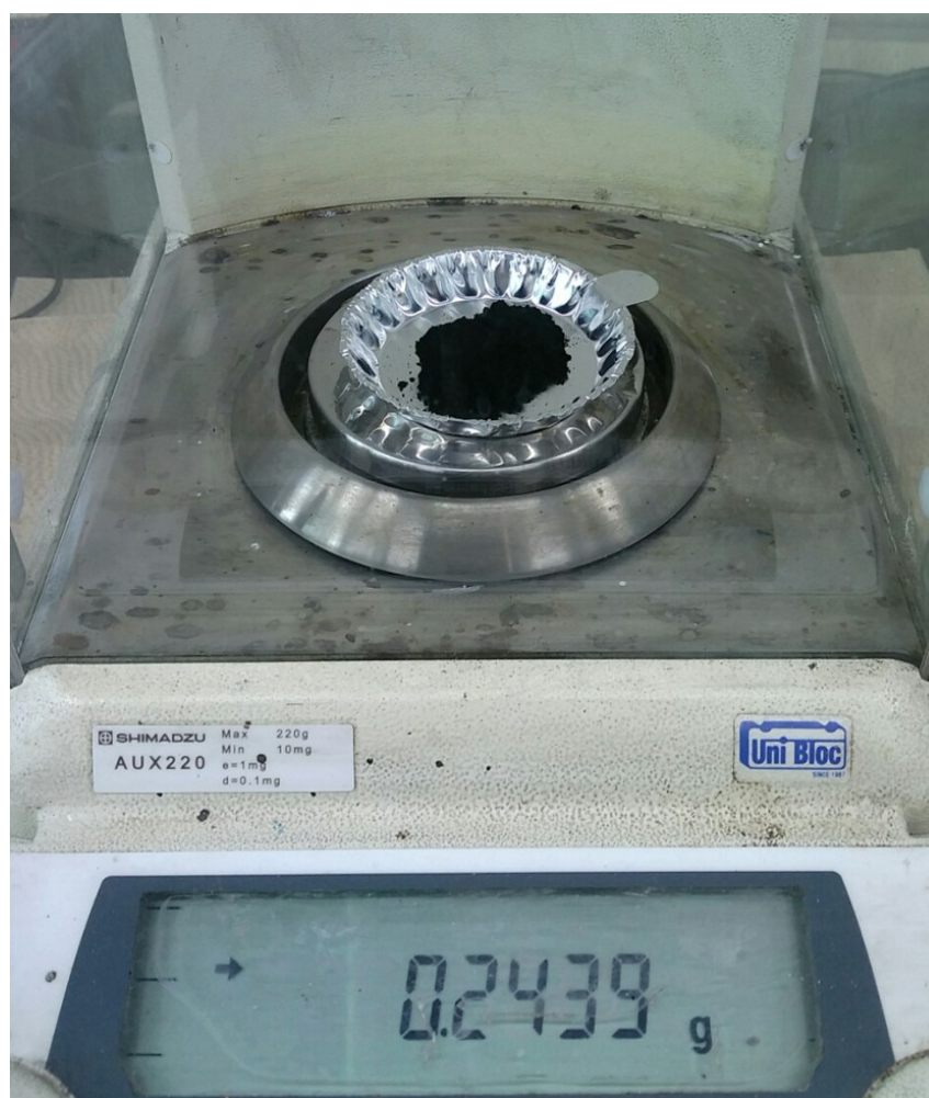
Fig. S2 Large scale synthesis of MCNC/G composites (using 0.15 g of graphene)
