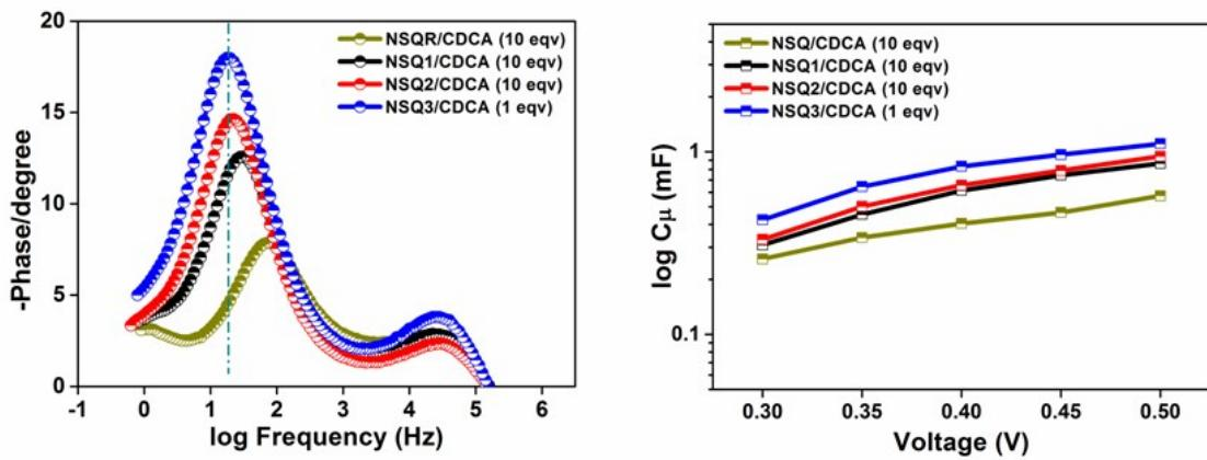
**Figure S51.** (a) Bode plot of NSQ dye cells (with an applied potential of -0.5 V), and (b)  $C_{\mu}$  as a function of voltage (with an applied potential of -0.3 V).
