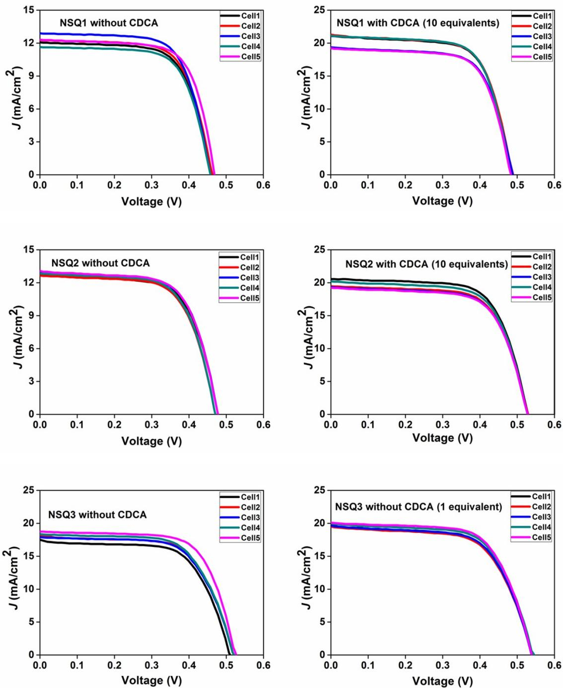
**Figure S49.**  $J$ - $V$  characteristics of **NSQR** and **NSQ1-3** with deviation of 5 cells measured under simulated AM 1.5 G simulated sunlight ( $100 \text{ mW cm}^{-2}$ ).
