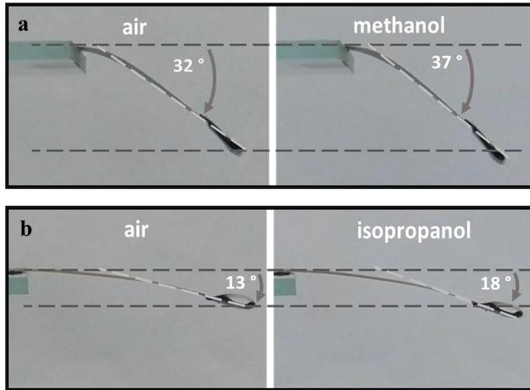
**Figure S11: Vapor induced bending stiffness alteration of bilayer stripe:** Snapshots of the stripes of (a) GO and (b) vermiculite with load applied on one end, before and after exposure to vapors.
