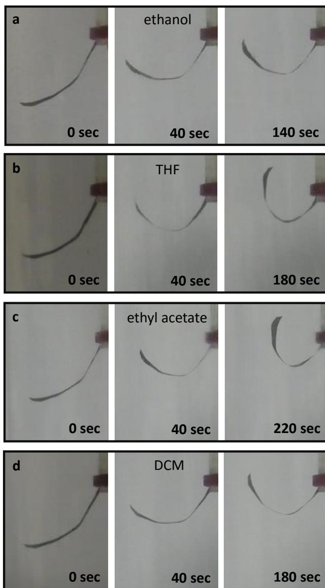
**Figure S6: Vapor assisted bending:** Snapshots of the bending movements of the bilayer stripe upon exposure to (a) ethanol, (b) THF, (c) ethyl acetate and (d) DCM.
