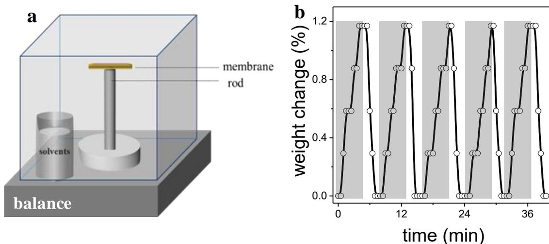
**Figure S9: Reversible adsorption and desorption of solvent vapors by clay-GO bilayer membrane:** (a) Semantic representation of the experimental setup used for measuring weight change of the bilayer membrane. (b) Plot of weight changes versus time of the bilayer membrane during the process of adsorption and desorption of methanol vapor (weight increased portion of the curve shows adsorption of methanol and weight decreased part shows desorption of methanol in air atmosphere).
