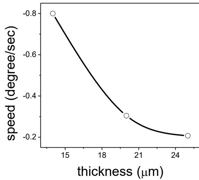
**Figure S7:** Effect of thickness on the bending speed of clay-GO bilayer stripe in presence of methanol vapor.
