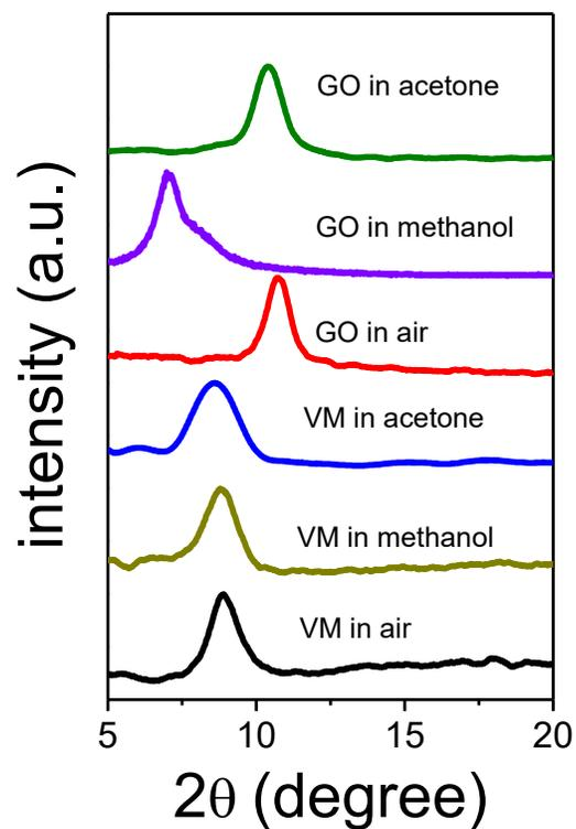
**Figure S12: Alteration of interlayer spacing due to solvent intercalation:** XRD patterns of air-dried GO and vermiculite membrane were compared with the one recorded after wetting the same with methanol and acetone solvents.
