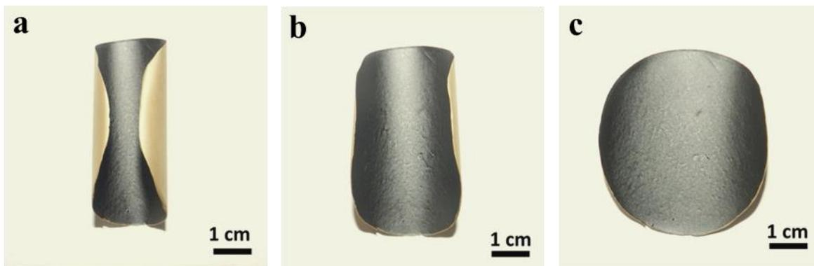
**Figure S1: Humidity driven curling:** Reversible curling of the clay-GO bilayer membrane as a function of relative humidity at 23 °C. (a) 78%. (b) 87% and (c) 95 % humidity.
