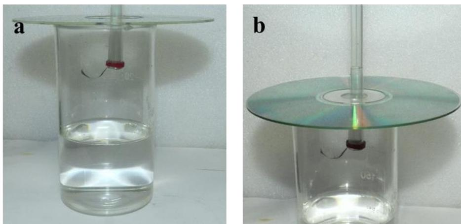
**Figure S5: Experimental setup:** Digital photos of the experimental setup utilized for the investigation of vapor stimulated bending properties of clay-GO bilayer membrane (a) side view and (b) top view of the experimental set up.
