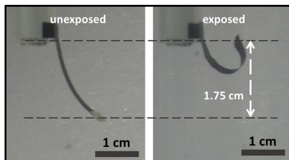
**Figure S8: Work done by the bilayer stripe:** Vapors assisted weight lifting by the bilayer stripe.
