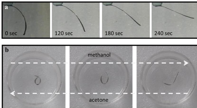
**Figure S10, Responsiveness of bilayer membrane:** (a) Bending of bilayer stripe against gravity in methanol environment. (b) Reversible curling and opening of the stripe in methanol-acetone system keeping both the ends unrestricted.
