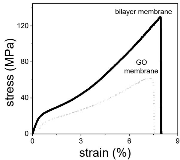
**Figure S4: Stress-stain curve:** Stress-stain curve of GO and clay-GO bilayer membrane (43 weight % of the GO membrane was replaced by vermiculite in the bilayer membrane).
