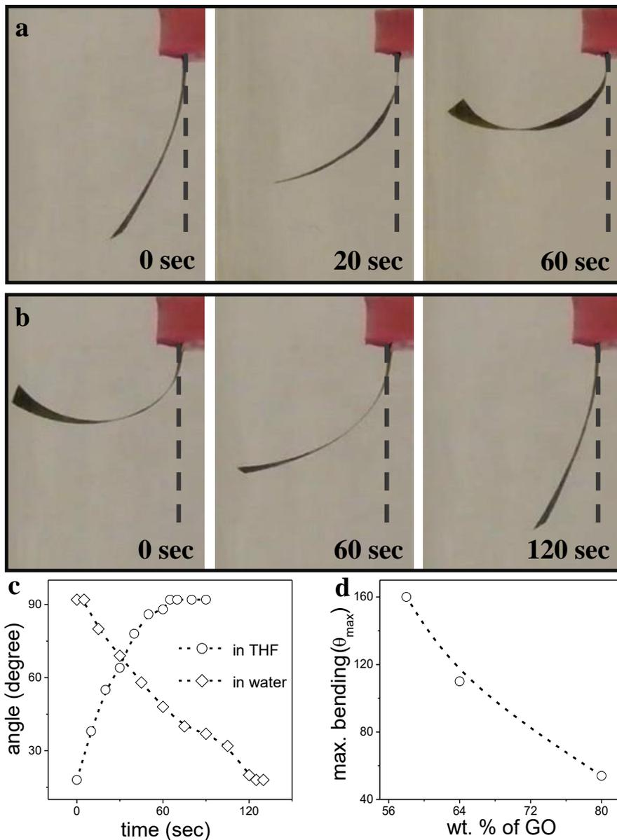
**Figure S13: THF and water assisted bending of bilayer stripe:** (a) Photos of bilayer stripe inside liquid THF after 0, 20, and 60 seconds of insertion. (b) Snapshots showing recovery of the bilayer stripe inside water at 0, 60, and 120 seconds. (c) Time versus bending angle plot in THF and water solvent. (d) Maximum bending of bilayer stripe in THF-water system as a function of GO content (weight %) in the membrane.
