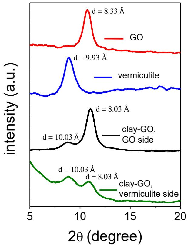
**Figure S2: XRD patterns of membranes:** XRD patterns of air dried GO, vermiculite and clay-GO bilayer membranes, exposing GO side and vermiculite side of the bilayer membrane.
