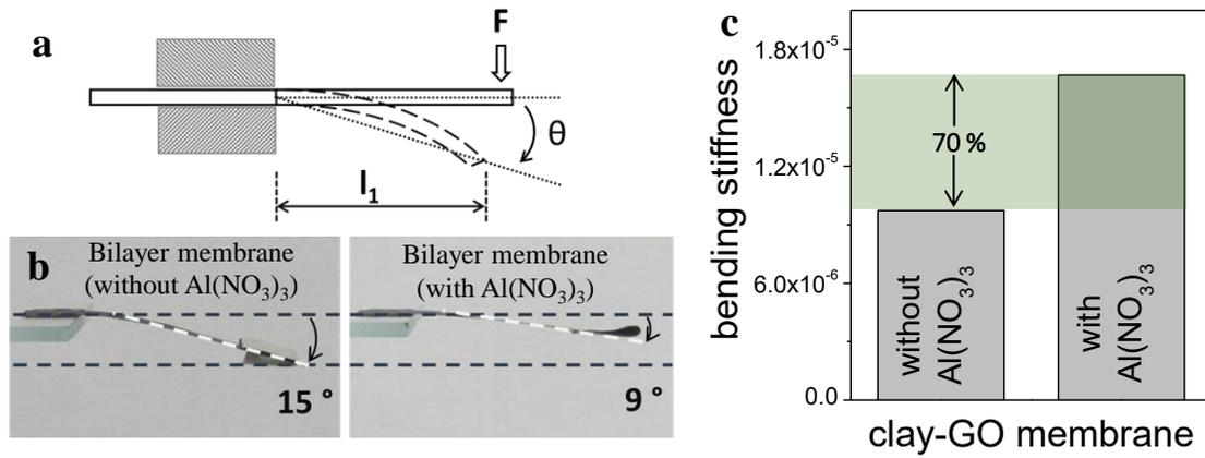
**Figure S3: Bending stiffness of clay-GO bilayer membranes:** (a) Schematic representation of bending stiffness measurements using 2 – point method. (b) Snapshots of the stripes of clay-GO bilayer membrane with load applied on the free end. (c) Comparison of the bending stiffness of the clay-GO membrane with and without addition of  $\text{Al}(\text{NO}_3)_3$ .
