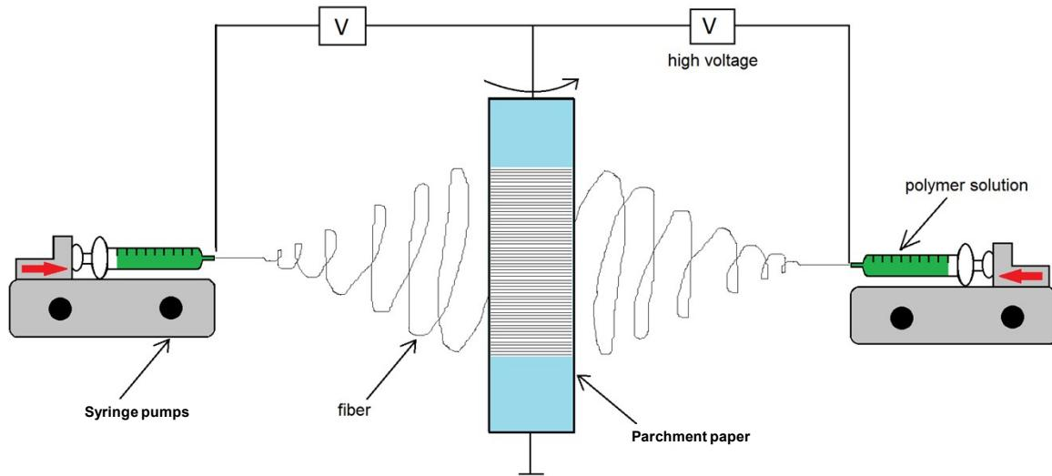
**Fig. S1.** Schematic illustration of the electrospinning setup for preparing large scale fibers.
