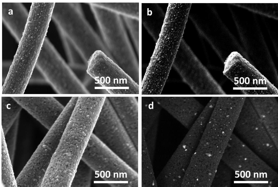
**Fig. S3.** HR-SEM micrographs of an electrospun fiber containing nickel nanoparticles after carbonization step under argon at (a, b) 600 and (c, d) 700 °C, respectively, for 3 h before CVD process. a) and c) are secondary electron SEM pictures whereas b) and d) are back scattered electron SEM pictures highlighting the nickel nanoparticles as white spots available at the carbon fiber surface.
