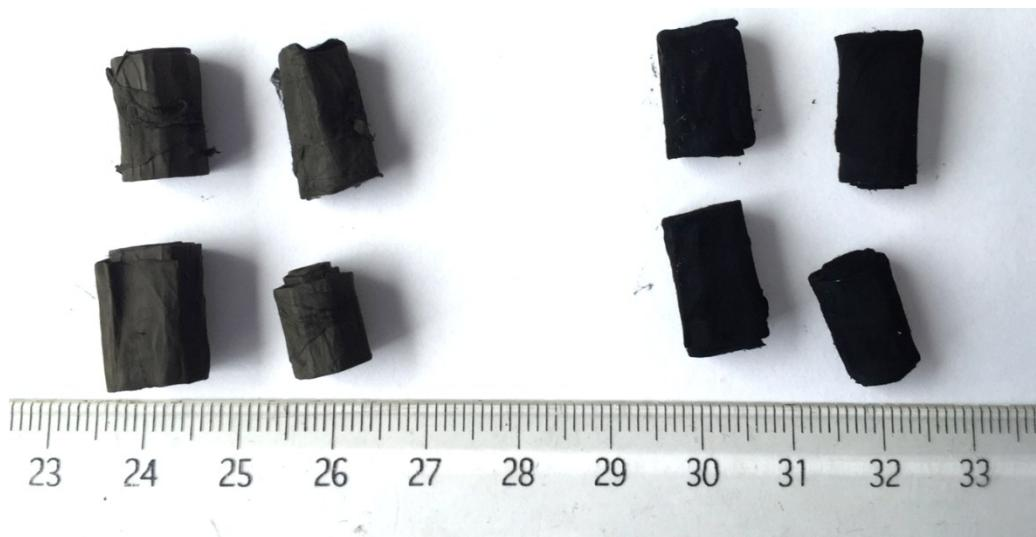
**Fig. S4.** Digital photos of macroscopic cylindrical shapes of Ni/CNF (left) and hierarchical CF/CNF after CVD process (right).
