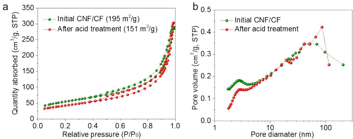
**Fig. S7.**  $\text{N}_2$  adsorption -desorption isotherms and pore size distribution calculated by BJH method of the CNF/CF composite (CNF/CF700-700/2-2) before and after acid treatment.
