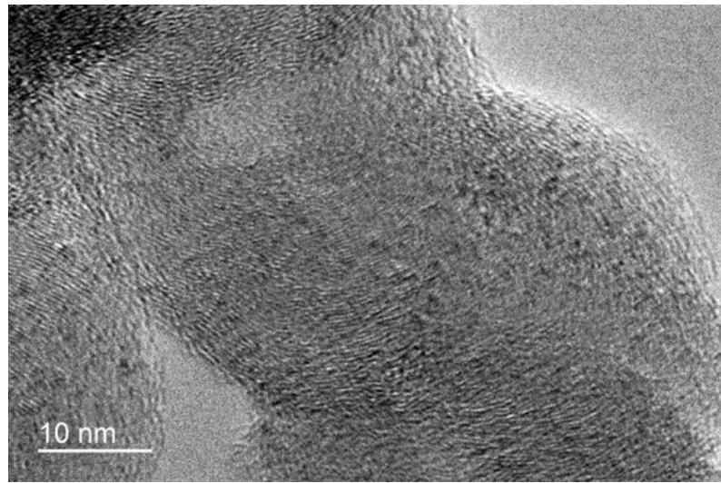
**Fig. S5.** HR-TEM micrographs of typical carbon nanofibers grown by CVD process from Ni/CF sample showing the presence of prismatic planes along the fiber axis.
