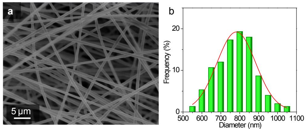
**Fig. S2.** SEM image of as-spun organic fibers and the corresponded diameter distribution.
