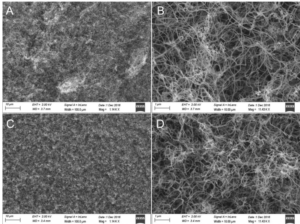
**Fig. S6.** SEM micrographs of a CF/CNF/800-800/120-120 monolith (A, B) before and (C, D) after ultrasonic treatment showing the high adhesion strength of the carbon nanofibers to the carbon fibers.
