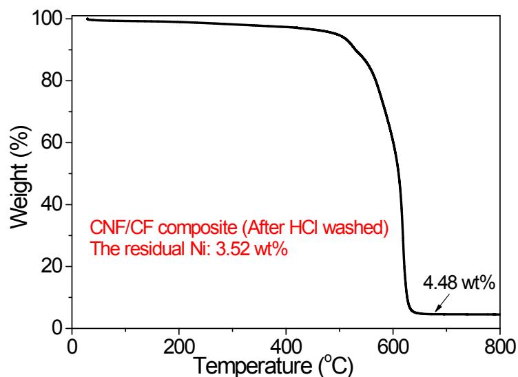
**Figure S8.** TGA result performed under air of the CF/CNF monolith after HCl treatment presenting 3.53 wt % of Ni residue covered by graphical carbon wall which could not be removed by concentrated HCl solution.
