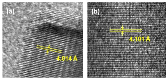
**Fig. S4** HR-TEM lattice images along  $[001]$  of (a) pristine  $\text{Mg}_x\text{Mo}_{2.5+y}\text{VO}_{9+z}$  ( $x = 0$ ) and (b) Mg-inserted product ( $x = 2$ ), showing a slight expansion of the  $c$  parameter (layer stacking direction), which is consistent with an expansion observed by the profile fitting.
