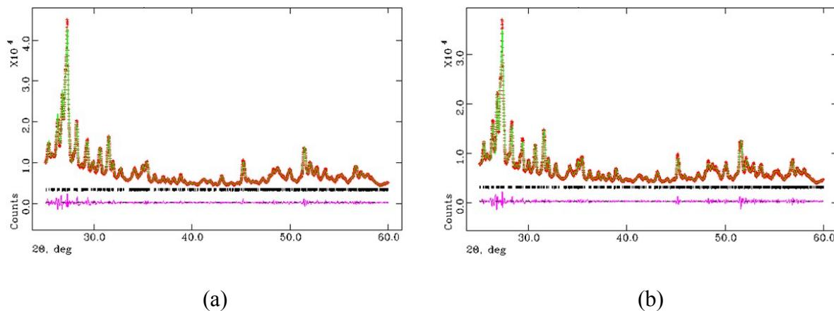
**Fig. S8** Le Bail refinements of (a) the parent host compound  $\text{Mo}_{2.48}\text{VO}_{9.93}$  and (b) Mg-inserted  $\text{Mg}_x\text{Mo}_{2.48}\text{VO}_{9.93}$  ( $x = 2$ ) prepared by the microwave-assisted chemical insertion:  $Pba2$ ,  $wR_p = 3.14\%$ , lattice parameters  $a = 21.2675(2)$  Å,  $b = 26.7935(3)$  Å, and  $c = 4.1006(3)$  Å (measured, orange; calculated, green; difference, pink; Bragg reflections, vertical tick marks).
