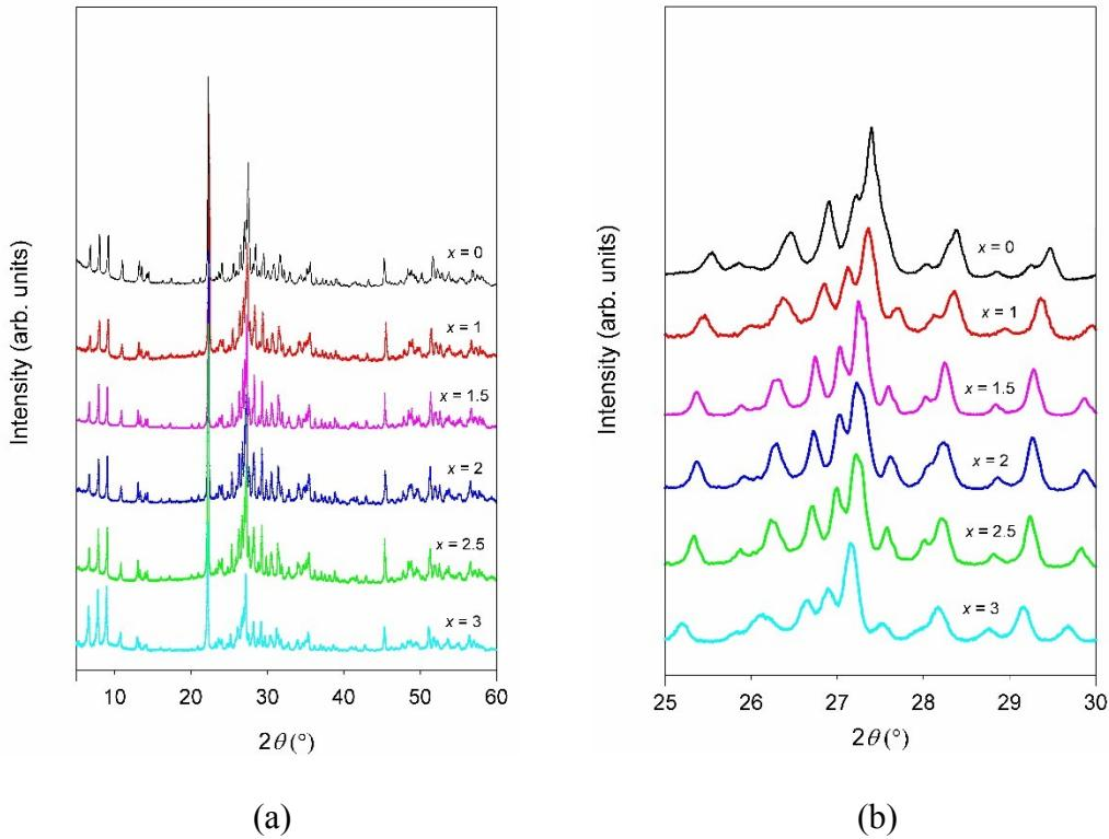
**Fig. S3** (a) PXRD patterns of  $\text{Mg}_x\text{Mo}_{2.5+y}\text{VO}_{9+z}$  ( $0 \leq x \leq 3$ ) prepared by the microwave-assisted chemical insertion with DEG and  $\text{Mg}(\text{CH}_3\text{COO})_2$ . (b) PXRD patterns at selected  $2\theta$  range (25–30°) to illustrate the changes in the peak positions.
