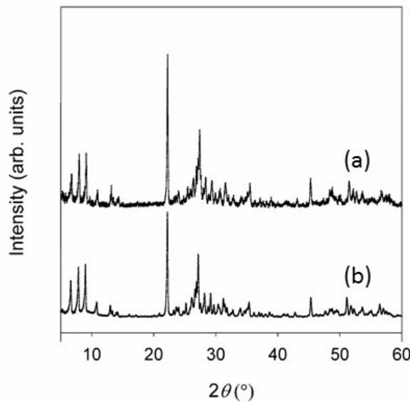
**Fig. S12** X-ray diffraction pattern of  $\text{Mg}_x\text{Mo}_{2.5+y}\text{VO}_{9+z}$  electrode mixture (a) recovered from a cell at the end of first charge (after a complete removal of  $\text{Mg}^{2+}$ ) compared to (b) that of a fresh Mg-inserted compound  $\text{Mg}_x\text{Mo}_{2.5+y}\text{VO}_{9+z}$  with  $x = 1.6$ , indicating that the host framework  $\text{Mo}_{2.5+y}\text{VO}_{9+z}$  is maintained after the electrochemical extraction of  $\text{Mg}^{2+}$  ions.
