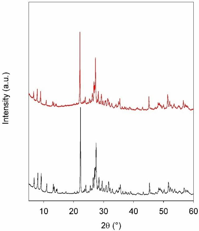
**Fig. S1** Powder X-ray diffraction patterns of as-synthesized  $\text{Mo}_{2.5+y}\text{VO}_{9+z}$  from microwave-assisted hydrothermal reaction (red) and microporous  $\text{Mo}_{2.5+y}\text{VO}_{9+z}$  after calcination at 400 °C (black).
