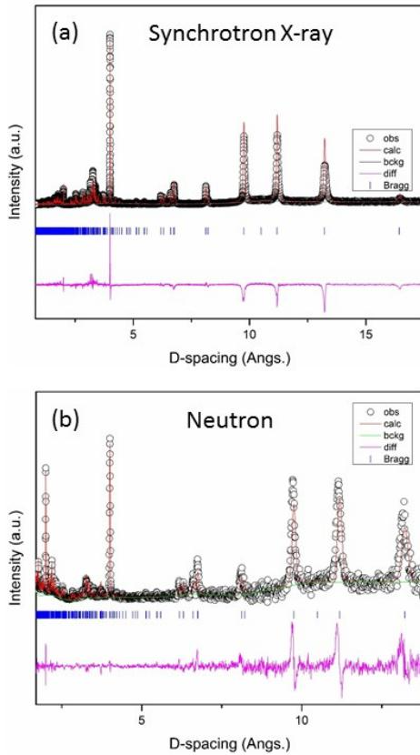
**Fig. S14** (a) SXRD data and (b) NPD data (POWGEN Bank 5, wavelength 3.731 Å) from joint neutron and synchrotron X-ray Rietveld refinement of  $\text{Mg}_x\text{Mo}_{2.5+y}\text{VO}_{9+z}$  ( $x = 0.2$ ).
