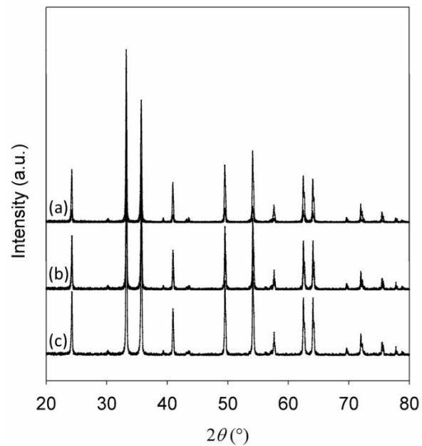
**Fig. S7** PXRD patterns of  $\text{Li}_x\text{Fe}_2\text{O}_3$  prepared by the microwave-assisted chemical insertion: (a)  $x = 0.03$ , (b)  $x = 0.14$ , and (c)  $x = 0.15$ .
