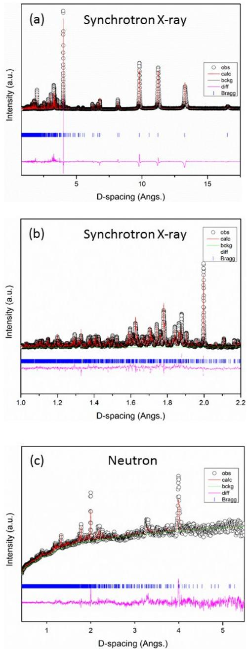
**Fig. S15** Joint neutron and synchrotron X-ray Rietveld refinement of the Mg-inserted compound  $\text{Mg}_x\text{Mo}_{2.5+y}\text{VO}_{9+z}$ ,  $x = 1$ : (a) and (b) SXRD data. (c) NPD data from POWGEN Bank 3, wavelength 1.333 Å.
