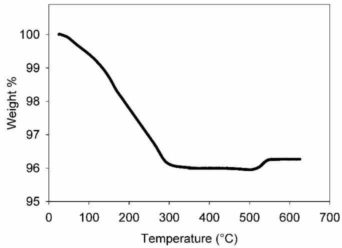
**Fig. S2** Thermogravimetric analysis of the as-synthesized  $\text{Mo}_{2.5+y}\text{VO}_{9+z}$  in oxygen atmosphere.
