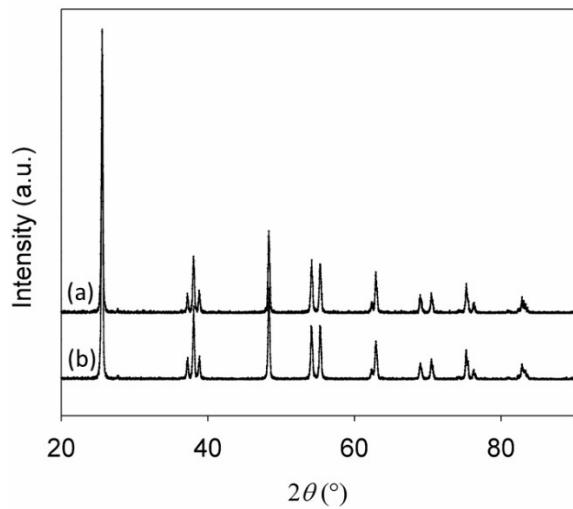
**Fig. S6** PXRD patterns of  $\text{Li}_x\text{TiO}_2$  prepared by the microwave-assisted chemical insertion: (a)  $x = 0.48$  and (b)  $x = 0.62$ .
