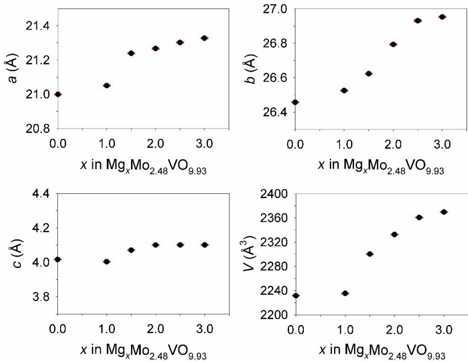
**Fig. S9** Unit cell parameters of  $\text{Mg}_x\text{Mo}_{2.5+y}\text{VO}_{9+z}$  ( $0 < x \leq 3$ ) prepared by the microwave-assisted chemical insertion with DEG and  $\text{Mg}(\text{CH}_3\text{COO})_2$ , from Le Bail refinements (error bars in red).
