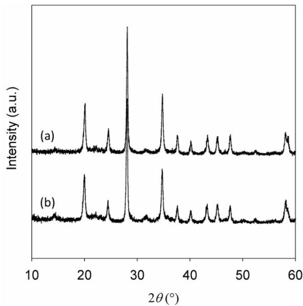
**Fig. S5** PXRD patterns of  $\text{Li}_x\text{VOPO}_4$  prepared by the microwave-assisted chemical insertion: (a)  $x = 1.31$  and (b)  $x = 1.55$ .
