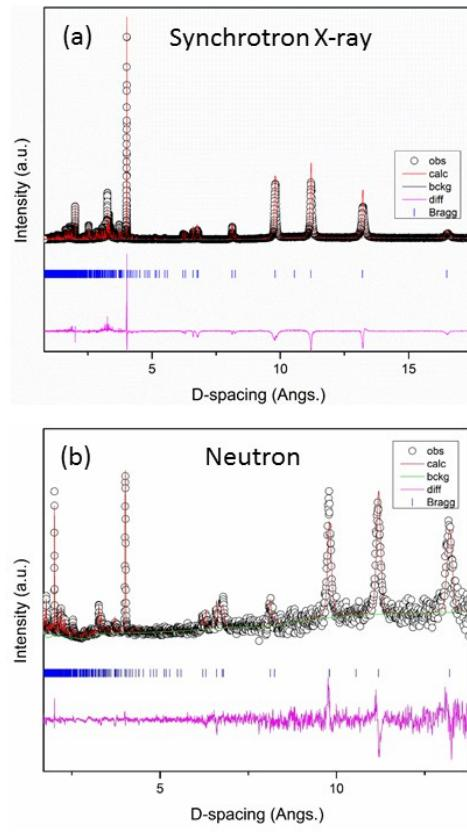
**Fig. S13** (a) SXRD data and (b) NPD data (POWGEN Bank 5, wavelength 3.731 Å) from joint neutron and synchrotron X-ray Rietveld refinement of the parent host compound  $\text{Mo}_{2.5+y}\text{VO}_{9+z}$ .
