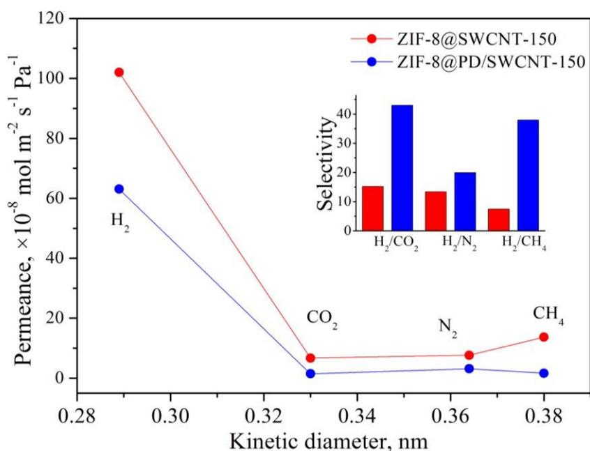
**Figure S10.** Comparison of gas permeance and ideal gas selectivity between ZIF-8 membranes grown on PD/SWCNT-150 and SWCNT-150 without PD wrapping measured under the same condition.
