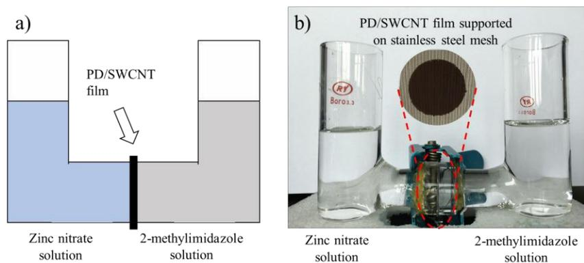
**Figure S3.** Diagrammatic sketch (a) and photography (b) of a homemade two-cell diffusion setup.
