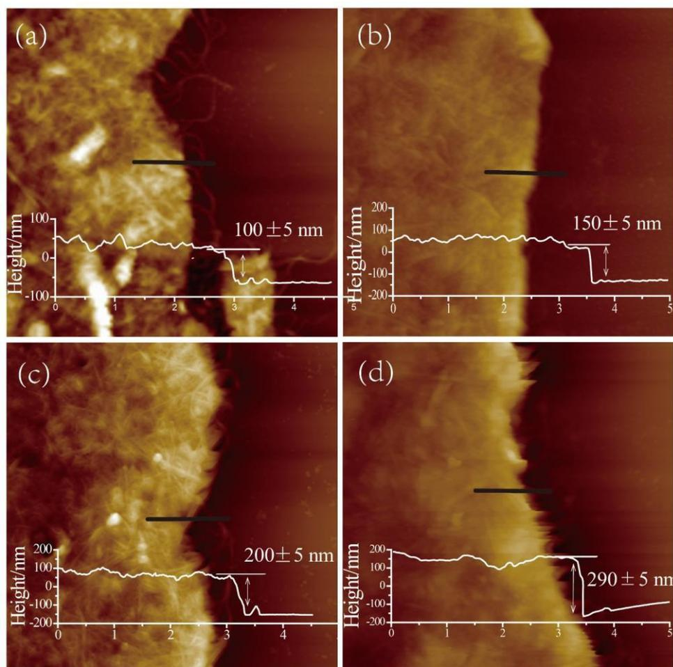
**Figure S2.** AFM images and their height profiles of PD/SWCNT films with different thickness: (a)  $\sim 100$  nm, (b)  $\sim 150$  nm, (c)  $\sim 200$  nm, and (d)  $\sim 290$  nm.
