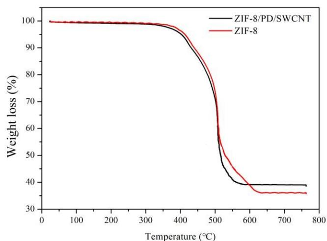
**Figure S5.** Thermogravimetric analysis (TGA) curves of ZIF-8 crystal and ZIF-8 composite membrane measured in a flow of air.
