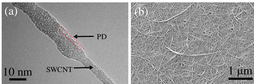
**Figure S1.** (a) TEM image of an individual polydopamine (PD)-wrapped SWCNT. (b) SEM image of PD/SWCNT film.
