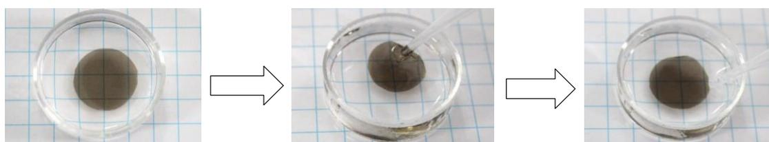
**Figure S4.** Digital photos of a ZIF-8 membrane floating on an acetone/water surface which could be lifted up by a pipette without cracking.
