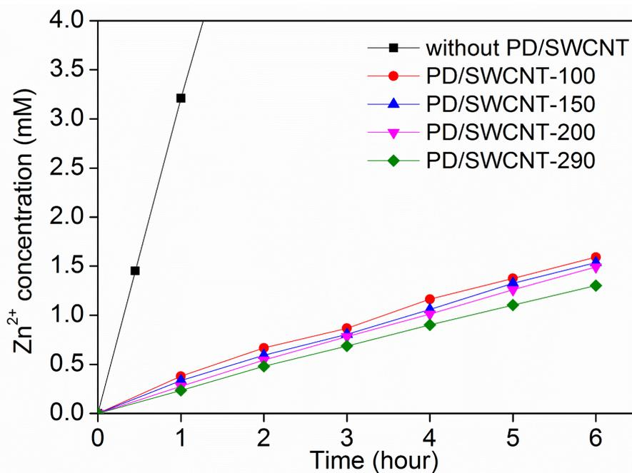
**Figure S7.** Variation of  $Zn^{2+}$  concentration vs diffusion time through PD/SWCNT films with different thicknesses.
