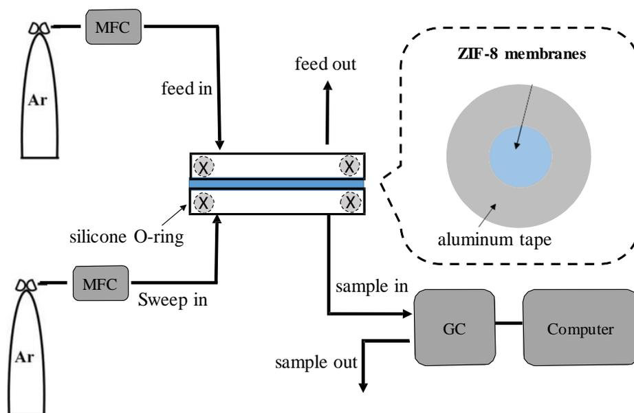
**Figure S8.** Illustration of the gas separation measurement apparatus used in this work.
