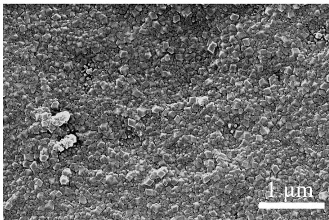
**Figure S9.** SEM image of ZIF-8 membrane grown on SWCNT-150 without PD wrapping.
