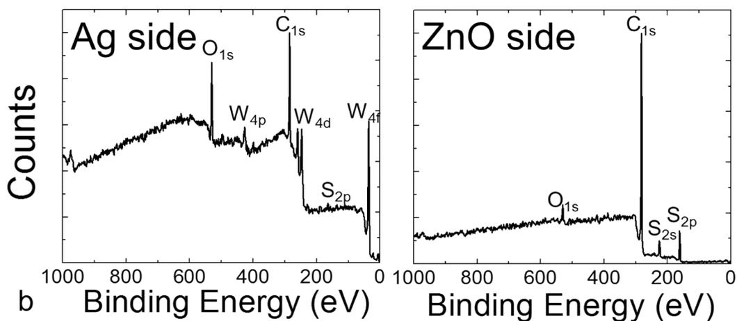
Figure S9: The XPS survey scans measured from the fractured Ag/WO<sub>3</sub> sample that was aged one week. The metal side is shown on the left and the ZnO side on the right.
