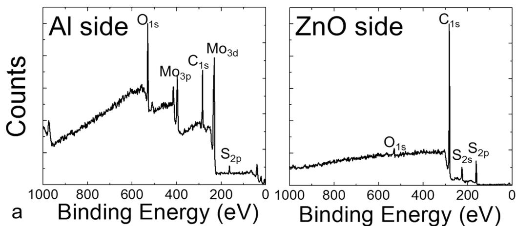
Figure S4: The XPS survey scans measured from the fractured unaged Al/MoO<sub>3</sub> sample. The metal side is shown on the left and the ZnO side on the right.
