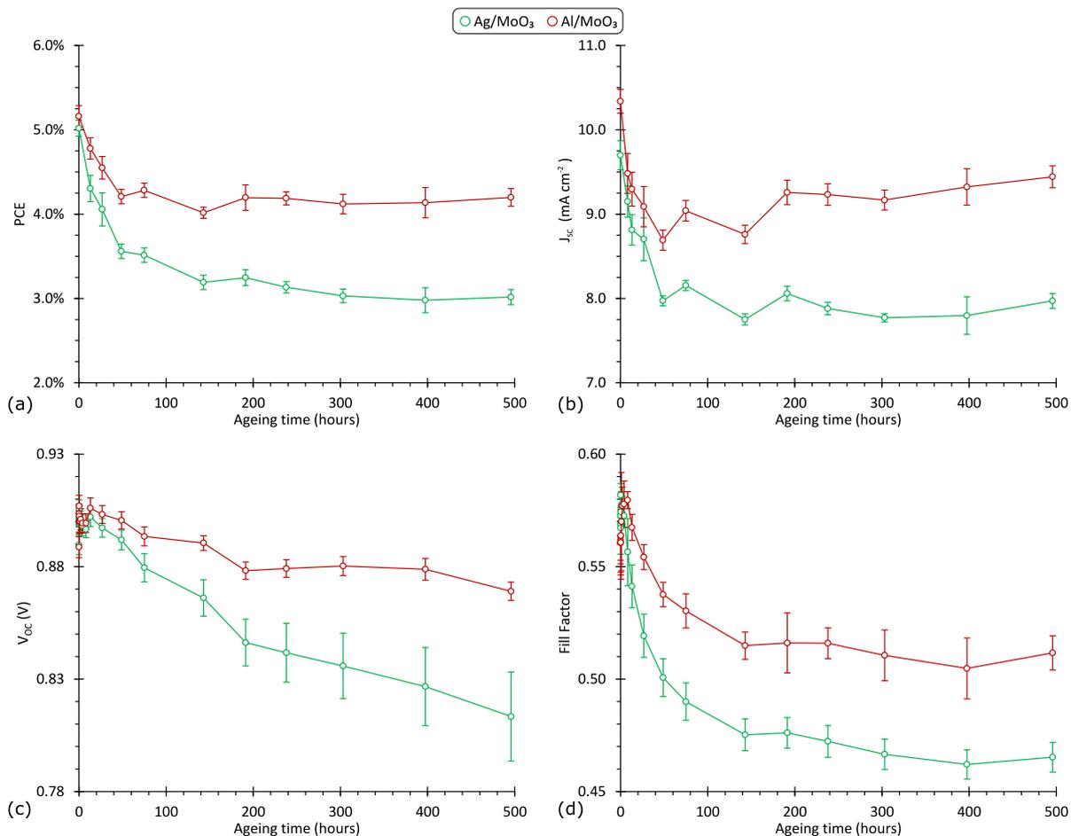
Figure S1: The evolution of the PCE (a),  $J_{sc}$  (b), the  $V_{oc}$  (c), and the fill factor (d) of the PCDTBT:PC<sub>71</sub>BM inverted OPV devices with thermal ageing in the dark in an inert atmosphere. The devices have MoO<sub>3</sub> HTLs and either aluminium or silver top electrodes. The uncertainties represent one standard deviation when averaged across 12 devices.
