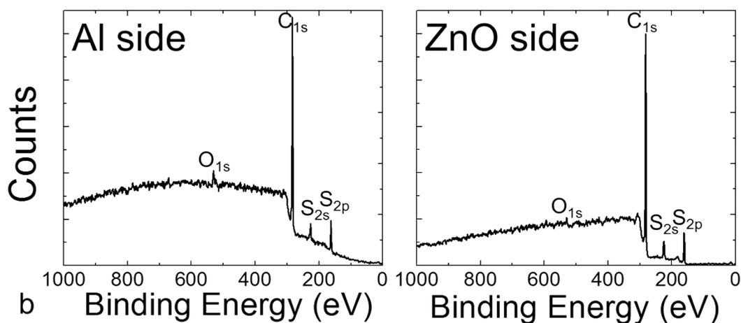
Figure S5: The XPS survey scans measured from the fractured unaged Al/WO<sub>3</sub> sample. The metal side is shown on the left and the ZnO side on the right.
