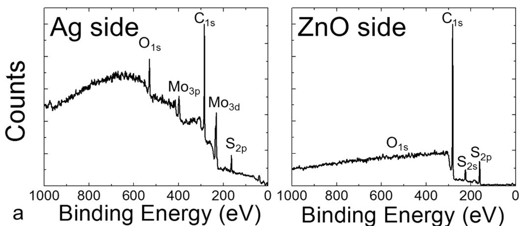
Figure S8: The XPS survey scans measured from the fractured Ag/MoO<sub>3</sub> sample that was aged one week. The metal side is shown on the left and the ZnO side on the right.
