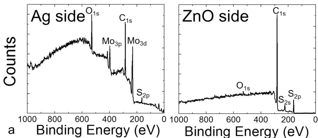
Figure S6: The XPS survey scans measured from the fractured unaged Ag/MoO<sub>3</sub> sample. The metal side is shown on the left and the ZnO side on the right.
