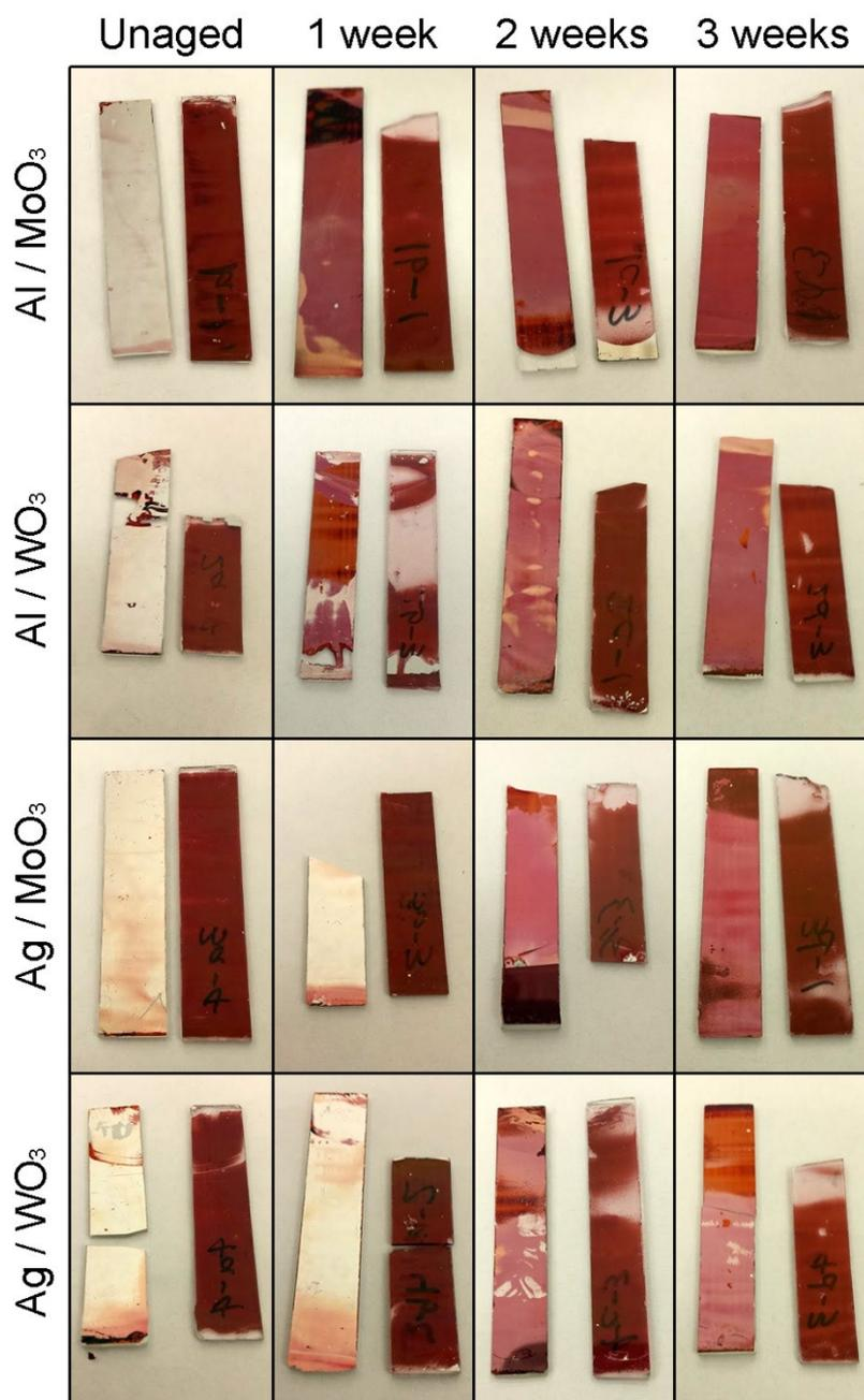
Figure S3: Photographs of fractured samples from each top electrode/HTL material combination that have been thermally aged for between 0 and 3 weeks at 85°C in the dark under an inert atmosphere. In each image, the “metal side” fractured half is shown on the left, and the “ZnO side” half on the right. A sample that fractures in the BHJ exhibits purple colouration of both halves, while those that fracture at the HTL/BHJ interface only exhibit purple colouration on the ZnO side.
