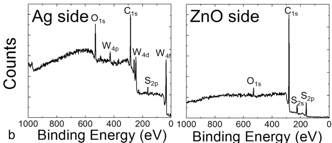
Figure S7: The XPS survey scans measured from the fractured unaged Ag/WO<sub>3</sub> sample. The metal side is shown on the left and the ZnO side on the right.
