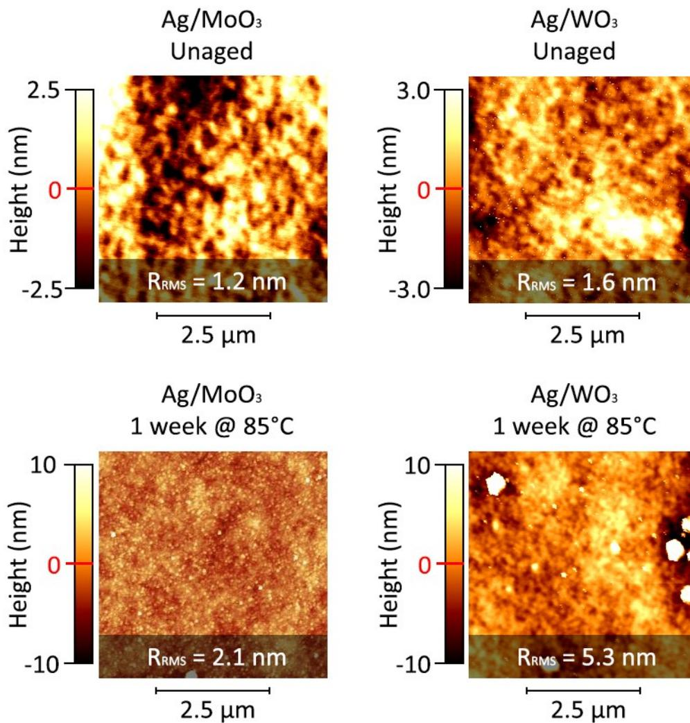
Figure S10: AFM topography data obtained from the fractured silver-containing samples that underwent XPS depth profiling. The RMS roughness ( $R_{RMS}$ ) values are superimposed on the micrographs, indicating only minor changes in roughness occur with thermal ageing.
