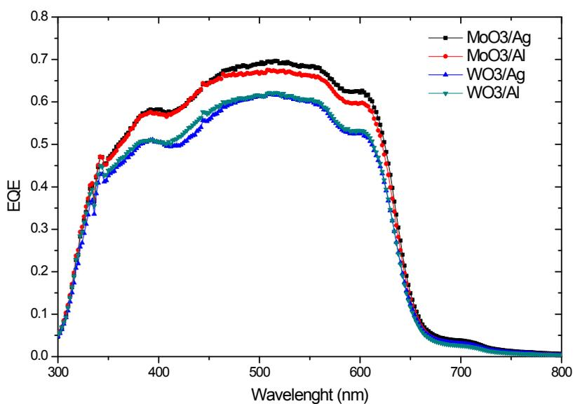
Figure S2: EQE spectra of P3HT:PCBM organic solar cells with different combination of top electrode (MoO<sub>3</sub>/Ag, MoO<sub>3</sub>/Al, WO<sub>3</sub>/Ag and WO<sub>3</sub>/Al).
