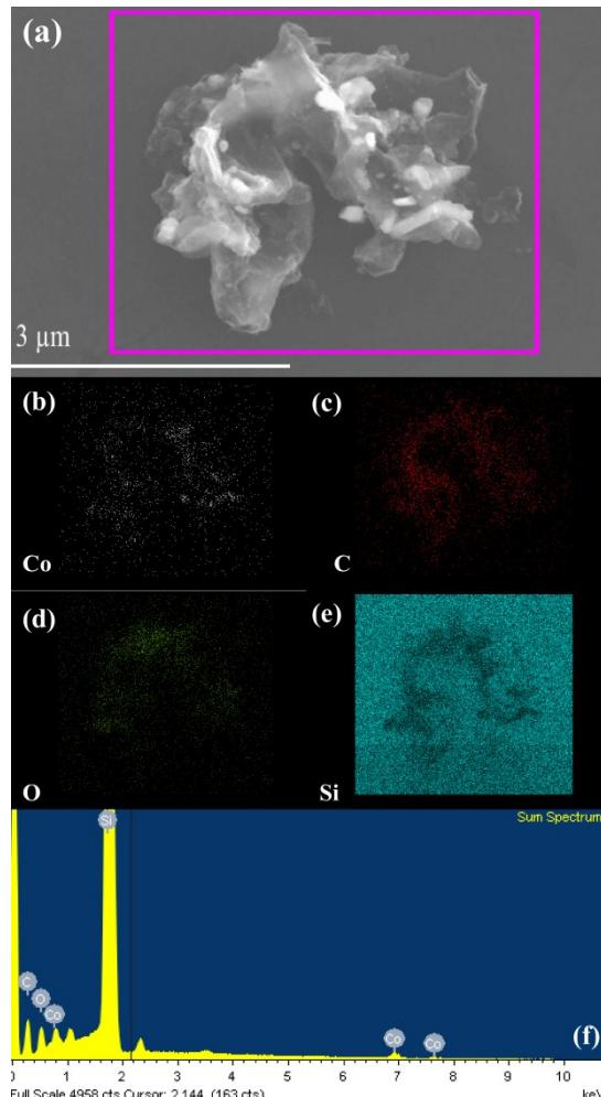
Figure S1. (a) SEM image, elemental mapping of (b) cobalt (c) carbon (d) oxygen (e) silicon substrate, and (f) EDS spectrum of Co<sub>2</sub>C/rGO.
