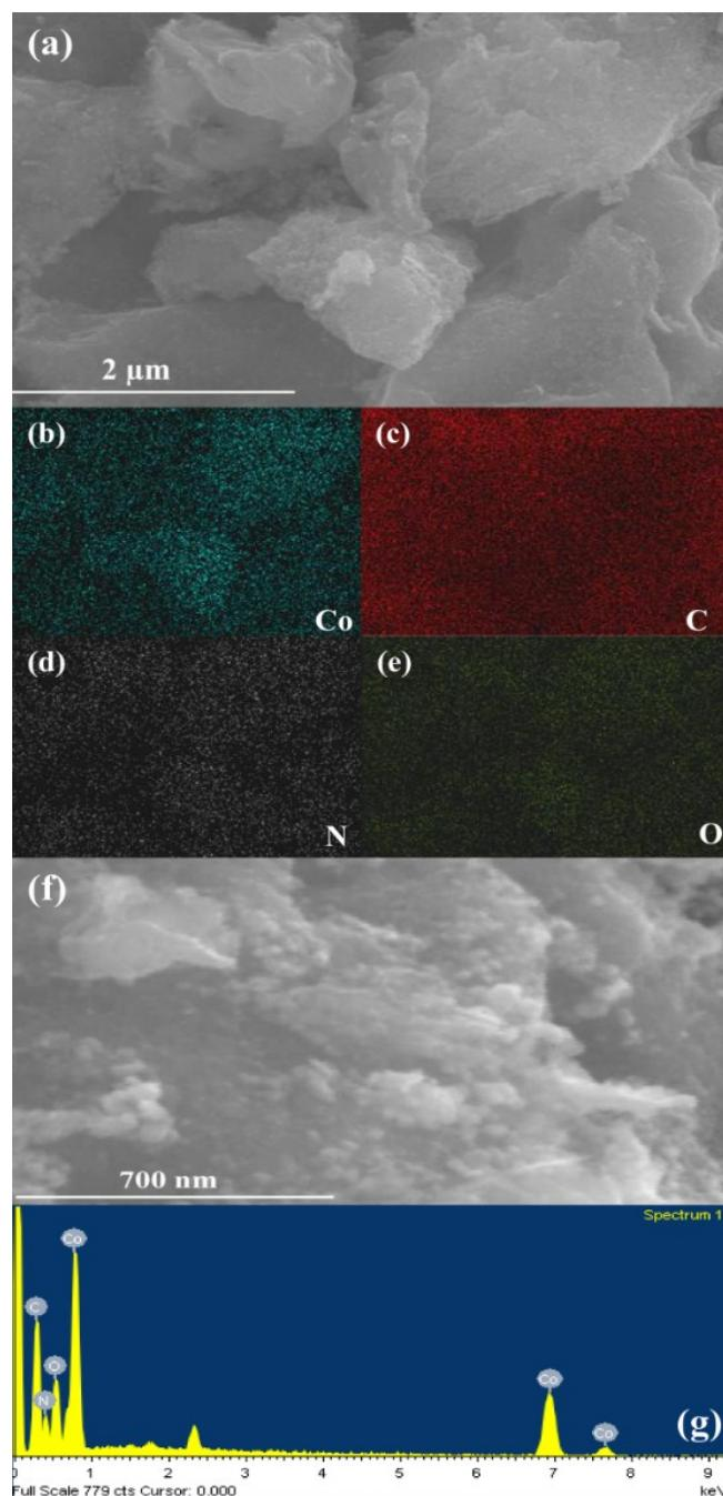
Figure S2. (a) SEM image, corresponding elemental mapping of (b) cobalt (c) carbon (d) nitrogen (e) oxygen. (f) SEM image and (g) EDS spectrum of  $\text{Co}_4\text{N}/\text{rGO}$ .
