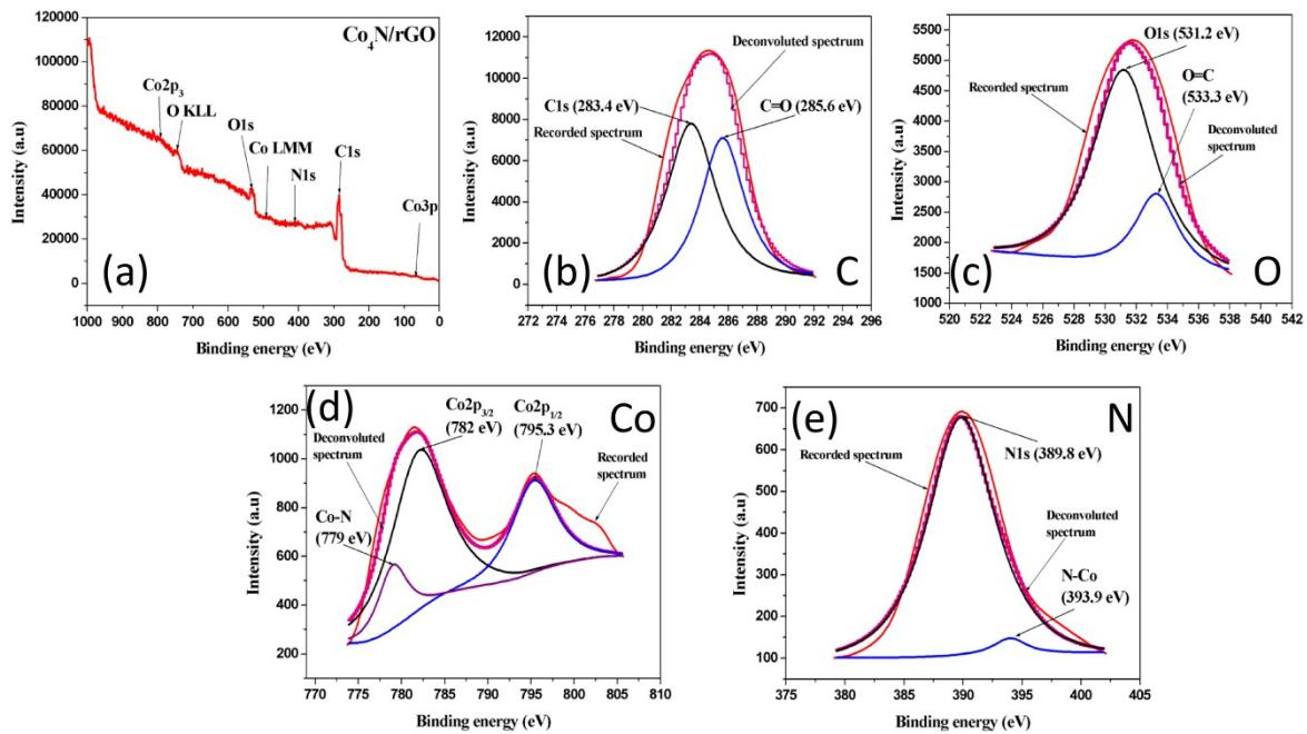
Figure S4. (a) XPS spectrum of  $\text{Co}_4\text{N}/\text{rGO}$ . High-resolution XPS spectra of (b) carbon, (c) oxygen, (d) cobalt and (e) nitrogen.
