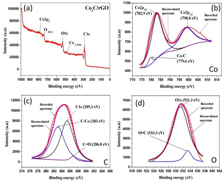
Figure S3. (a) XPS spectrum of  $\text{Co}_2\text{C}/\text{rGO}$ . High-resolution XPS spectra of (b) cobalt, (c) carbon and (d) oxygen.
