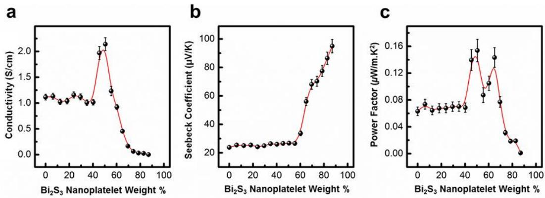
**Figure S9.** Dependence of (a) electrical conductivity, (b) Seebeck coefficient and (c) power factor on the weight percentage of bismuth sulfide nanoplatelets in the hybrid film with PEDOT:PSS. The red curve is a guide to the eye. Vertical error bars represent the variance of measurements over multiple samples. Horizontal error bars that represent the uncertainty in the weight percentage measurement are typically in the order of 5% and are not shown in the figure for clarity.
