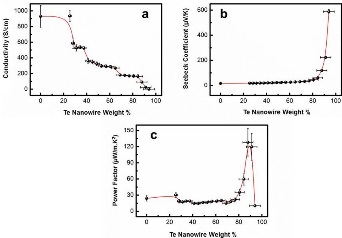
**Figure S11.** Dependence of (a) electrical conductivity, (b) Seebeck coefficient and (c) power factor on the weight percentage of tellurium nanowires in the hybrid film with PEDOT:PSS treated with formic acid. Vertical error bars represent the variance of measurements over multiple samples while horizontal error bars represent the uncertainty in the weight percentage measurement. The red curve is a guide to the eye.
