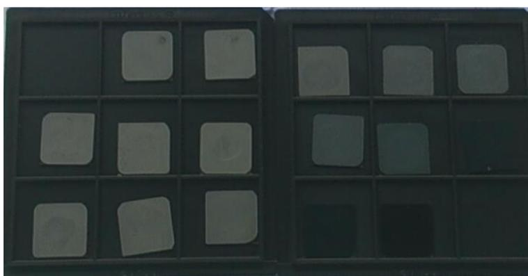
**Figure S7.** Smooth films cast from a series of dispersions of hybrid tellurium-PEDOT:PSS nanowires in water with varying amounts of PEDOT:PSS on 1cm X 1cm square glass substrates.
