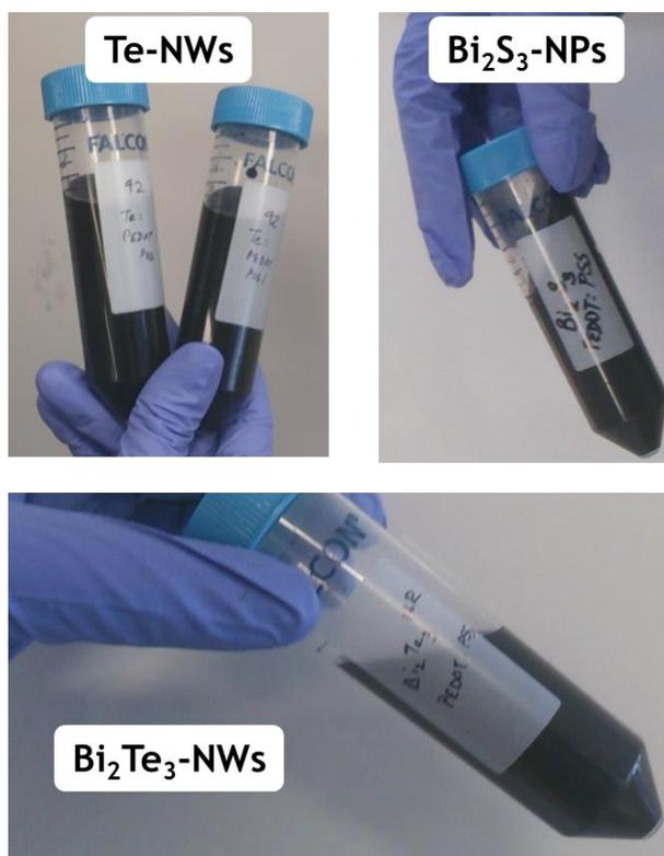
**Figure S6.** Stable dispersions of hybrid PEDOT:PSS-capped tellurium nanowires, bismuth sulfide nanoplatelets and bismuth telluride nanowires in water.
