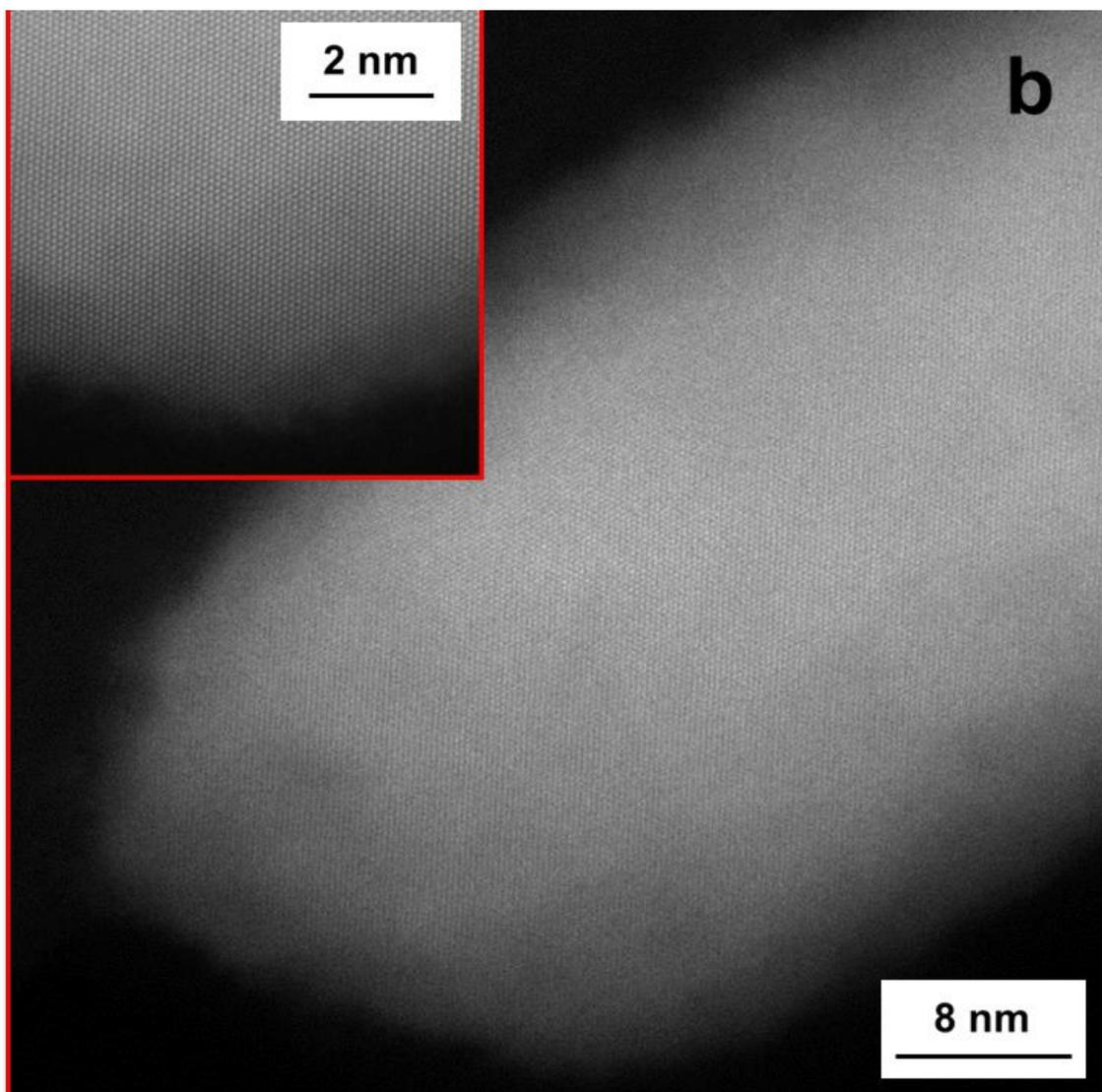
**Figure S3.** High resolution scanning transmission electron micrographs of (a) Te nanowires synthesized in-situ with PEDOT:PSS and (b) sulfur-capped Te nanowires synthesized without PEDOT:PSS. Insets show zoomed-in images of the respective nanostructures. While the nanowires that are synthesized ex-situ (without PEDOT:PSS during growth) are highly crystalline, the Te-PEDOT:PSS nanowires from an one-pot synthesis are polycrystalline.
