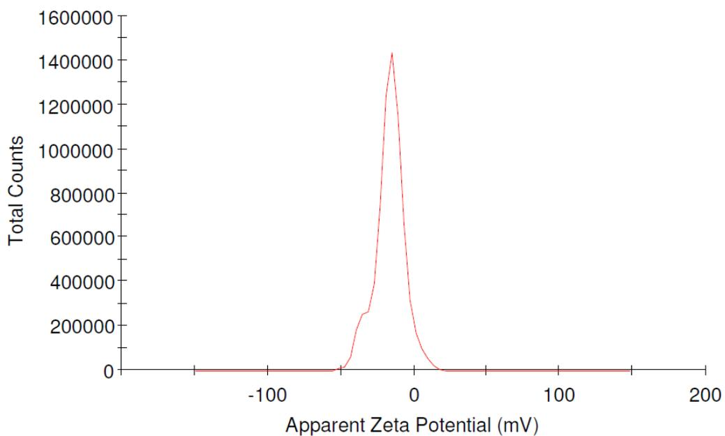
**Figure S2.** The averaged ( $n=72$ ) Zeta Potential and phase distribution for sulfur capped tellurium nanowires dispersed in water. Sample concentration was  $\sim 10$  microgram/mL. The sample was transferred to a zeta cell (Malvern Instruments) and measured at  $25$  °C. The zeta potential was  $-16.6 \pm 10.2$  mV ( $n=72$ ). A viscosity of  $0.8872$  cP, a dielectric constant of  $78.5$  and Henry function of  $1.5$  were used for the calculations.
