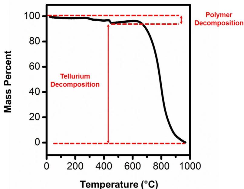
**Figure S4.** Thermogravimetric analyses (TGA) of the hybrid Te-PEDOT:PSS nanowires. The material was dried thoroughly before the TGA so there was no appreciable mass loss before 100 °C. There is a slight mass gain after the polymer has fully decomposed due to oxidation of the tellurium to tellurium dioxide.
