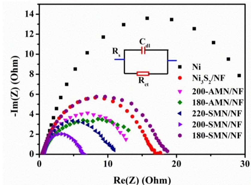
**Figure S11.** Nyquist plots of, 180-SMN/NF, 200-SMN/NF, 220-SMN/NF, 180-AMN/NF, 220-AMN/NF, Ni<sub>3</sub>S<sub>2</sub>/NF, and bare Ni foam electrodes recorded at an applied potential of -1.2 V with a frequency range of 10 kHz to 10 mHz in 1 m KOH
