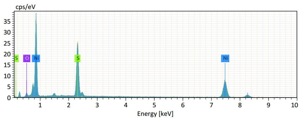
**Figure S6.** EDX spectrum of  $\text{Ni}_3\text{S}_2/\text{NF}$
