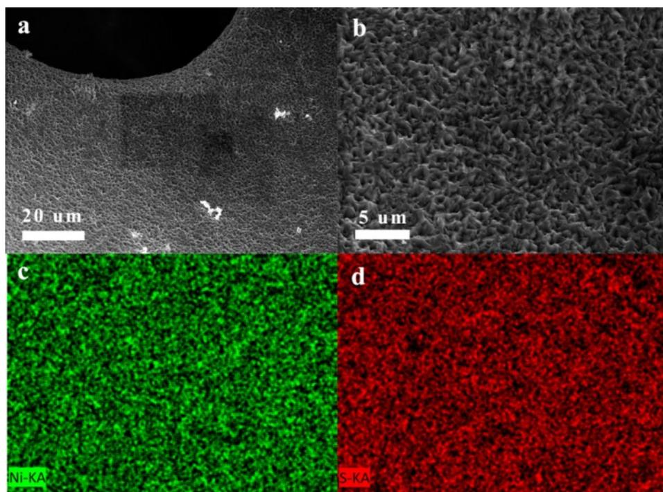
**Figure S5.** SEM images and EDX-mapping of  $\text{Ni}_3\text{S}_2/\text{NF}$
