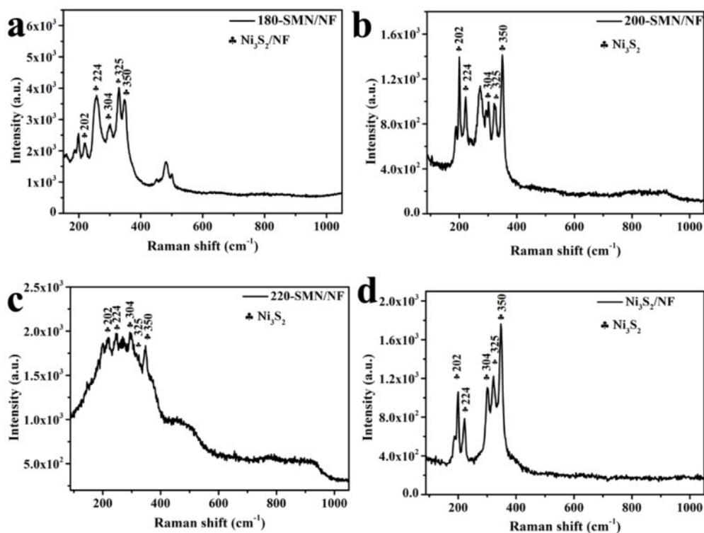
**Figure S4.** Raman spectrum of 180-SMN/NF (a), 200-SMN/NF (b), 220-SMN/NF (c), Ni<sub>3</sub>S<sub>2</sub>/NF (d)
