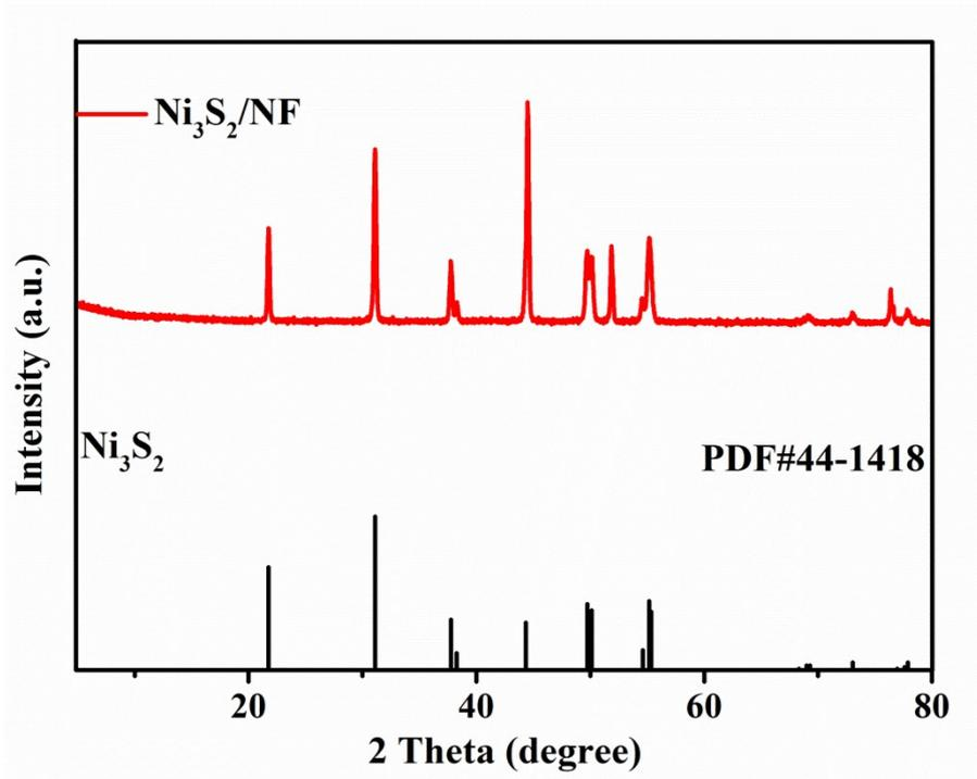
Figure S2. XRD patterns of  $\text{Ni}_3\text{S}_2/\text{NF}$
