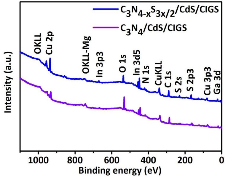
**Figure S5.** High resolution XPS spectrum of  $C_3N_4/CdS/CIGS$  and  $C_3N_{4-x}S_{3x/2}/CdS/CIGS$  photocathodes.
