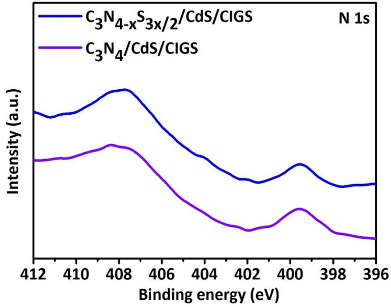
**Figure S4.** High resolution XPS spectra of N 1s in  $C_3N_4/CdS/CIGS$  and  $C_3N_{4-x}S_{3x/2}/CdS/CIGS$  samples.
