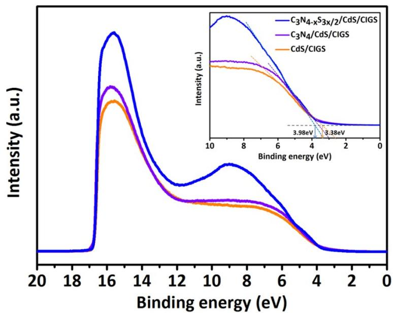
**Figure S12.** Ultraviolet Photoelectron Spectra of  $CdS/CIGS$ ,  $C_3N_4/CdS/CIGS$  and  $C_3N_{4-x}S_{3x/2}/CdS/CIGS$ .
