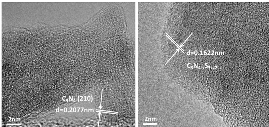
**Figure S3.** Typical TEM images of  $C_3N_4$  (a) and  $C_3N_{4-x}S_{3x/2}$  (b) particles.
