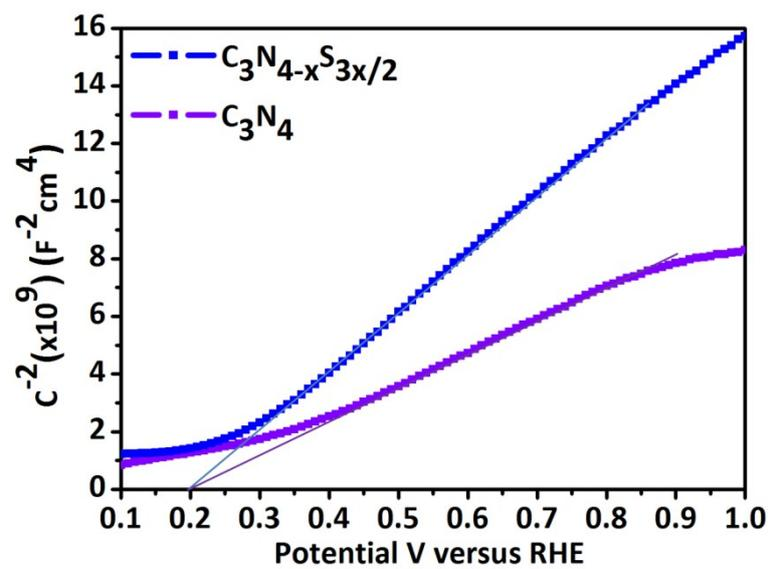
**Figure S8.** Mott-Schottky plots of  $\text{C}_3\text{N}_4$  and  $\text{C}_3\text{N}_{4-x}\text{S}_{3x/2}$  photocathodes. The ac amplitude is 10 mV and the frequency is 200 Hz.
