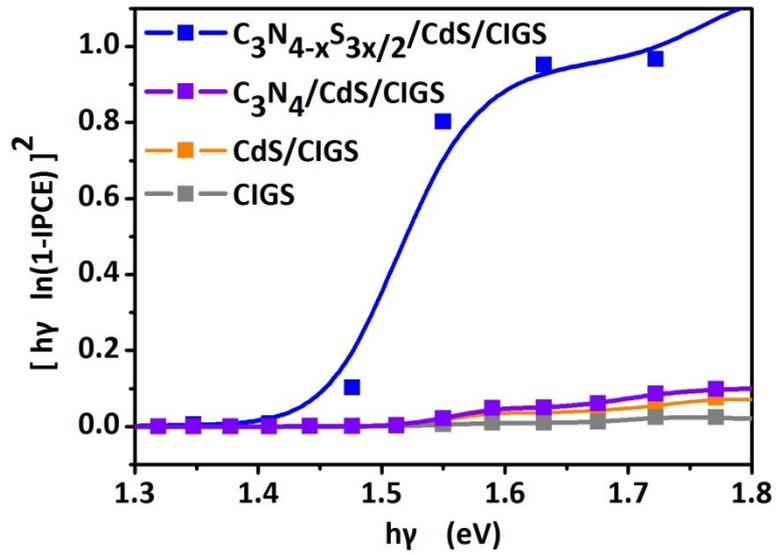
**Figure S11.**  $[hy \ln(1-IPCE)]^2$  vs. band gap (eV) plots of CIGS, CdS/CIGS,  $C_3N_4/CdS/CIGS$  and  $C_3N_{4-x}S_{3x/2}/CdS/CIGS$ .
