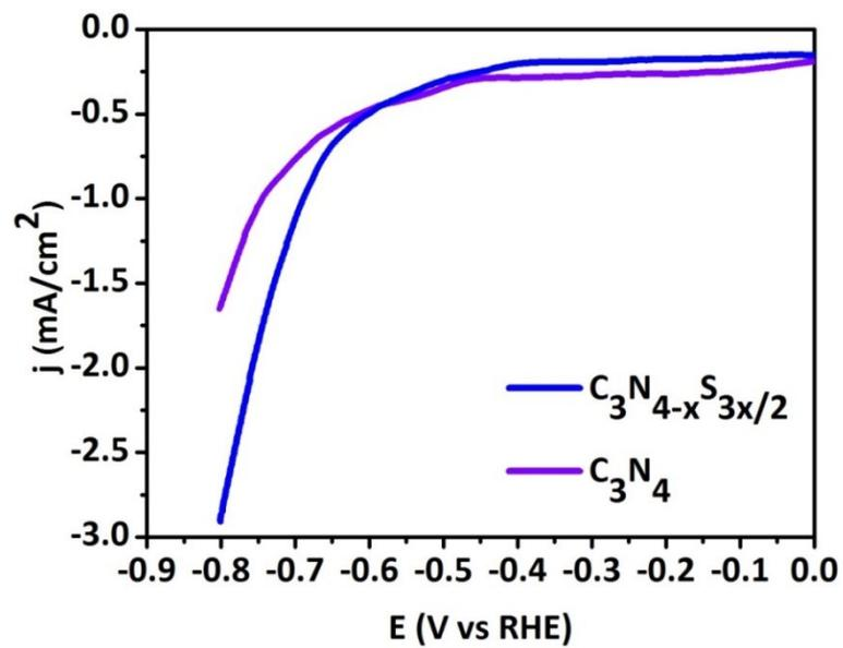
**Figure S6.** The Steady-state current density as a function of applied voltage during HER at 1 M  $K_2HPO_4/KH_2PO_4$  solution (pH=7) over  $C_3N_{4-x}S_{3x/2}$  and  $C_3N_4$ .
