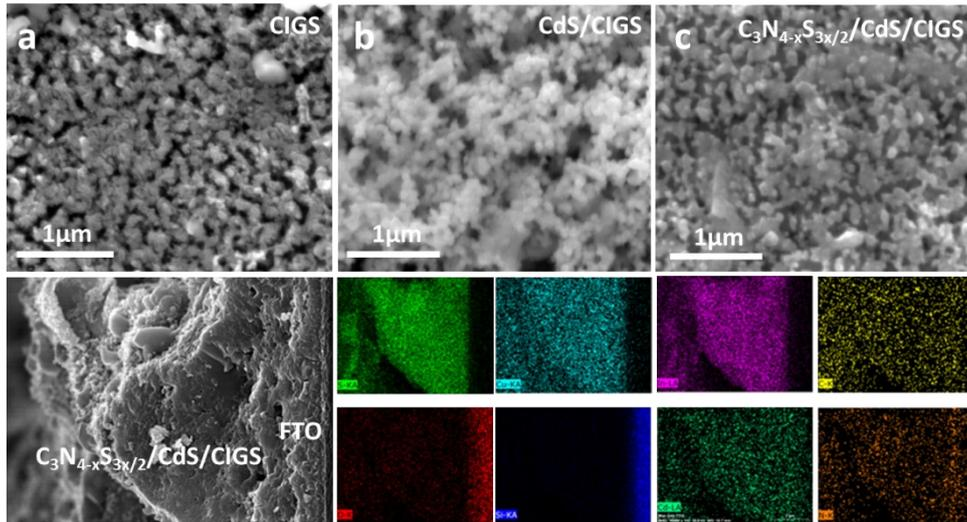
**Figure S1.** a-c) SEM images of (a) CIGS, (b) CdS/CIGS, and (c) C<sub>3</sub>N<sub>4-x</sub>S<sub>3x/2</sub>/CdS/CIGS. d) EDS measurements of C<sub>3</sub>N<sub>4-x</sub>S<sub>3x/2</sub>/CdS/CIGS.
