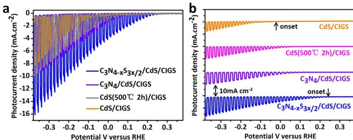
**Figure S7.** The Current–potential plots for  $\text{CdS}/\text{CIGS}$ ,  $\text{C}_3\text{N}_4/\text{CdS}/\text{CIGS}$  and  $\text{C}_3\text{N}_{4-x}\text{S}_{3x/2}/\text{CdS}/\text{CIGS}$  photocathodes all the  $\text{CdS}/\text{CIGS}$  substrate using a chemical vapor deposition (CVD) route in a 1 M  $\text{K}_2\text{HPO}_4/\text{KH}_2\text{PO}_4$  solution ( $\text{pH}=7$ ) irradiated with chopped AM 1.5G illumination.
