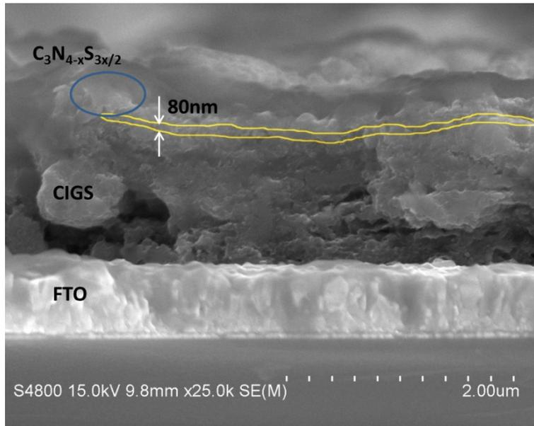
**Figure S2.** Cross-section SEM image of  $C_3N_{4-x}S_{3x/2}/CdS/CIGS$  electrode.
