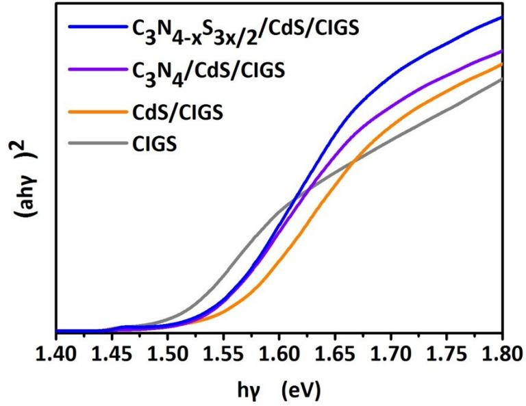
**Figure S10.** Absorbance spectra in the band edge region for samples CIGS, CdS/CIGS,  $C_3N_4/CdS/CIGS$  and  $C_3N_{4-x}S_{3x/2}/CdS/CIGS$  with an extrapolation of the spectra in order to determine the band gap values.
