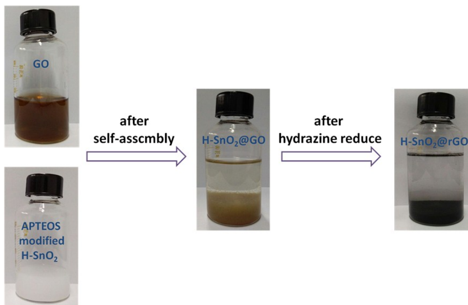
Figure S3. Photographs of the assembly process of APTEOS modified H-SnO 2 and graphene oxide in aqueous solutions at pH 2.
