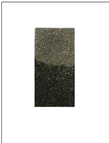
Fig. S5 Optical photograph of the deposited NG/NiSe 2 /NF electrode on the surface of N-doped graphene encapsulated Ni foam.
