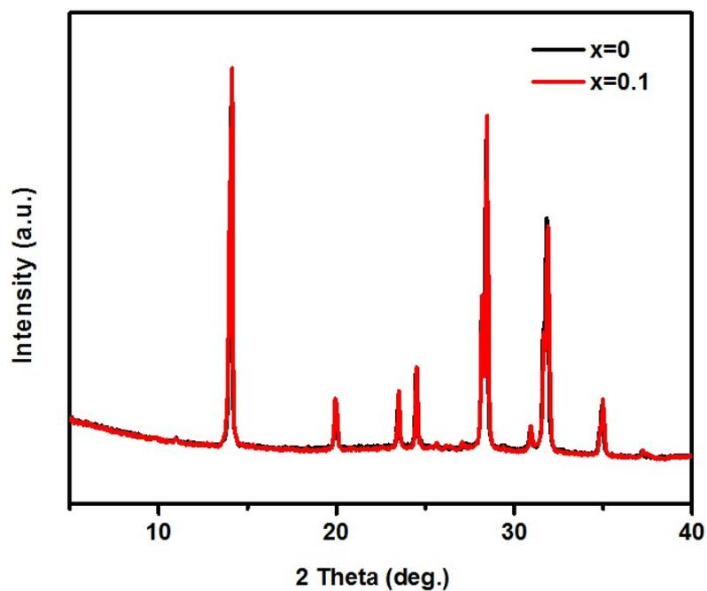
Figure S11. XRD patterns of  $\text{Cs}_x\text{MA}_{1-x}\text{PbI}_3$  ( $x=0, 0.1$ ) powder.
