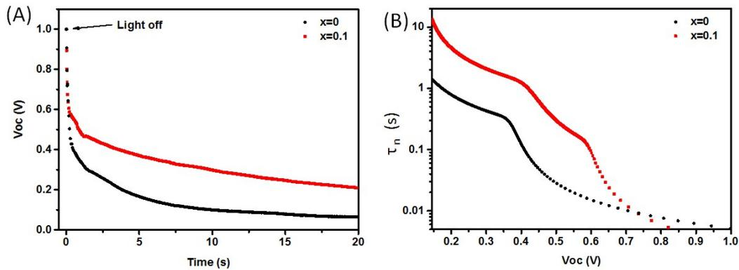
Figure S10. (A)  $V_{oc}$  decay curves and (B) Electron lifetime  $\tau_n$  extracted from  $V_{oc}(t)$  as a function of  $V_{oc}$  of  $\text{Cs}_x\text{MA}_{1-x}\text{PbI}_3$  ( $x=0, 0.1$ ) solar cells.
