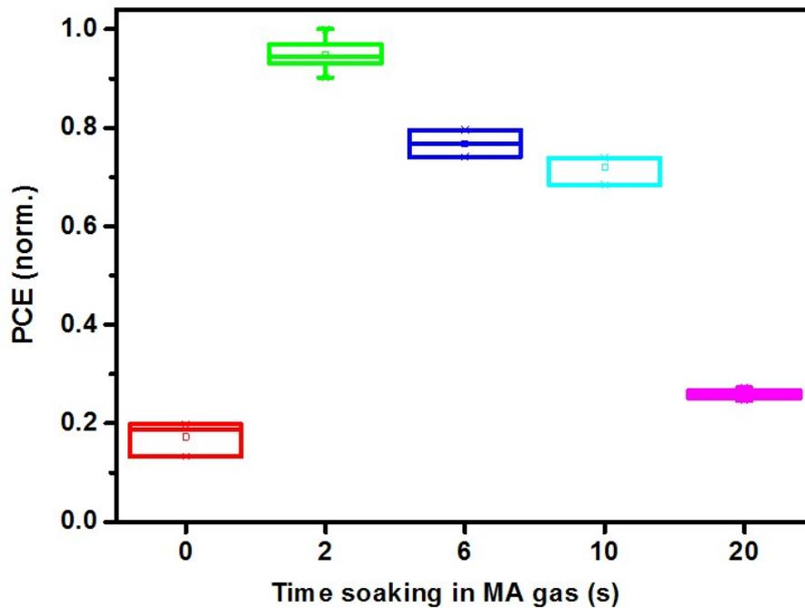
Figure S6. The efficiency distribution of the  $\text{Cs}_{0.1}\text{MA}_{0.9}\text{PbI}_3$  perovskite solar cells fabricated by treating the perovskite films in MA gas from 0 s to 20 s.
