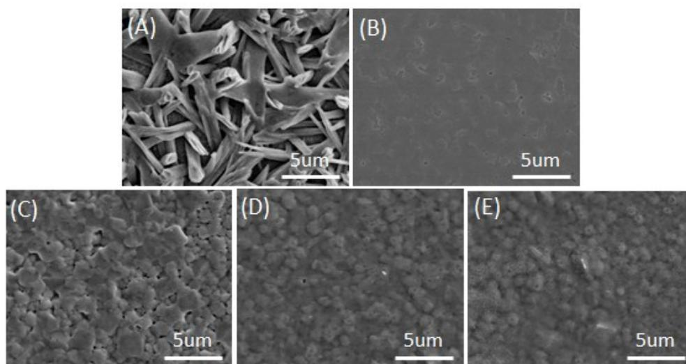
Figure S4. SEM images of  $\text{Cs}_{0.1}\text{MA}_{0.9}\text{PbI}_3$  perovskite films with different soaking time in MA gas: 0 s (A), 2 s (B), 6 s (C), 10 s (D), 20 s (E).
