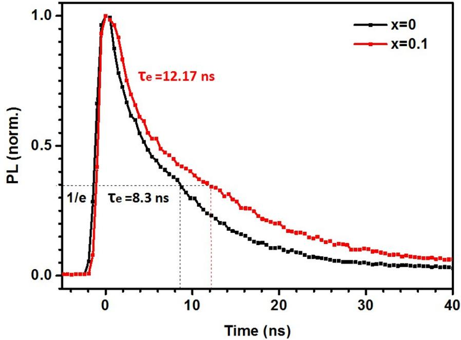
Figure S9. Time-resolved PL measurements, with lifetimes  $\tau_e$  quoted as the time taken to reach  $1/e$  of the initial intensity for  $\text{Cs}_x\text{MA}_{1-x}\text{PbI}_3$  ( $x=0, 0.1$ ) solar cells.
