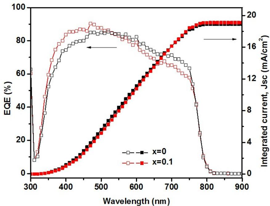
Figure S8. External quantum efficiency (EQE) and integrated current ( $J_{sc}$ ) of  $\text{Cs}_x\text{MA}_{1-x}\text{PbI}_3$  ( $x=0, 0.1$ ) solar cells.
