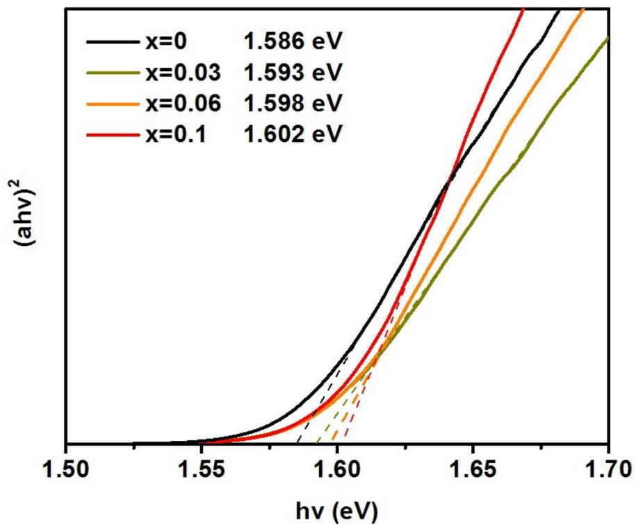
Figure S2. UV-Vis absorbance of Cs<sub>x</sub>MA<sub>1-x</sub>PbI<sub>3</sub> perovskite films, where x is varied from 0 to 0.1.
