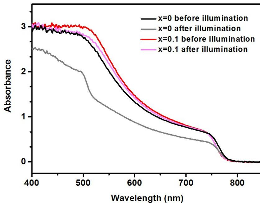
Figure S12. UV-Vis absorbance spectra of  $\text{Cs}_x\text{MA}_{1-x}\text{PbI}_3$  ( $x=0, 0.1$ ) perovskite films before and after one sun illumination for 3 h without any protection under a humidity of 40%.
