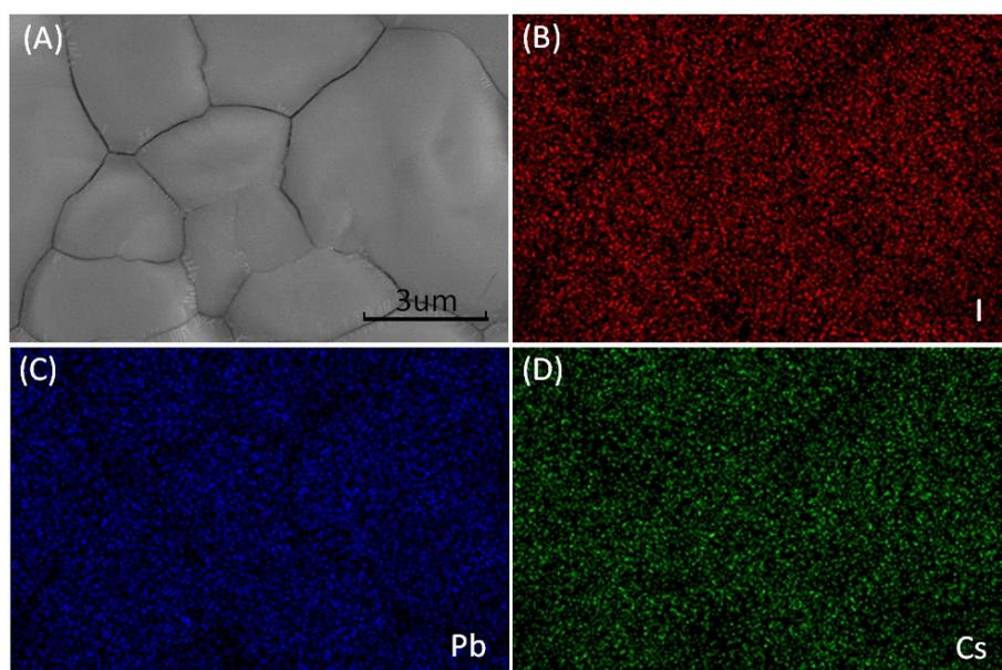
Figure S3. Top surface SEM image of  $\text{Cs}_{0.1}\text{MA}_{0.9}\text{PbI}_3$  film (A) and its corresponding EDS maps for iodine (B), lead (C), and cesium (D).
