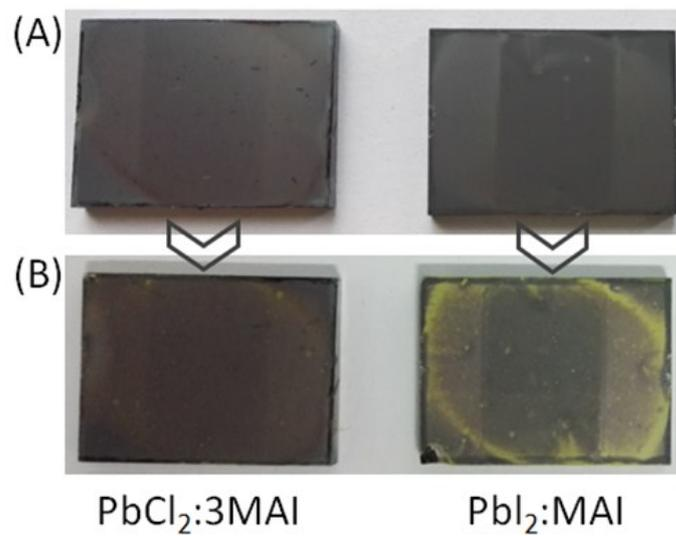
Figure S1. (A) Fresh MAPbI<sub>3</sub> films prepared from the PbCl<sub>2</sub>: 3MAI and PbI<sub>2</sub>: MAI recipes. (B) The MAPbI<sub>3</sub> films exposed in air under a humidity of 40% for 2 days.
