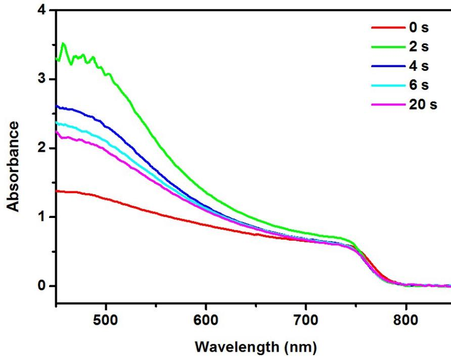
Figure S5. UV-Vis absorbance spectra of  $\text{Cs}_{0.1}\text{MA}_{0.9}\text{PbI}_3$  perovskite films with different treating time in MA gas from 0 s to 20 s.
