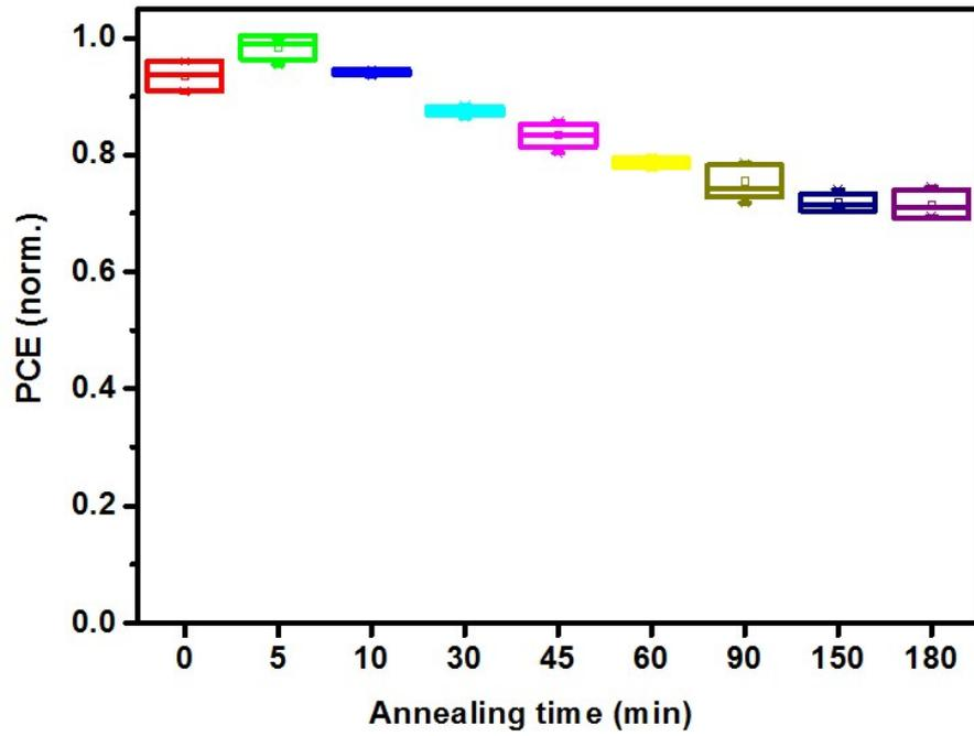
Figure S7. The efficiency distribution of the  $\text{Cs}_{0.1}\text{MA}_{0.9}\text{PbI}_3$  perovskite solar cells fabricated with different annealing time at  $100^\circ\text{C}$  from 0 min to 180 min.
