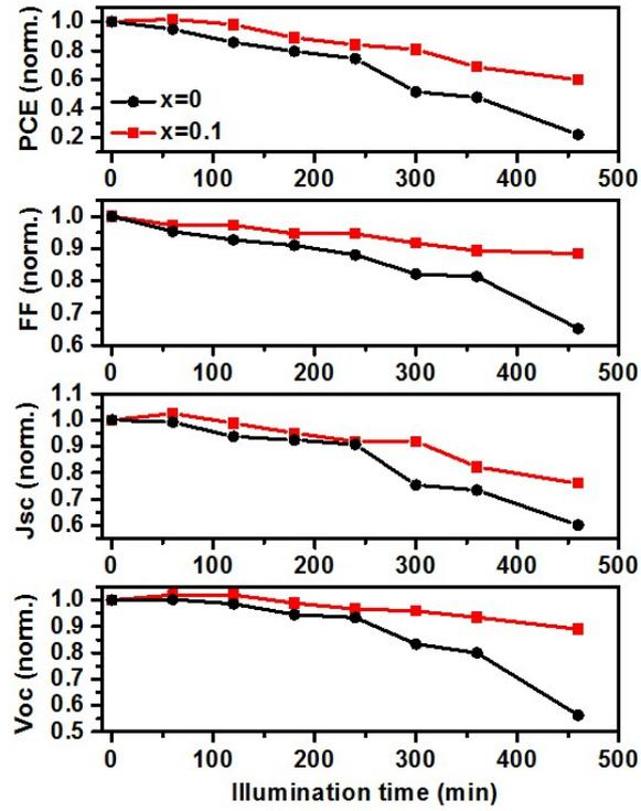
Figure S13. Comparison of the stability of  $\text{Cs}_x\text{MA}_{1-x}\text{PbI}_3$  ( $x=0, 0.1$ ) perovskite solar cells.
