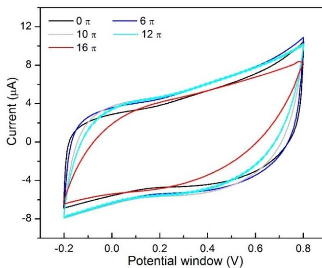
**Fig. S7** CV curves of a SACNT-film based supercapacitor at different torsion levels.
