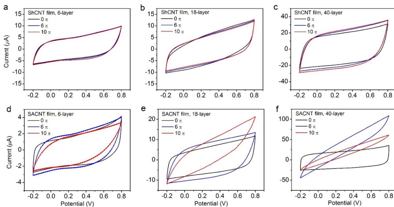
**Fig. S8** CV curves of the supercapacitors with ShCNT-film electrodes (a-c) and SACNT-film electrodes (d-f) at various torsion levels.
