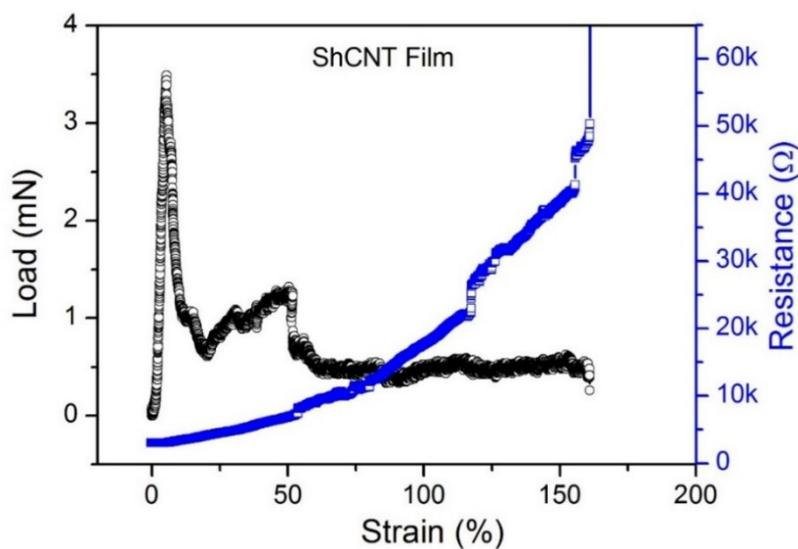
**Fig. S3** The tensile and electrical properties of a single-layer ShCNT film. Dimensions: length  $\times$  width  $\times$  thickness = 6 mm  $\times$  1 mm  $\times$  1  $\mu$ m).
