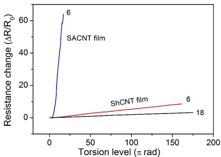
**Fig. S4** Resistance change of the conductor based on the ShCNT film (6- and 18- layers) and the SACNT film (6-layer) during torsional loading.
