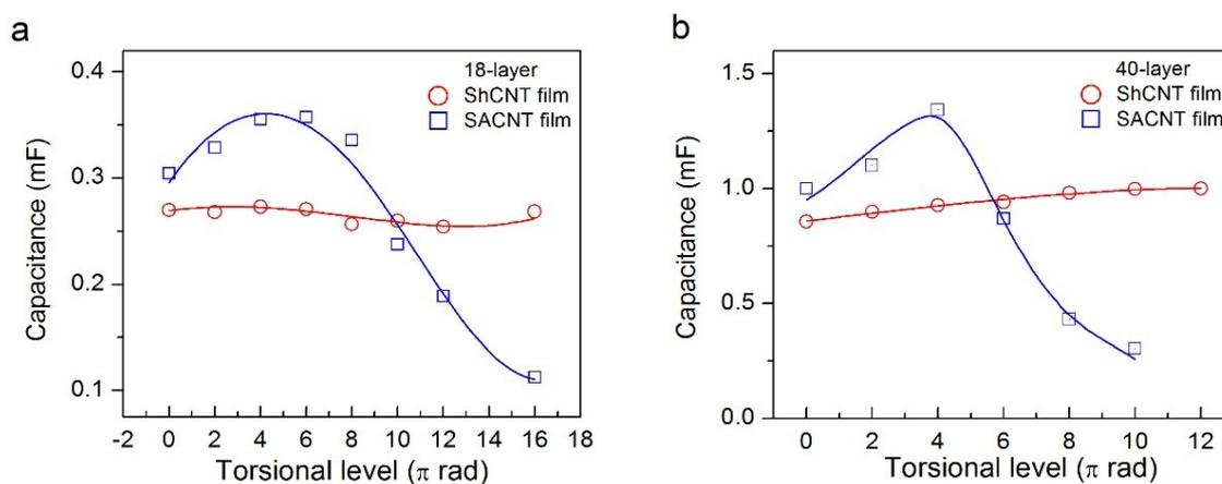
**Fig. S9** The capacitances comparison between ShCNT-film based supercapacitors and SACNT-film based supercapacitors made of 18 layers of CNTs (a) and 40 layers of CNTs (b).
