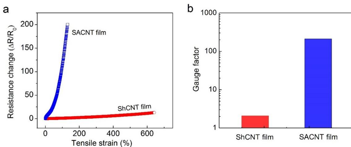
**Fig. S5** (a) Resistance change of conductors based on 6-layer ShCNT film and SACNT film during tensile deformation and, (b) the corresponding gauge factors (after the tensile strain >50%).
