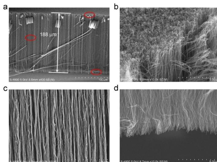
**Fig. S1** SEM images of the CNT array: Views from (a) the side, (b) the top, (c) the middle and (d) the bottom. The majority of the CNTs have a length of 188  $\mu\text{m}$ , the same as the height of the array. CNT fibrils intertwined between the vertical CNT bundles can be seen in the top, middle and bottom parts of the array.
