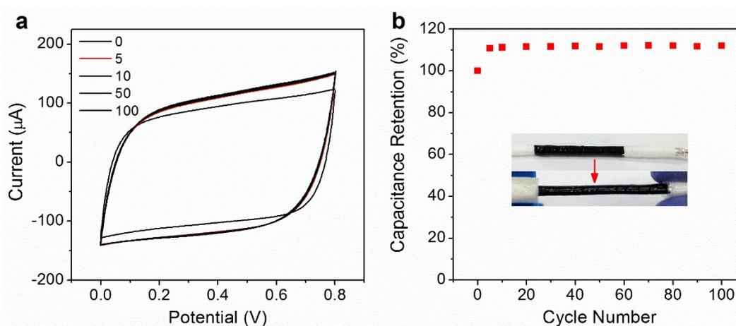
**Fig. S10** The capacitive performance of the torsionable supercapacitor (150 layer) under repeated stretching (50% strain) and release cycles. (a) CV curves at various cycles. (b) Capacitance retention calculated from the CV curves. The inset shows a supercapacitor being stretched.
