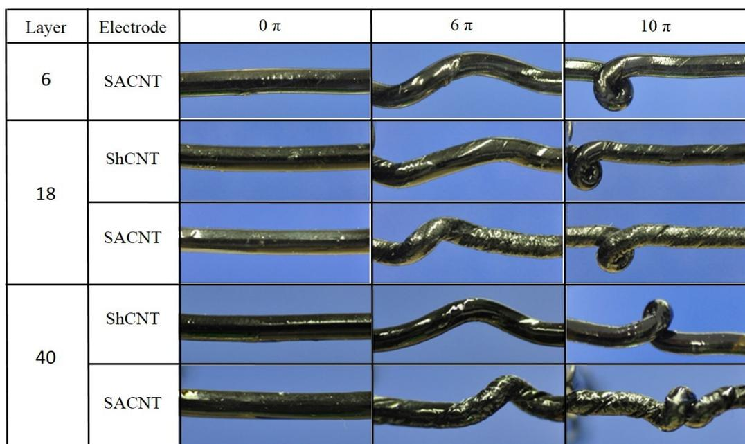
**Fig. S6** Digital photos showing the supercapacitors based on 6-, 18- and 40-layer ShCNT film and SACNT film electrodes subjected to different torsion levels.
