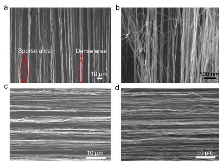
**Fig. S2** (a) An SEM image showing the sparse and dense areas of CNT bundles in a single layer ShCNT film and (b) A magnification of the dense area. (c,d) SEM images of 2- and 4-layer ShCNT films.
