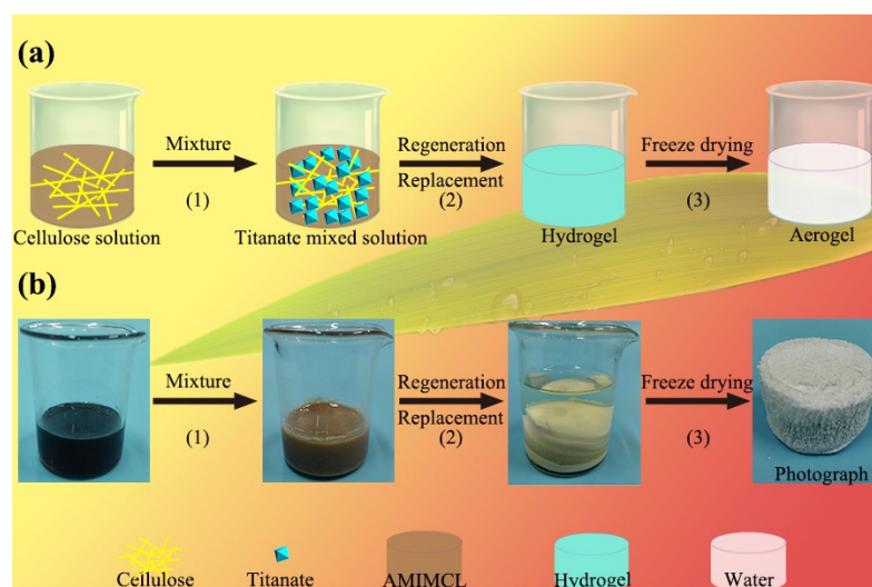
Figure S1. The schematic for the synthetic steps. (1) Titanate powder is dispersed into cellulose solution to generate a uniform suspension via vigorous stirring. (2) The composite hydrogel are gotten after dipping the freezing mixture in solidification liquid. (3) 3-D network titanate aerogel is obtained after further freeze-drying.
