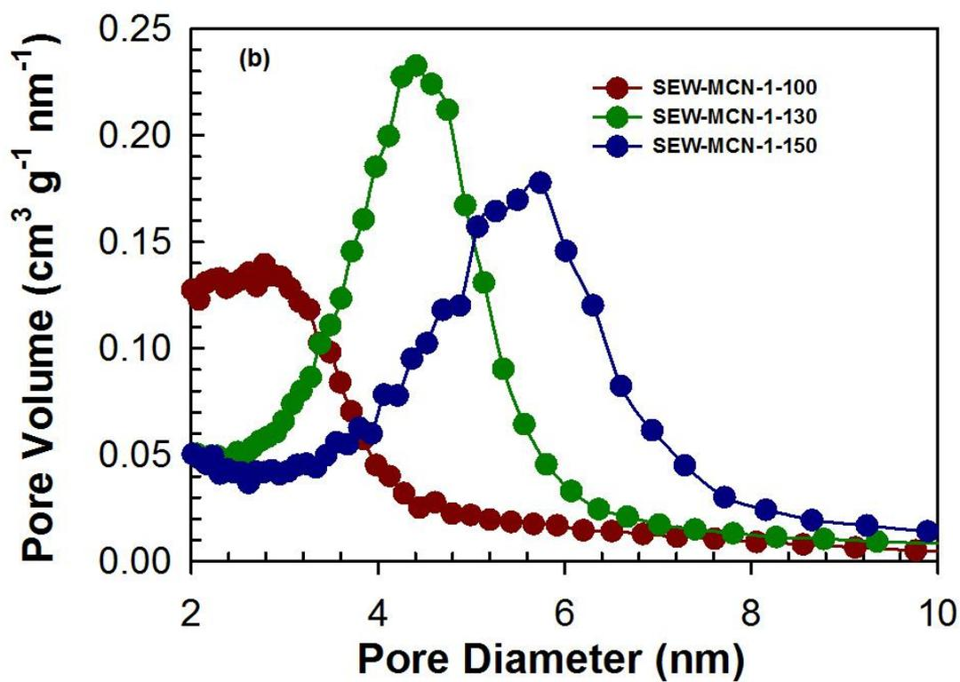
**Figure 15.** Pore size distribution plot obtained from the adsorption branch of nitrogen adsorption isotherm: (a) SEW-SBA-15-T and (b) SEW-MCN-1-T.
