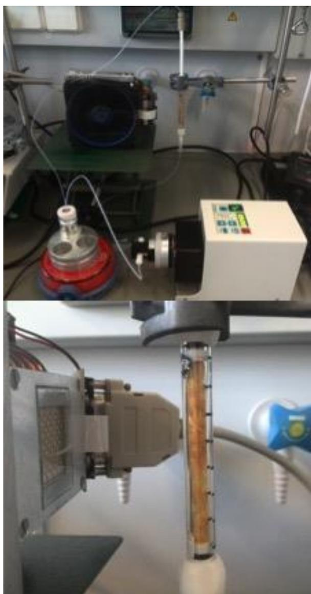
**Figure S5.** Setup of the fix-bed photoreactor in the continuous flow system.
