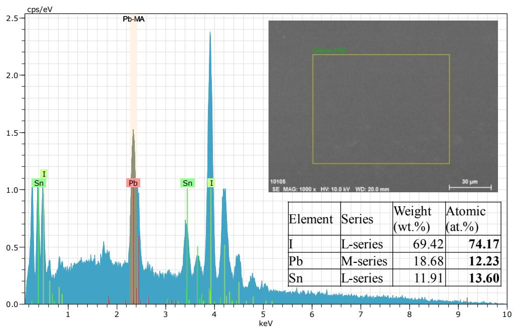
Figure S5. EDX analysis of  $\text{FASn}_{0.5}\text{Pb}_{0.5}\text{I}_3$  perovskite film on glass substrate.
