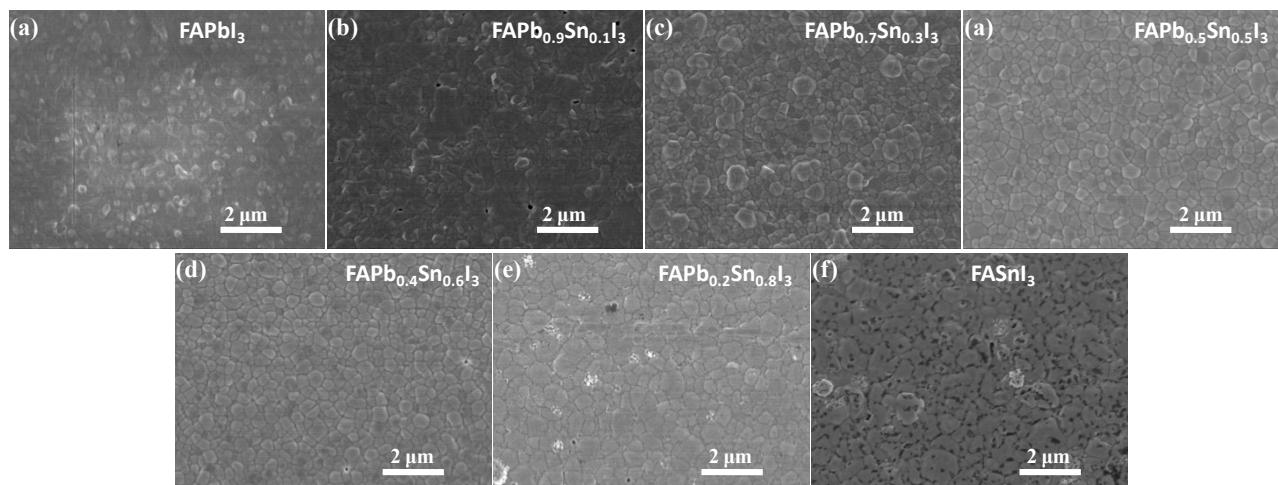
Figure S2. Low magnification SEM images of  $\text{FAPb}_{1-x}\text{Sn}_x\text{I}_3$  films on ITO-coated substrates
