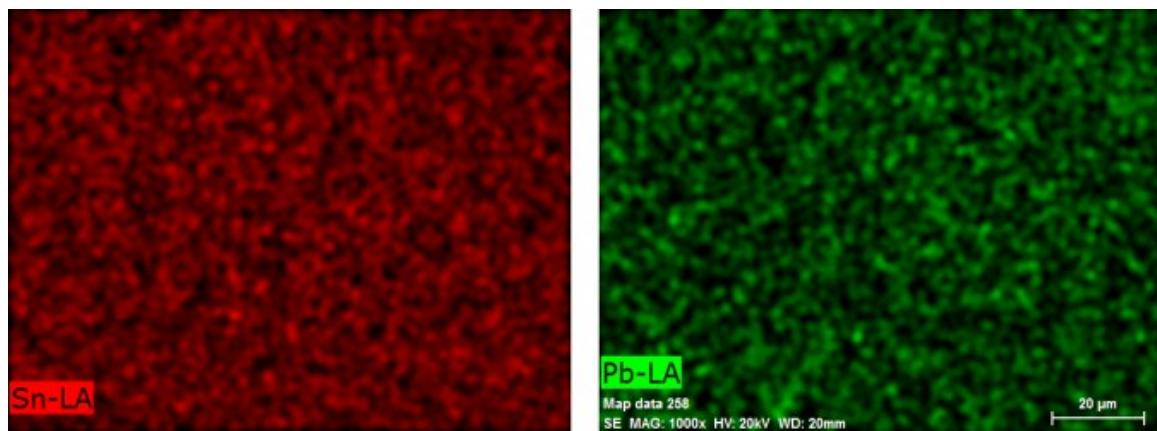
Figure S6. Elemental mapping images of  $\text{FASn}_{0.5}\text{Pb}_{0.5}\text{I}_3$  perovskite film.
