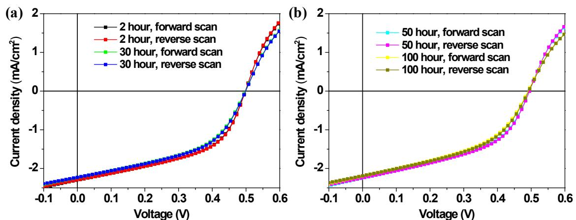
Figure S8. J-V curves of the perovskite solar cell measured under LED array light for different storage times.
