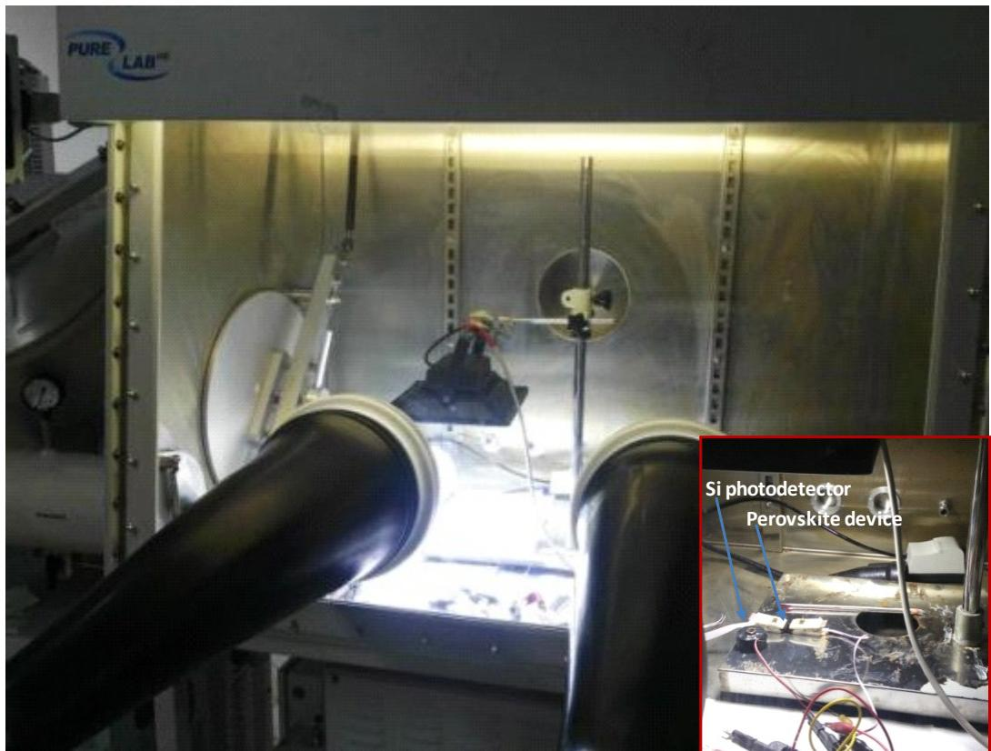
Figure S7. Stability measurement for perovskite solar cell.
