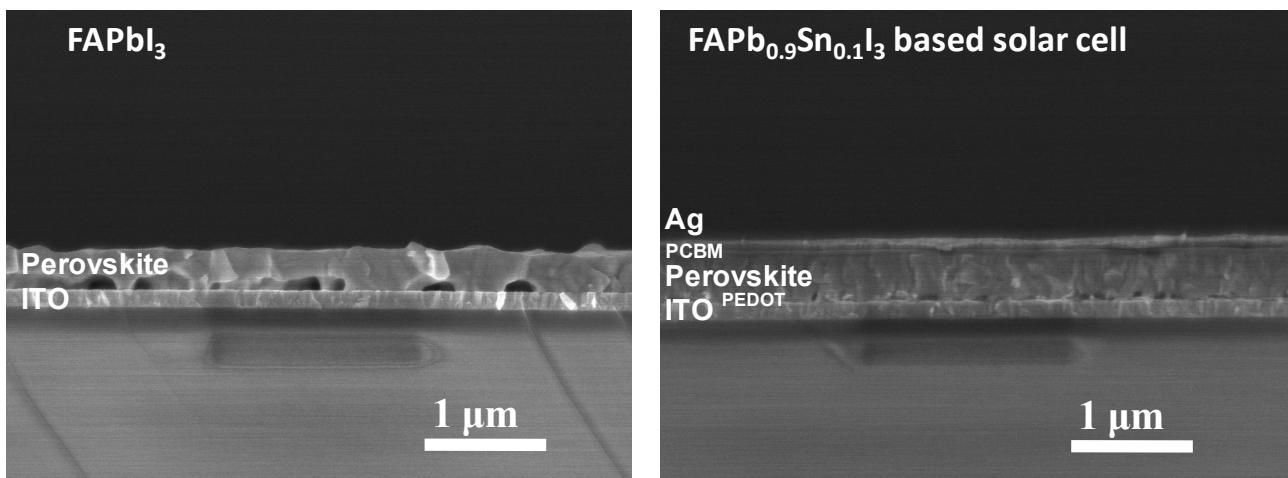
Figure S4. Cross-section Scanning Electron Micrograph (SEM) images of perovskite films
