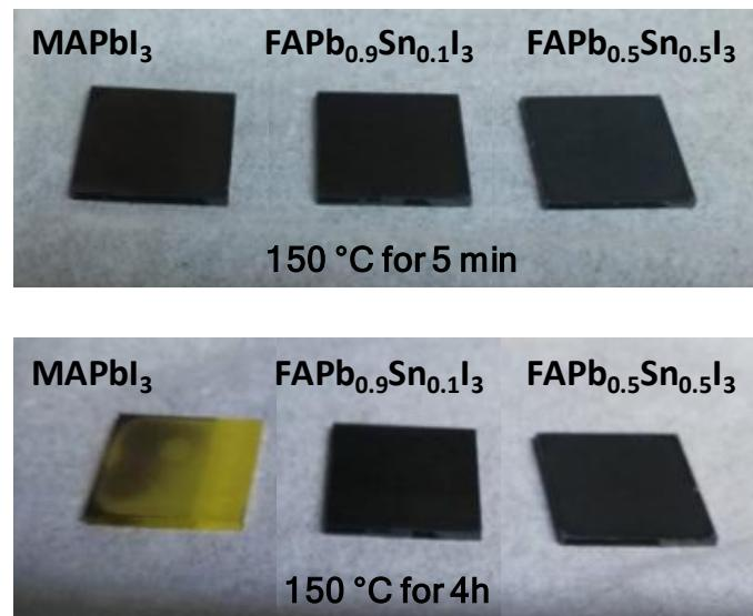
Figure S1. Images of  $\text{MAPbI}_3$ ,  $\text{FAPb}_{0.9}\text{Sn}_{0.1}\text{I}_3$  and  $\text{FAPb}_{0.5}\text{Sn}_{0.5}\text{I}_3$  films annealed under different conditions.
