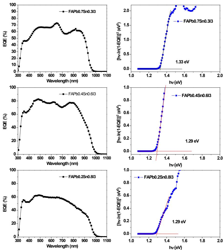
Figure S3. External quantum efficiency (EQE) of FAPb<sub>1-x</sub>Sn<sub>x</sub>I<sub>3</sub> perovskite solar cells with x = 0.3, 0.6 and 0.8.
