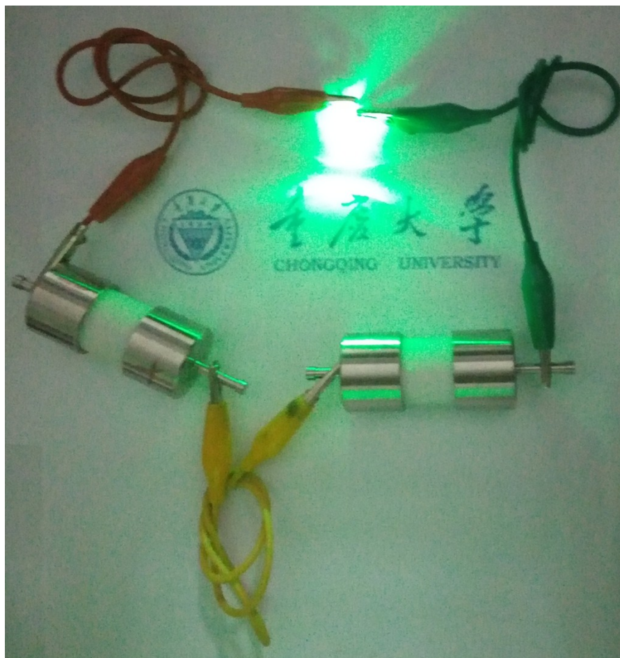
Fig. S3. Digital image of a green light-emitting diode (LED) lighted by the as-prepared ASC device.
