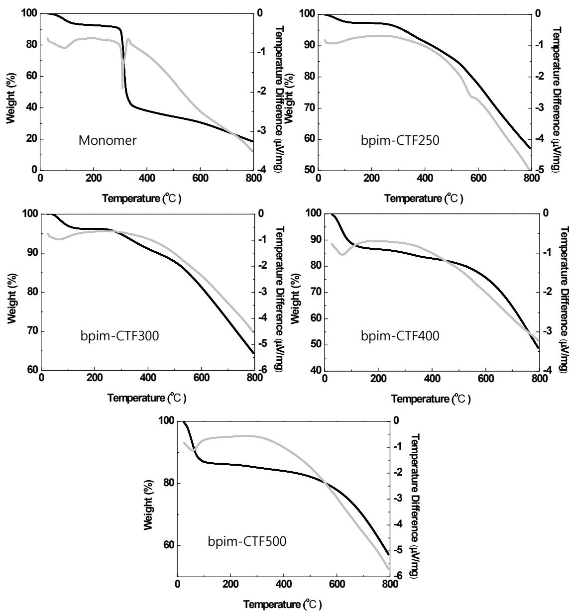
**Figure S4.** TGA measurements of bpim-CTFs and monomer
