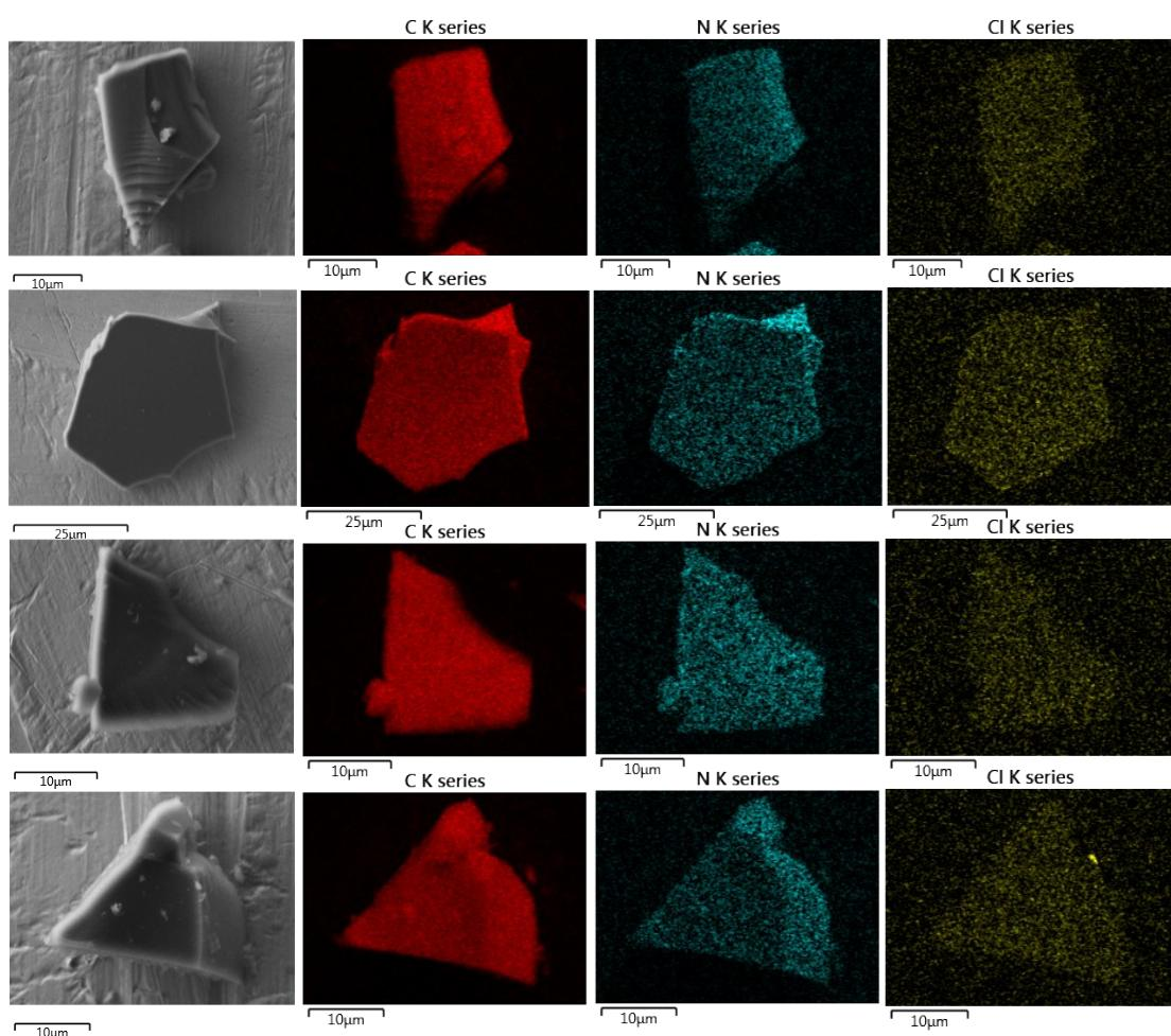
**Figure S2.** SEM & EDS mapping of bpim-CTFs
