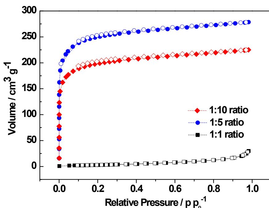
**Figure S1.** Nitrogen sorption isotherms of bpim-CTF synthesized with different  $\text{ZnCl}_2$  equivalent at 77 K
