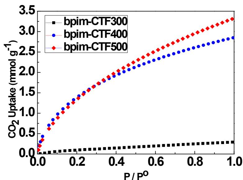
**Figure S5.** Carbon dioxide adsorption isotherms of bpim-CTFs at 288 K
