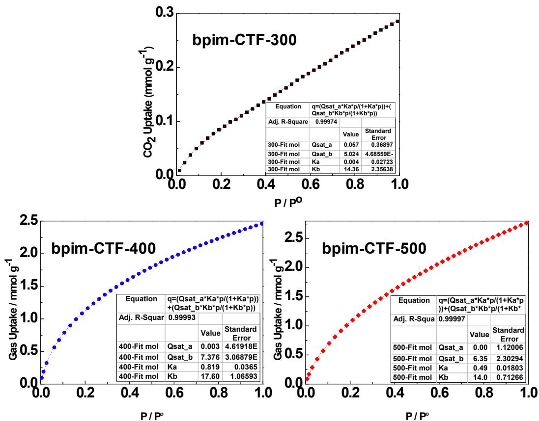
**Figure S8.** IAST plots of bpim-CTF-300 (top), 400 (bottom left), and 500 (bottom right) calculated from the carbon dioxide isotherms measured at 298 K.
