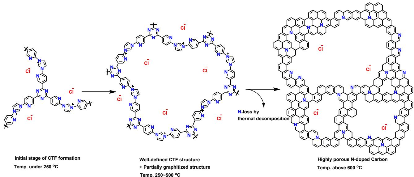
**Figure S13.** Proposed schematic representation for the gradual transformation of bpim-CTFs to N-doped porous carbons derived by thermal decomposition\*(concept for N-doped porous carbon was referred to ref 122)
