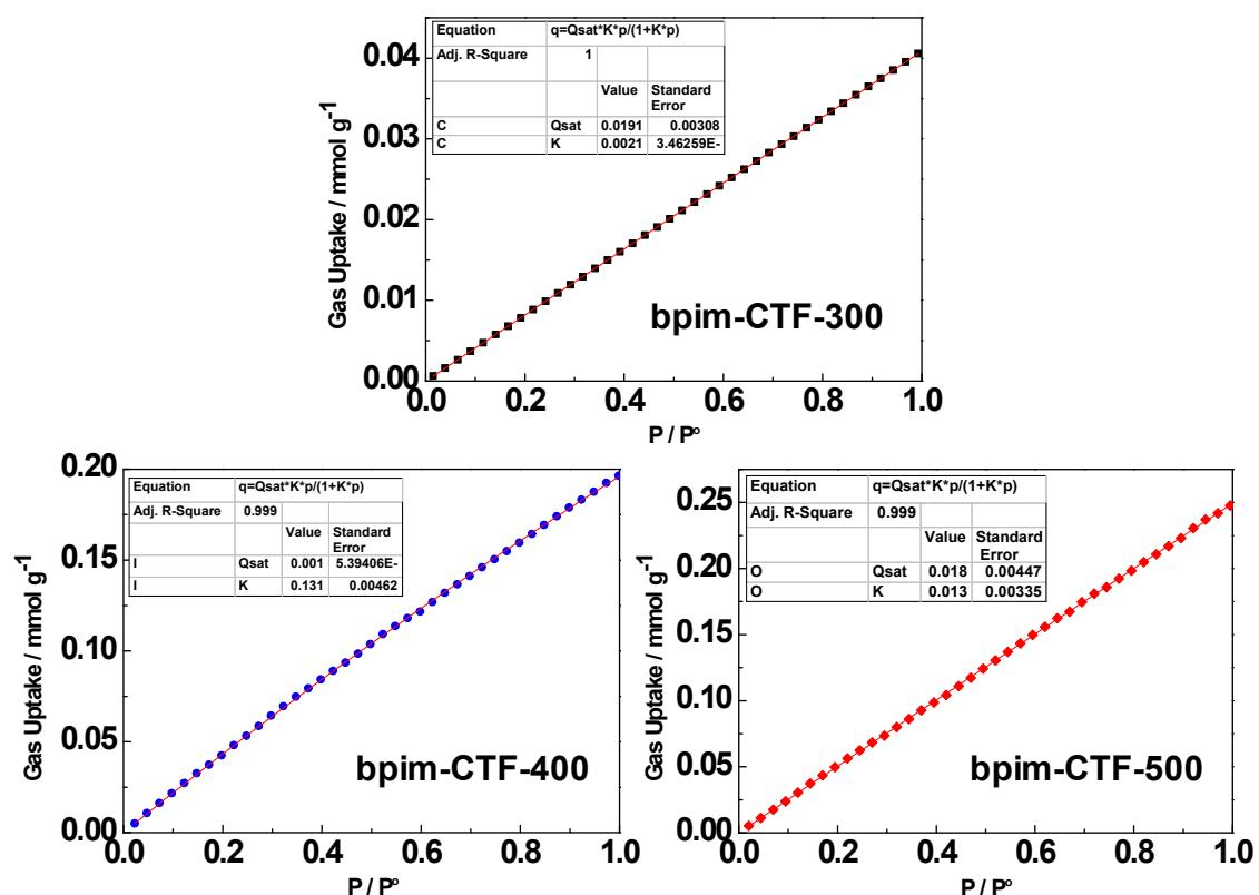
**Figure S9.** IAST plots of bpim-CTF-300 (top), 400 (bottom left), and 500 (bottom right) calculated from the nitrogen isotherms measured at 298 K.
