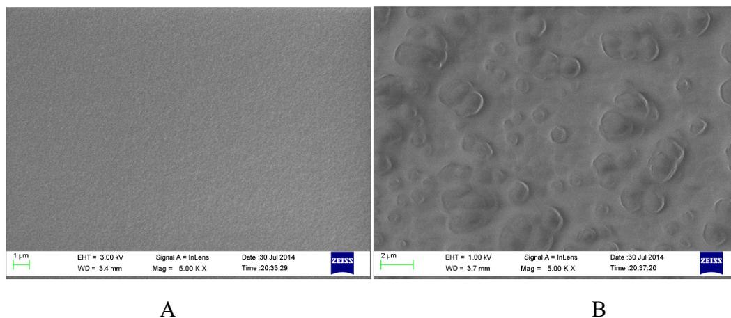
SEM images obtained to analyze the membrane structure of PBCA (A) and P-LKJ11 (B) at 5000 $\times$  magnification. The adhesives were uniformly smeared onto a support and polymerized to form the membrane. After spraying with gold, the analyses were performed using a JSM-5310 scanning microscope from Jeol.
