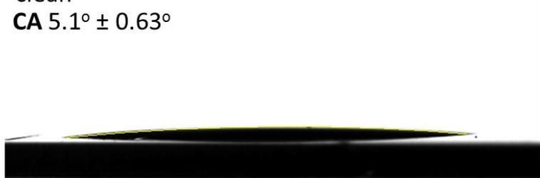
Figure S2: CA-images on SiNWs as synthesized (20 min MACE) and after overnight cleaning with nitric acid.
