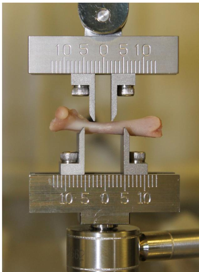
Supplementary Figure 2. Photograph of the 4-point mechanical testing setup. The image demonstrates the arrangement of the contact points. The mechanical driver is attached to the upper assembly and the force transducer is visible supporting the lower assembly.
