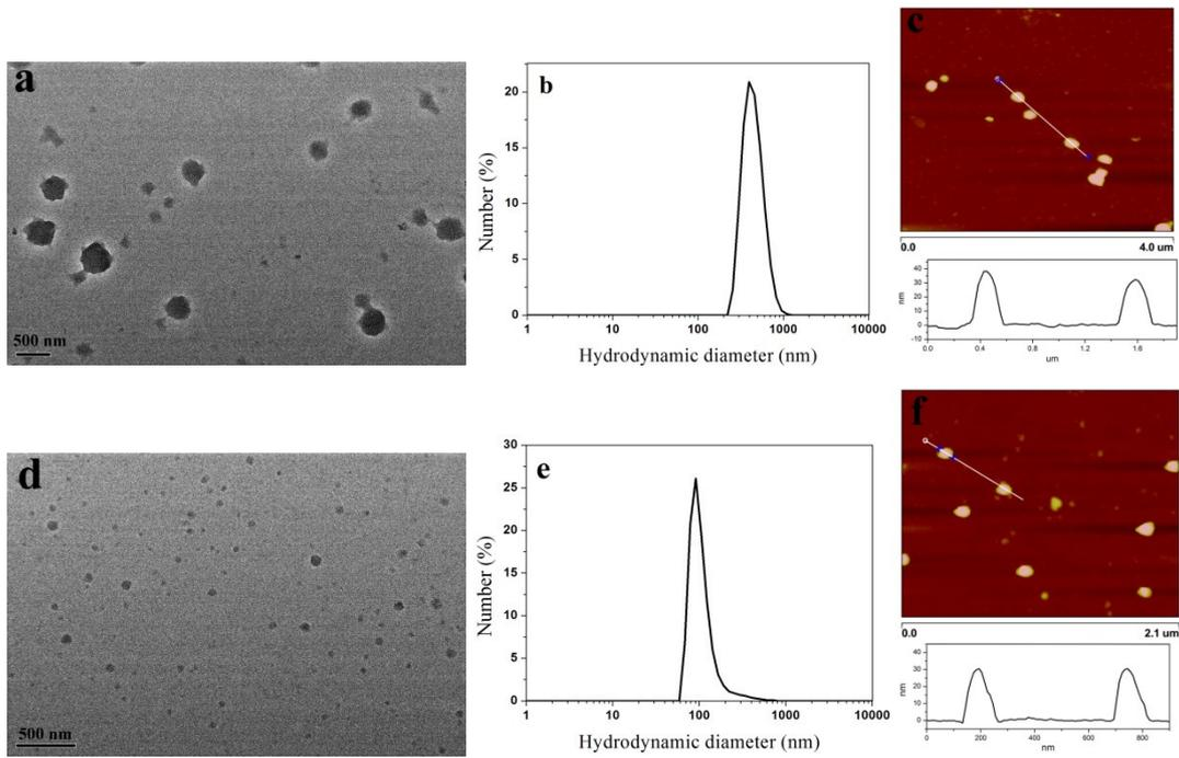
**Fig. S6** TEM image (a), DLS curve (b) and AFM image (c) of NP-1; TEM image (d), DLS curve (e) and AFM image (f) of NP-3.
