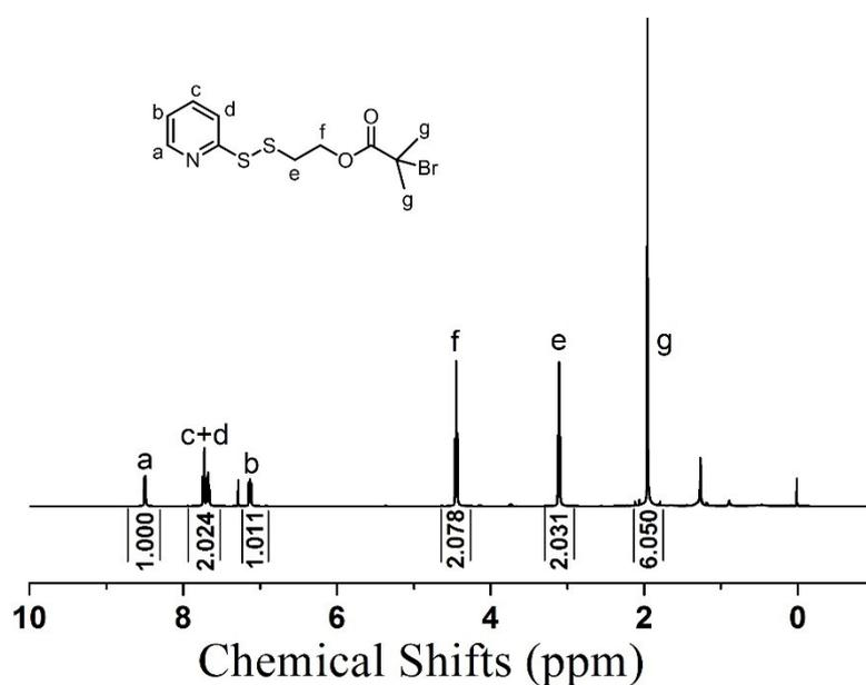
**Fig. S2** <sup>1</sup>H NMR spectrum of 2-(2-pyridinyldithio)ethyl 2-bromo-2-methylpropionate in CDCl<sub>3</sub>.
