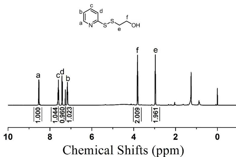
**Fig. S1** <sup>1</sup>H NMR spectrum of hydroxyethyl-mercaptopyridine in CDCl<sub>3</sub>.
