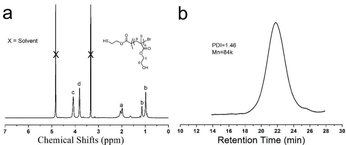
**Fig. S5**  $^1\text{H-NMR}$  spectrum (a) and GPC trace (b) of PHEMA after cleavage of disulfide bonds between BSA and PHEMA particles prepared in the absence of cross-linker.
