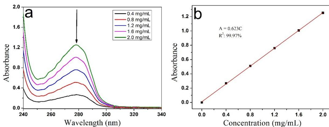
**Fig. S4** (a) UV-vis spectra of BSA at different concentrations in water. (b) Calibration curve for BSA determined by plotting the UV-vis absorbance at 278 nm against concentration.
