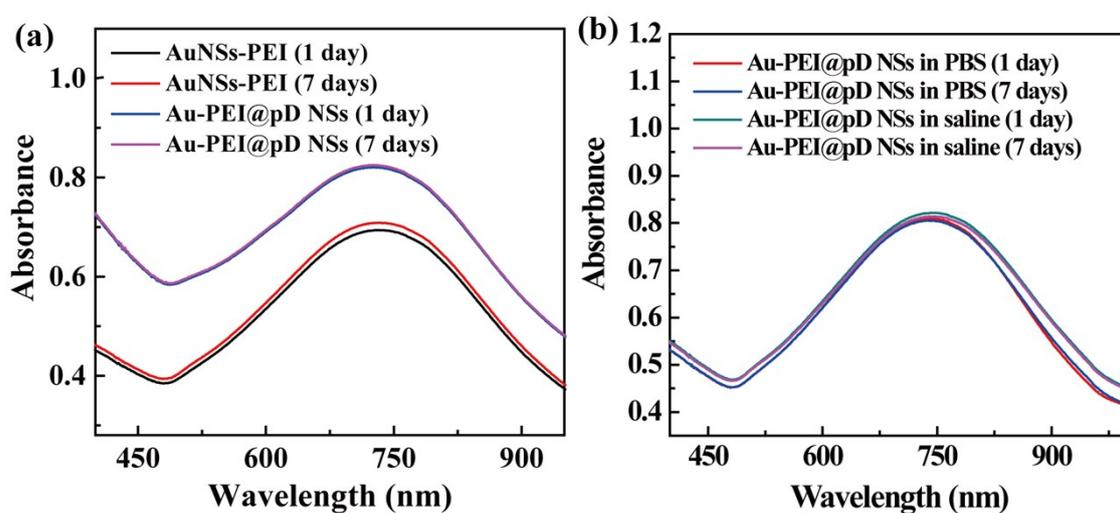
**Figure S5.** (a) UV-vis spectra of AuNSs-PEI and Au-PEI@pD NSs dispersed in water at the same Au concentration (0.35 mM) for different time periods. (b) UV-vis spectra of Au-PEI@pD NSs dispersed in PBS and saline at different time intervals.
