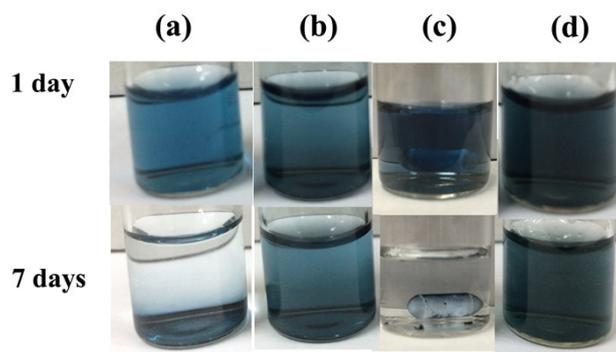
**Figure S4.** Photographs of AuNSs (a), AuNSs-PEI (b), AuNSs@pD (c) and Au-PEI@pD NSs (d) dispersed in water at the Au concentration of 0.35 mM for different time periods.
