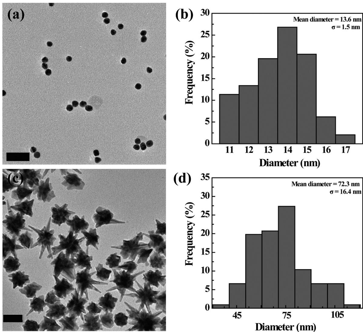
**Figure S1.** TEM images of Au seeds (a) and AuNSs-PEI (c). (b) and (d) show the size distribution histograms of the Au seeds and AuNSs-PEI, respectively. The scale bars in (a) and (c) represent 50 nm.
