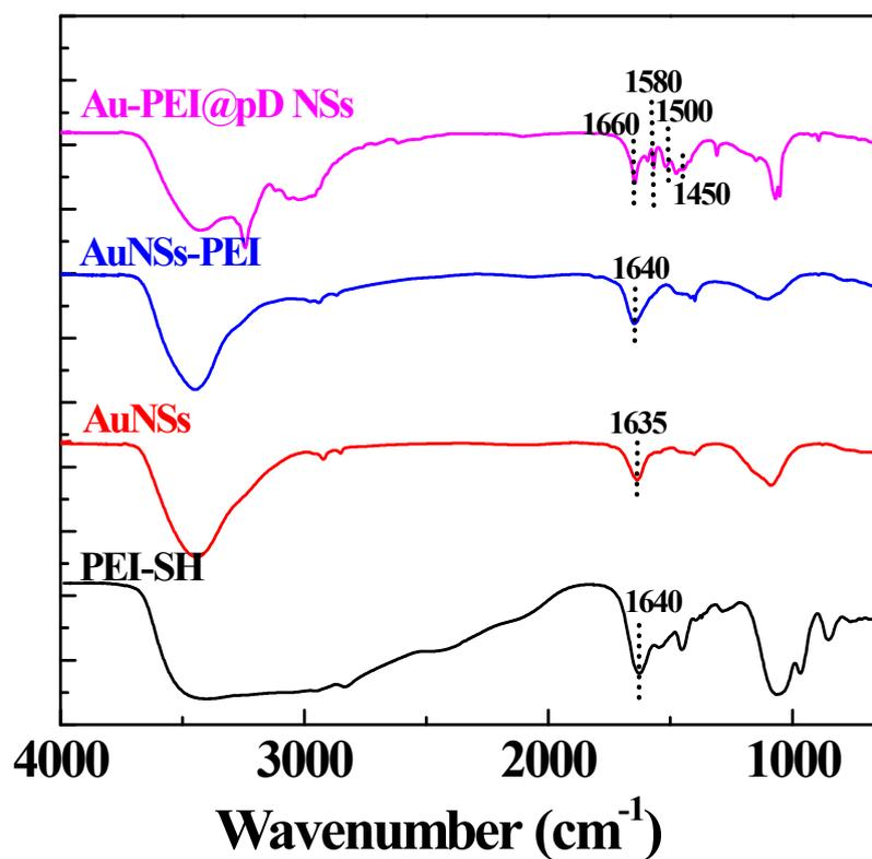
**Figure S2.** FTIR spectra of PEI-SH, AuNSs, AuNSs-PEI, and Au-PEI@pD NSs, respectively.
