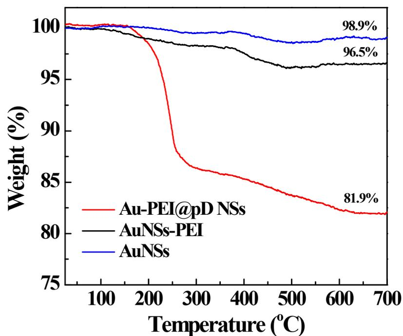
**Figure S3.** TGA curves of non-modified AuNSs, AuNSs-PEI, and Au-PEI@pD NSs, respectively.
