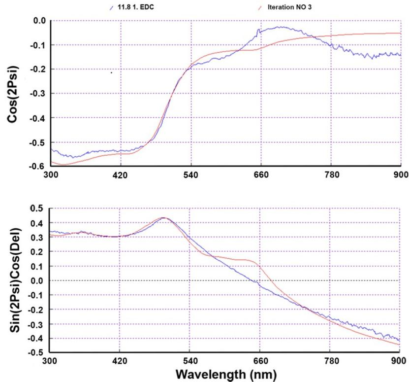
**Fig. S3** Ellipsometer spectrum and fitting curves of HADA modified surfaces.(The goodness of fit is 0.9694).
