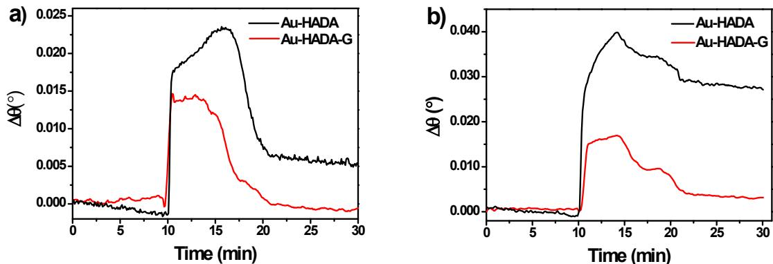
**Fig. S4** SPR sensorgrams showing the non-specific protein adsorption from lysozyme (a) and  $\beta$ -lactoglobulin (b) onto Au-HADA and Au-HADA-G surfaces.
