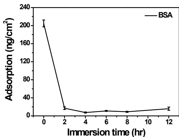
**Fig. S2** The amount of protein adsorbed onto Au-HADA-G chips prepared using different immersion durations for HADA modification.
