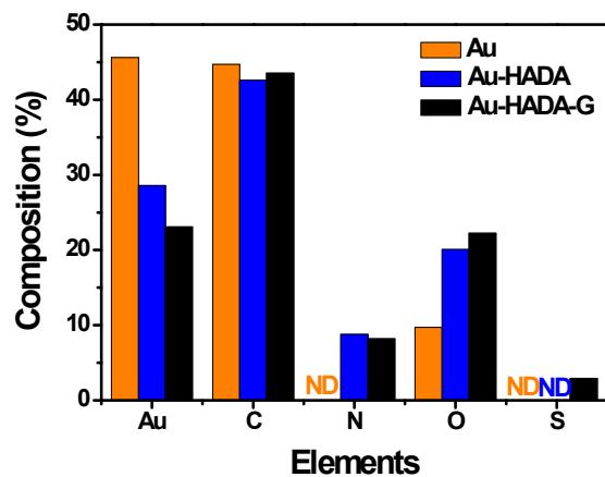
**Fig. S1** XPS surface compositions. Percent elemental surface compositions of Au, C, O, N, and S for bare Au (orange), Au-HADA (blue) and Au-HADA-G (black) surfaces. Note: “ND” represents that no N1S and S2P peak was determined.
