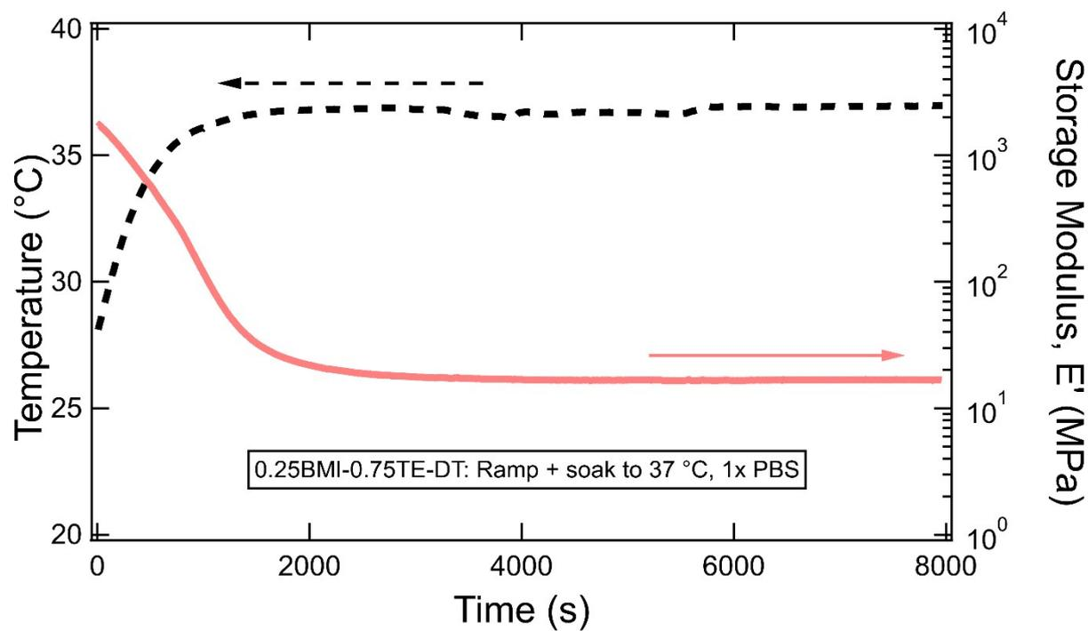
**Figure S5.** Isothermal soaks of 100  $\mu\text{m}$  rectangular bars of 0.25BMI-0.75TE-DT, showing the storage modulus  $E'$  dynamically moving to a steady-state value of  $\sim 17$  MPa after less than 1 hour soak in 1xPBS at 37  $^{\circ}\text{C}$ .
