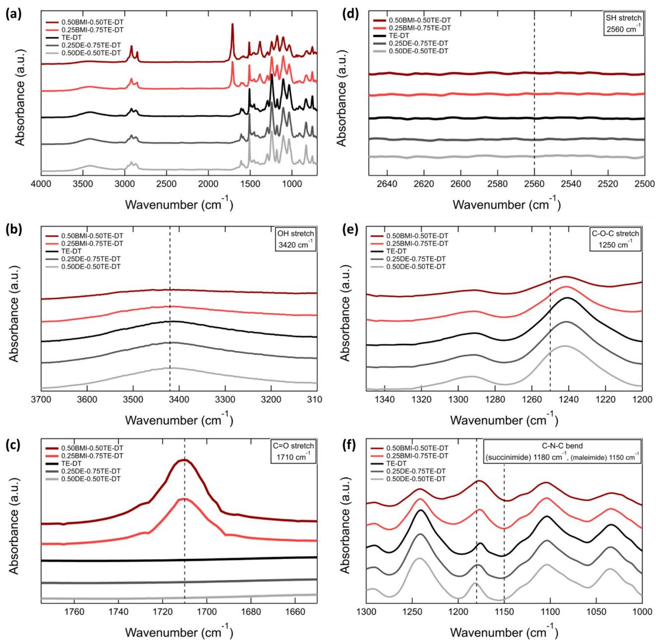
**Figure S1.** Attenuated Total Reflectance Fourier Transform Infrared (ATR-FTIR) spectra of (a) all polymer networks characterized within this work, with zoomed-in regions describing the (b) decrease in  $-OH$  and (c) increase in  $C=O$  functionality in the backbones as a function of the increasing BMI content. (d)  $-SH$ , (e)  $C-O-C$  and (f)  $C-N-C$  spectral zooms, observing the conversion of the thiol, epoxide and maleimide functionalities, respectively.
