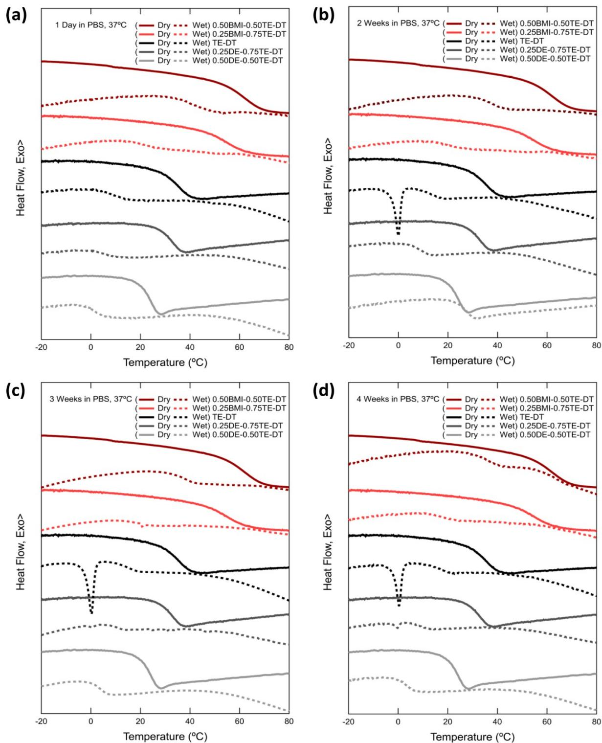
**Figure S3.** DSC thermograms of all five compositions tested showing dry vs. swollen behaviour over (a) 1, (b) 2, (c) 3 and (d) 4 weeks.
