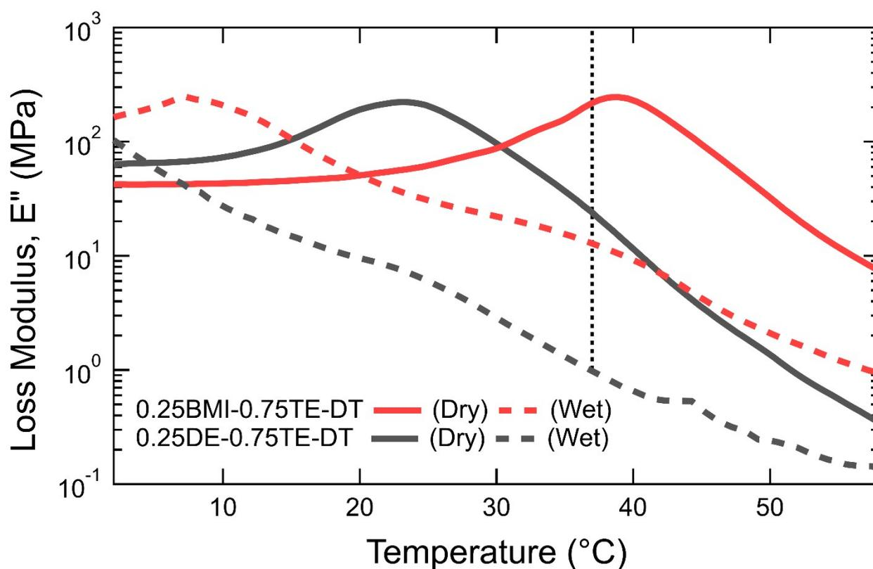
**Figure S4.** Dynamic mechanical analysis (DMA) of 0.25BMI-0.75TE-DT and 0.25DE-0.75TE-DT networks shows the dry and swollen (1 week, 1x PBS at 37  $^{\circ}\text{C}$ ) loss modulus as a function of the temperature. The dashed gray line represents a physiological 37  $^{\circ}\text{C}$ , marking the effective modulus of these materials at that temperature.
